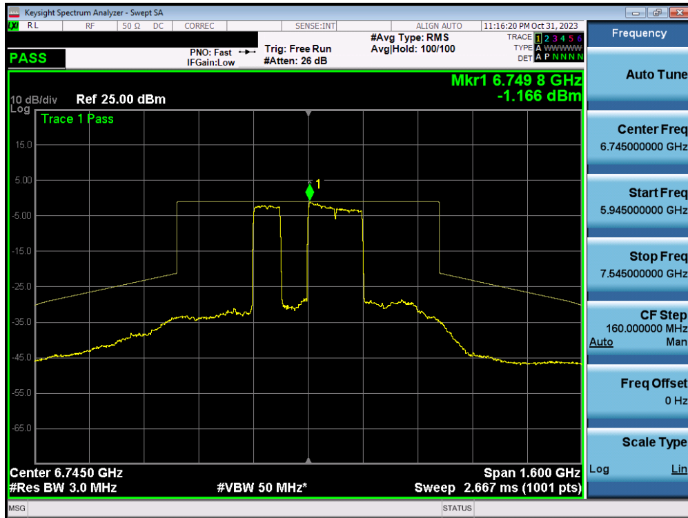
Plot 7-394. In-Band Emission Plot MIMO ANT2 (320MHz BW 802.11ax/be (MRU) (UNII Band 7) – Ch. 159) – SP – 3x996T
