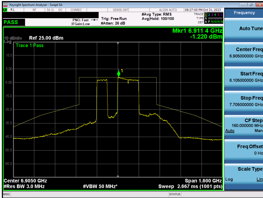
Plot 7-323. In-Band Emission Plot MIMO ANT1 (320MHz BW 802.11ax/be (MRU) (UNII Band 7/8) – Ch. 191) – LPI – 3x996T
