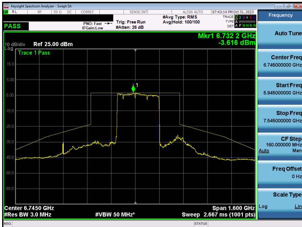
Plot 7-385. In-Band Emission Plot MIMO ANT2 (320MHz BW 802.11ax/be (MRU) (UNII Band 6/7) – Ch. 127) – LPI – 3x996+484T
