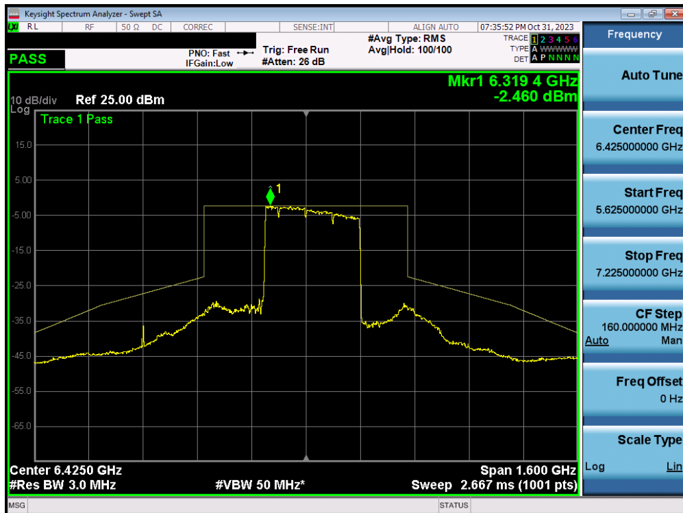
Plot 7-373. In-Band Emission Plot MIMO ANT2 (320MHz BW 802.11ax/be (MRU) (UNII Band 5/6/7) – Ch. 95) – LPI – 3x996+484T
