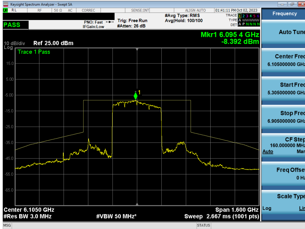
Plot 7-412. In-Band Emission Plot MIMO ANT2 (320MHz BW 802.11ax/be (26 Tones) (UNII Band 5) – Ch. 31) – LPI
