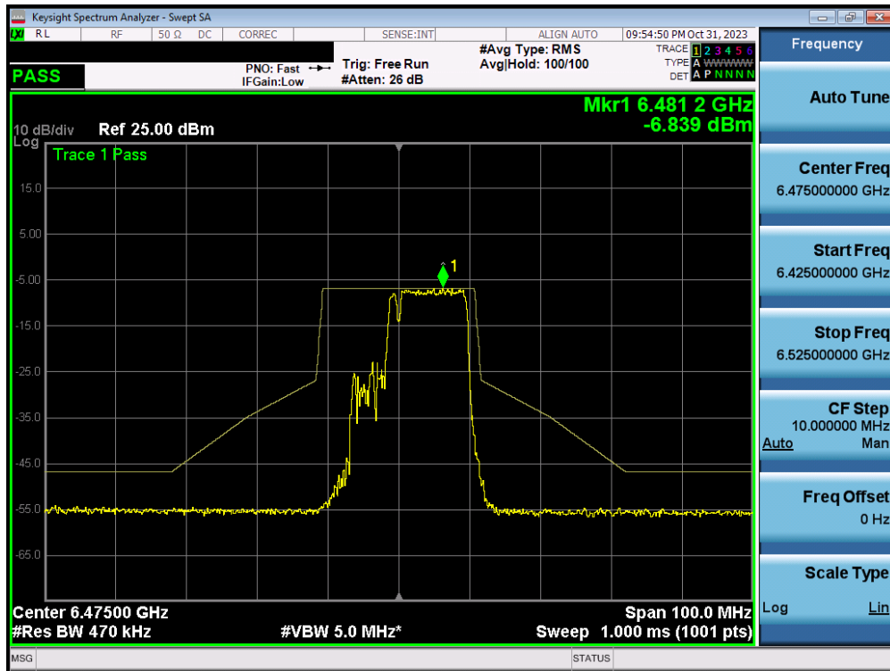
Plot 7-363. In-Band Emission Plot MIMO ANT2 (20MHz BW 802.11ax/be (MRU) (UNII Band 6) – Ch. 105) – LPI – 106+26T
