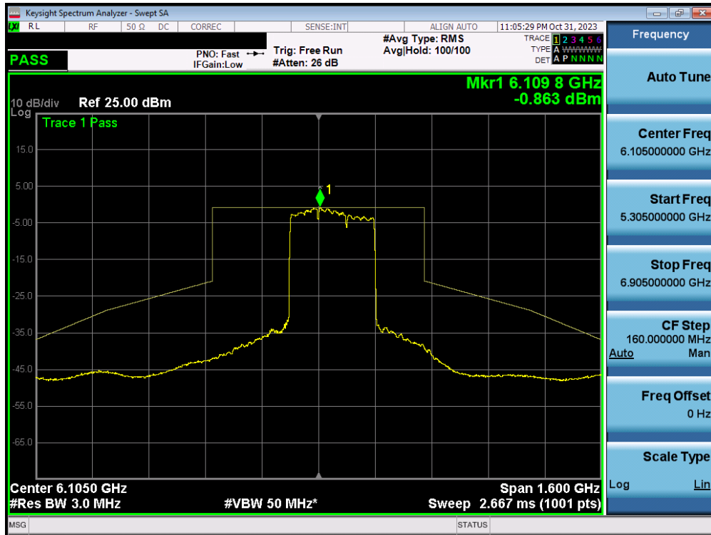
Plot 7-277. In-Band Emission Plot MIMO ANT1 (320MHz BW 802.11ax/be (MRU) (UNII Band 5) – Ch. 31) – SP – 3x996T
