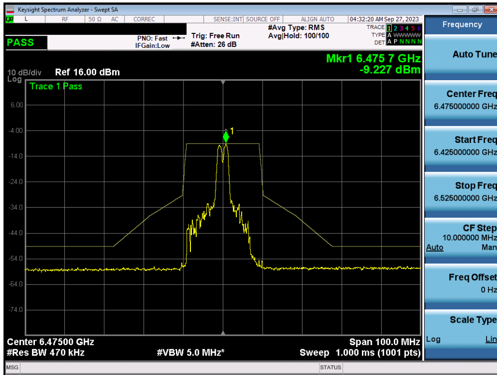
Plot 7-279. In-Band Emission Plot MIMO ANT1 (20MHz BW 802.11ax/be (26 Tones) (UNII Band 6) – Ch. 105) – LPI
