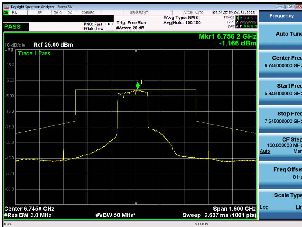
Plot 7-300. In-Band Emission Plot MIMO ANT1 (320MHz BW 802.11ax/be (MRU) (UNII Band 6/7) – Ch. 159) – LPI – 2x996+484T
