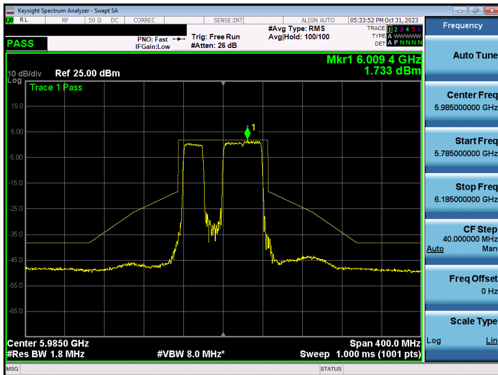
Plot 7-262. In-Band Emission Plot MIMO ANT1 (80MHz BW 802.11ax/be (MRU) (UNII Band 5) – Ch. 39) – LPI – 484+242T
