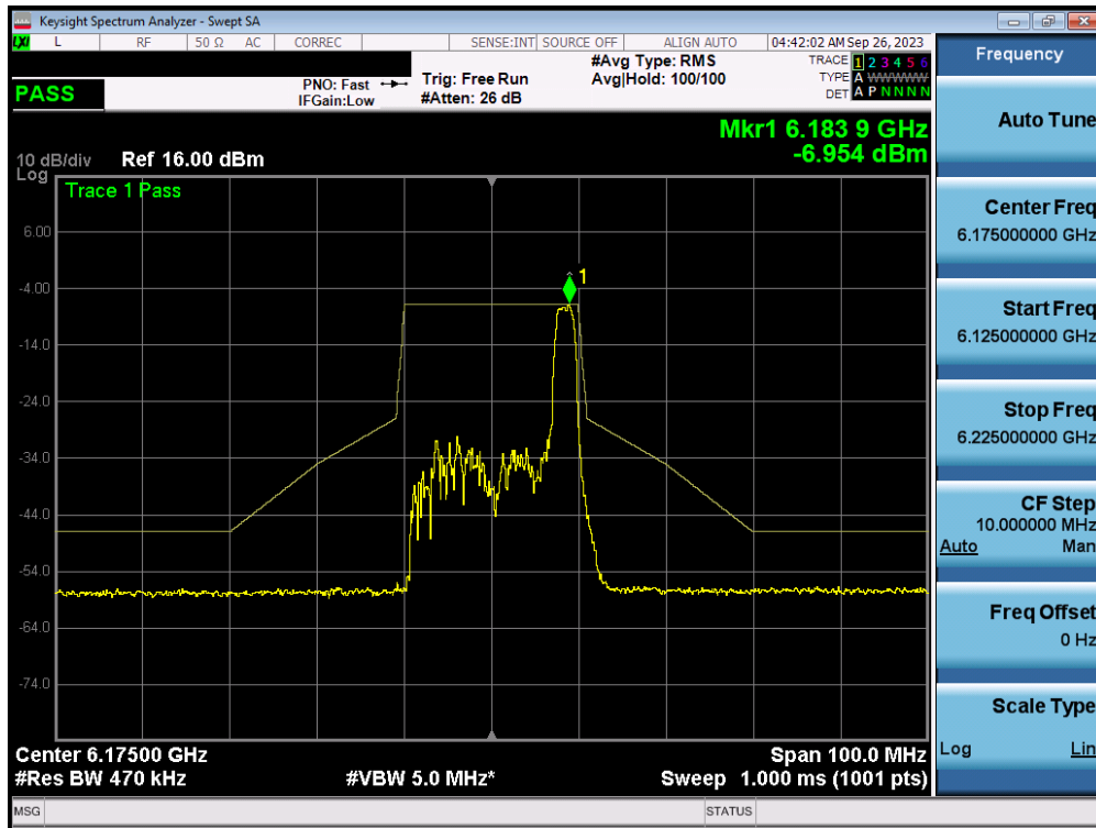
Plot 7-257. In-Band Emission Plot MIMO ANT1 (20MHz BW 802.11ax/be (26 Tones) (UNII Band 5) – Ch. 45) – LPI
