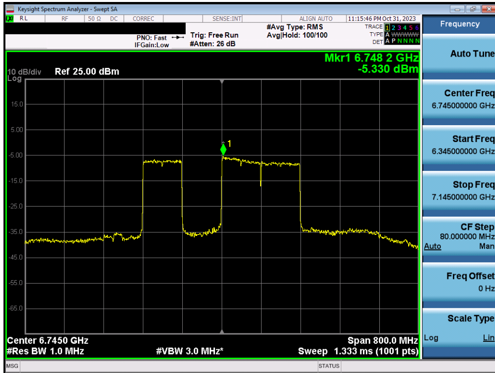
Plot 7-223. Power Spectral Density Plot MIMO ANT2 (320MHz BW 802.11ax/be (MRU) (UNII Band 7) – Ch. 159) – SP – 3x996T
