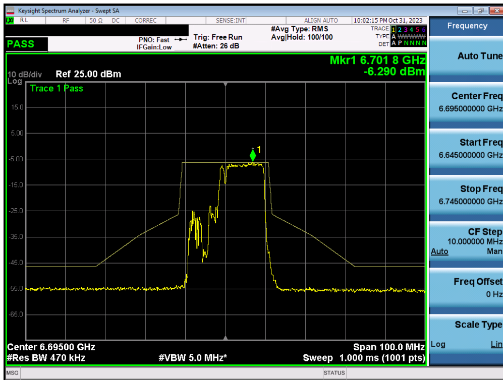
Plot 7-292. In-Band Emission Plot MIMO ANT1 (20MHz BW 802.11ax/be (MRU) (UNII Band 7) – Ch. 149) – LPI – 106+26T
