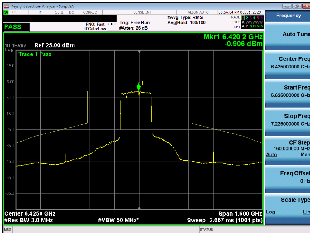
Plot 7-288. In-Band Emission Plot MIMO ANT1 (320MHz BW 802.11ax/be (MRU) (UNII Band 5/6/7) – Ch. 95) – LPI – 2x996+484T
