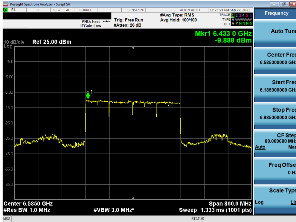
Plot 7-251. Power Spectral Density Plot MIMO ANT2 (320MHz BW 802.11ax/be (26 Tones) (UNII Band 6/7) – Ch. 127) – LPI
