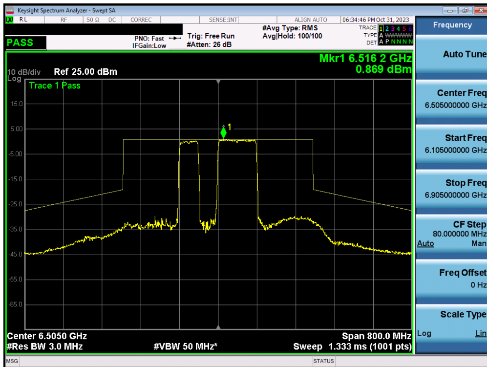
Plot 7-286. In-Band Emission Plot MIMO ANT1 (160MHz BW 802.11ax/be (MRU) (UNII Band 6) – Ch. 111) – LPI – 996+484T
