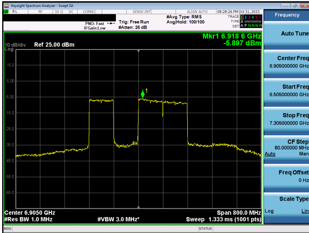
Plot 7-235. Power Spectral Density Plot MIMO ANT2 (320MHz BW 802.11ax/be (MRU) (UNII Band 7/8) – Ch. 191) – LPI – 3x996T
