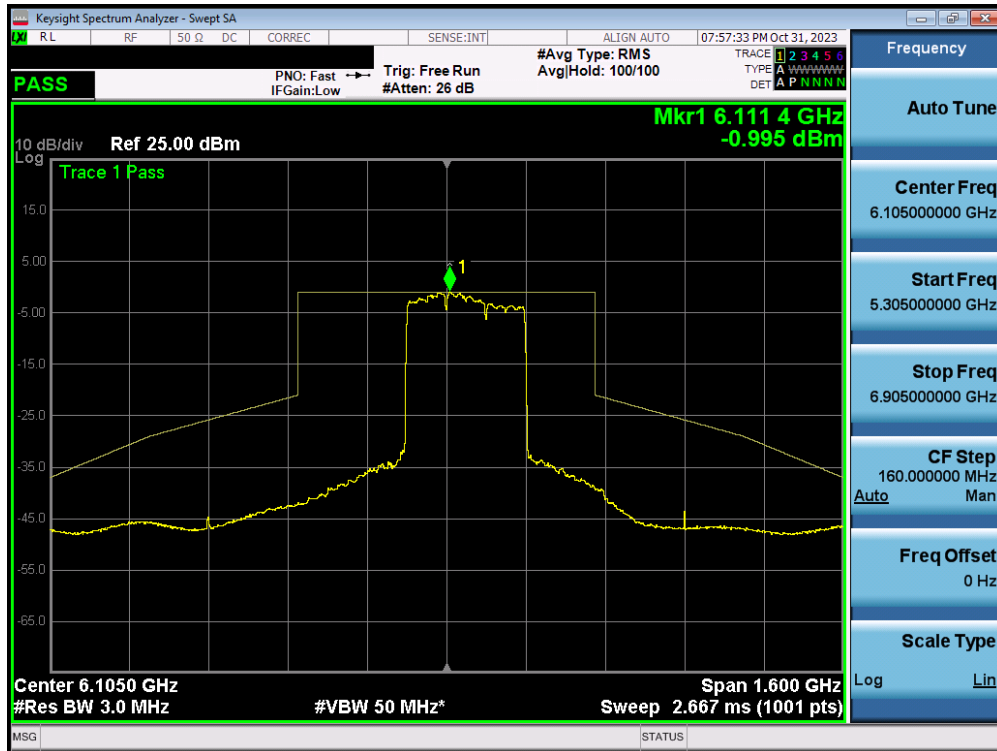
Plot 7-267. In-Band Emission Plot MIMO ANT1 (320MHz BW 802.11ax/be (MRU) (UNII Band 5) – Ch. 31) – LPI – 3x996T
