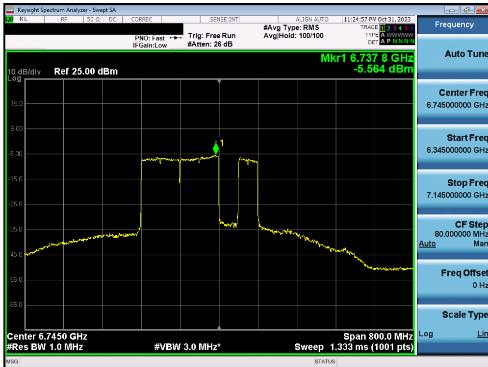
Plot 7-222. Power Spectral Density Plot MIMO ANT2 (320MHz BW 802.11ax/be (MRU) (UNII Band 7) – Ch. 159) – SP – 2x996+484T
