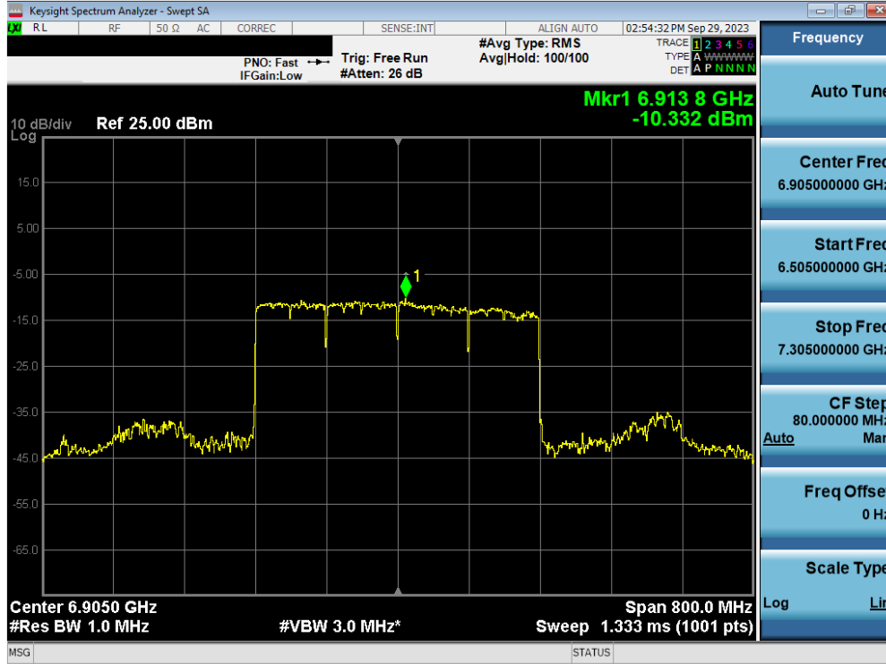
Plot 7-256. Power Spectral Density Plot MIMO ANT2 (320MHz BW 802.11ax/be (26 Tones) (UNII Band 8) – Ch. 191) – LPI
