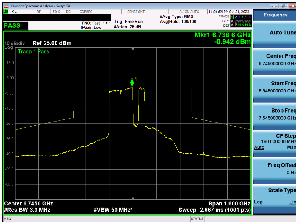
Plot 7-310. In-Band Emission Plot MIMO ANT1 (320MHz BW 802.11ax/be (MRU) (UNII Band 7) – Ch. 159) – SP – 2x996+484T
