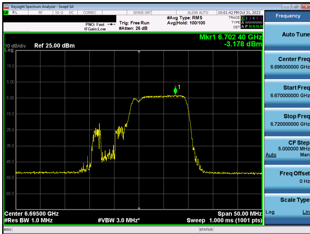
Plot 7-116. Power Spectral Density Plot MIMO ANT1 (20MHz BW 802.11ax/be (MRU) (UNII Band 7) – Ch. 149) – LPI – 106+26T
