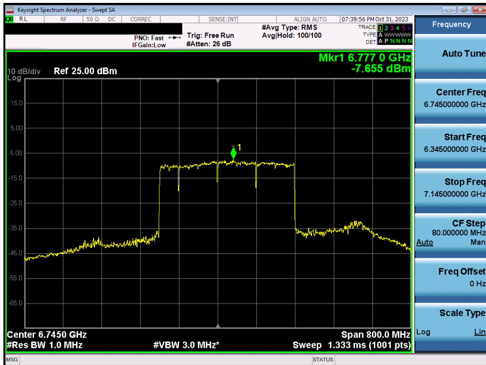
Plot 7-126. Power Spectral Density Plot MIMO ANT1 (320MHz BW 802.11ax/be (MRU) (UNII Band 6/7) – Ch. 127) – LPI – 3x996+484T
