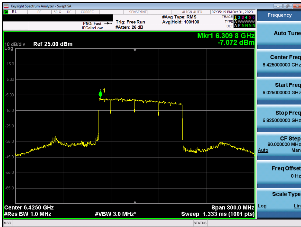
Plot 7-202. Power Spectral Density Plot MIMO ANT2 (320MHz BW 802.11ax/be (MRU) (UNII Band 5/6/7) – Ch. 95) – LPI – 3x996T+484
