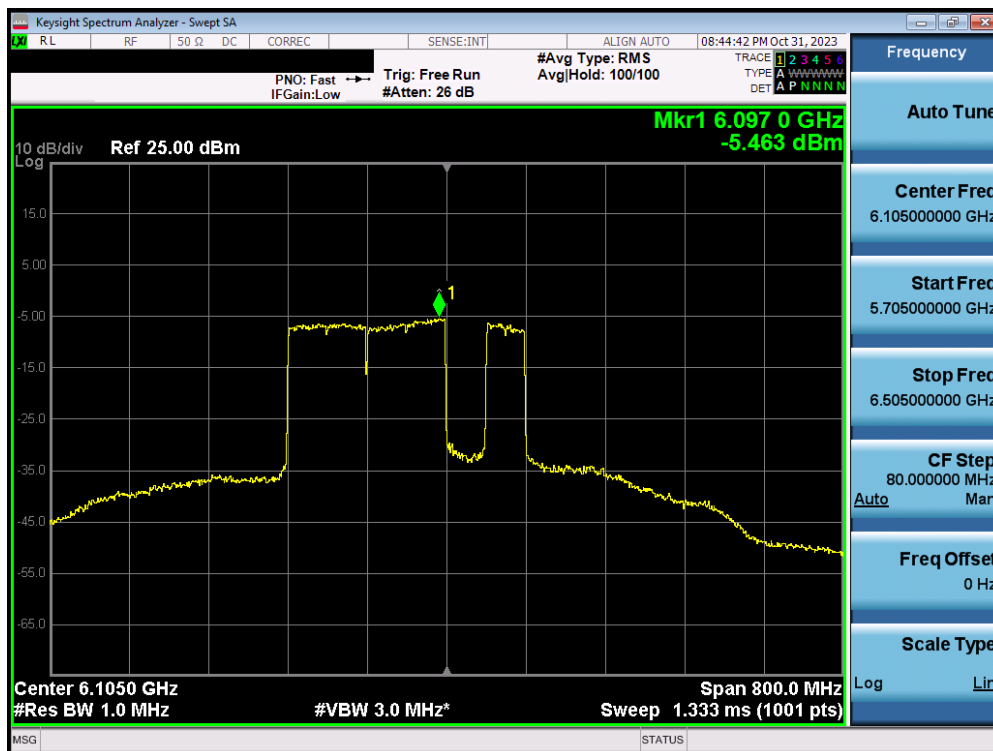
Plot 7-178. Power Spectral Density Plot MIMO ANT2 (320MHz BW 802.11ax/be (MRU) (UNII Band 5) – Ch. 31) – LPI – 2x996+484T
