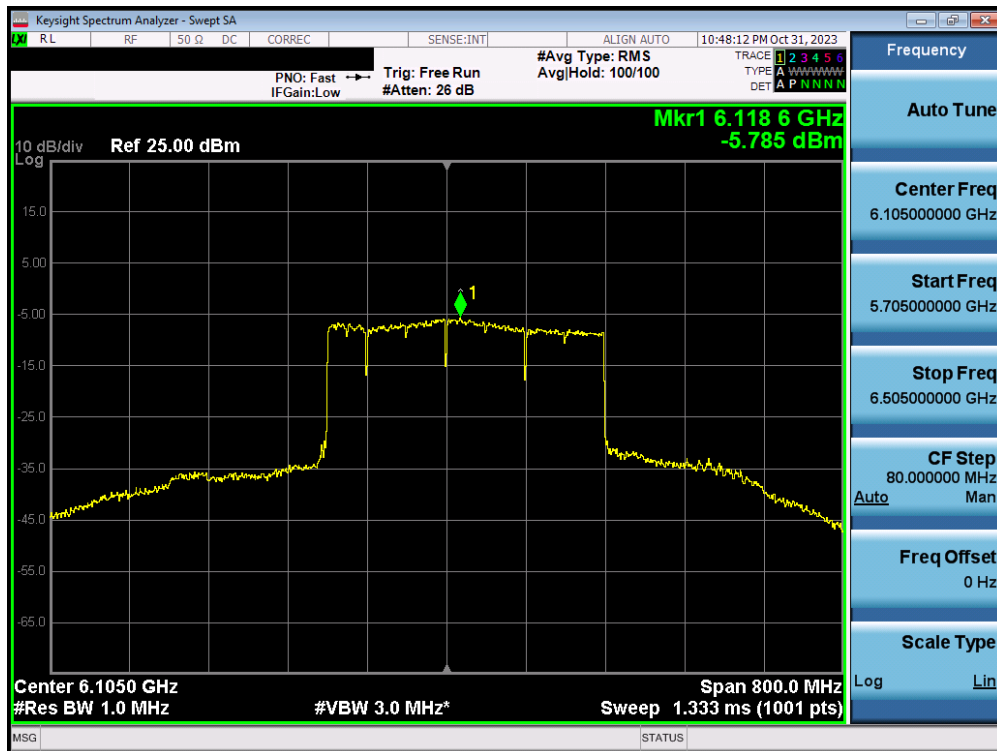
Plot 7-190. Power Spectral Density Plot MIMO ANT2 (320MHz BW 802.11ax/be (MRU) (UNII Band 5) – Ch. 31) – SP – 3x996+484T
