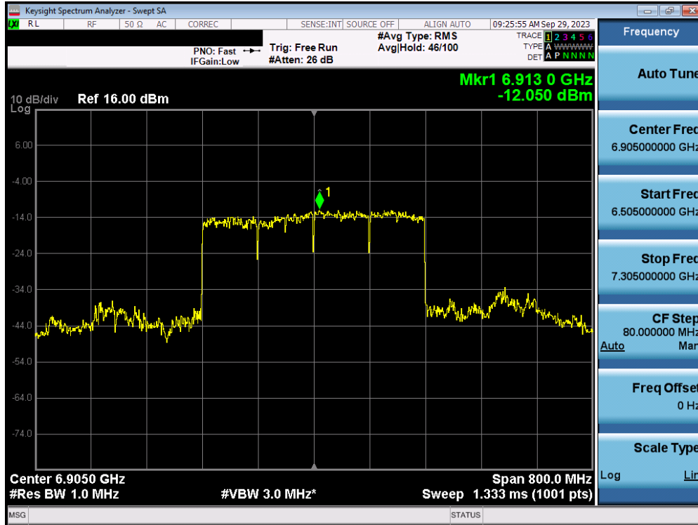
Plot 7-168. Power Spectral Density Plot MIMO ANT1 (320MHz BW 802.11ax/be (26 Tones) (UNII Band 8) – Ch. 191) – LPI
