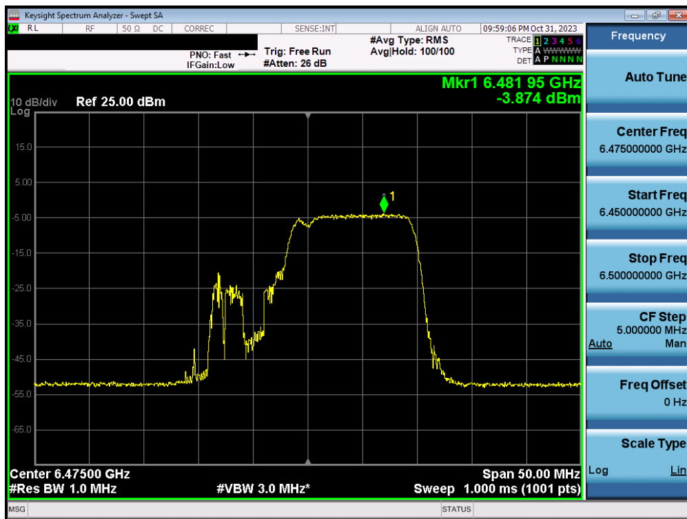
Plot 7-104. Power Spectral Density Plot MIMO ANT1 (20MHz BW 802.11ax/be (MRU) (UNII Band 6) – Ch. 105) – LPI – 106+26T
