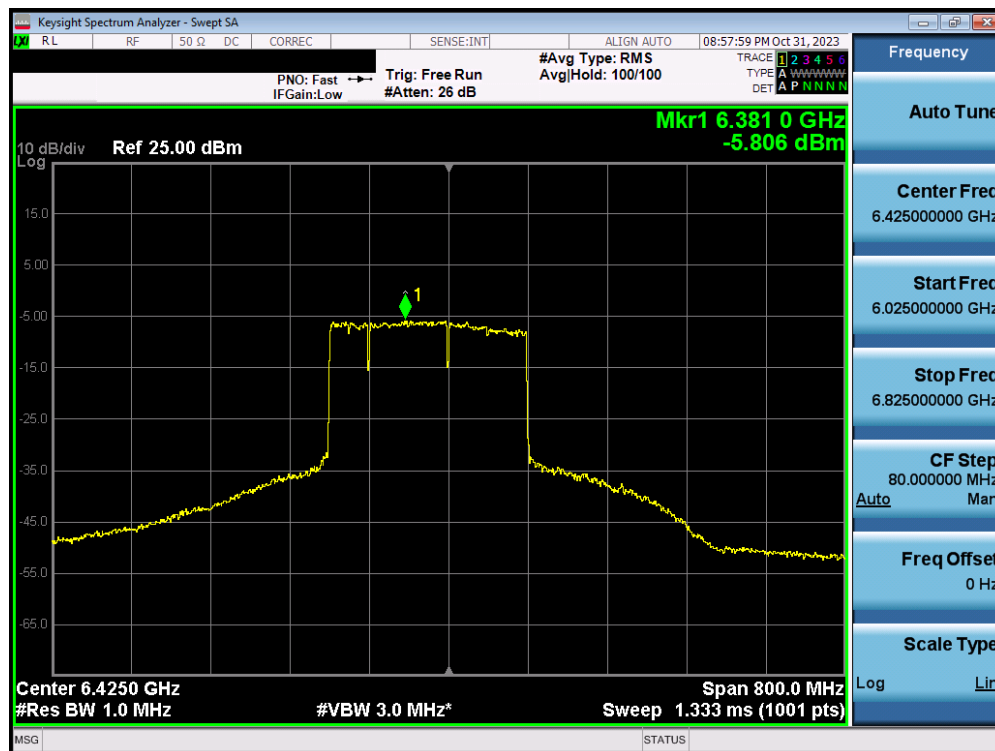
Plot 7-200. Power Spectral Density Plot MIMO ANT2 (320MHz BW 802.11ax/be (MRU) (UNII Band 5/6/7) – Ch. 95) – LPI – 2x996+484T
