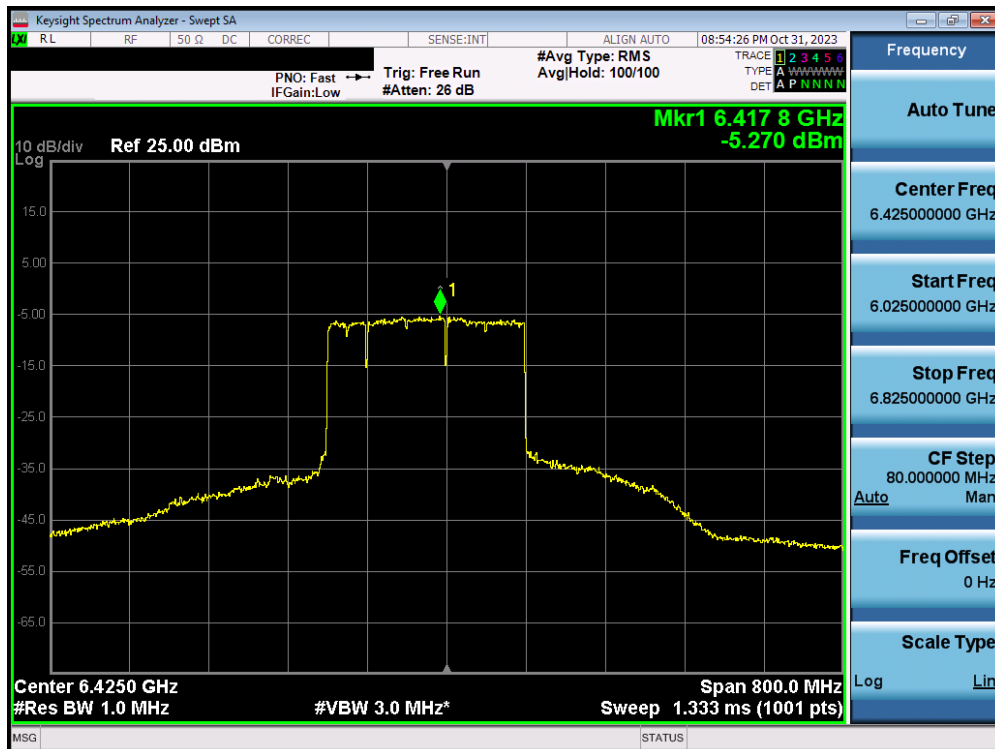
Plot 7-112. Power Spectral Density Plot MIMO ANT1 (320MHz BW 802.11ax/be (MRU) (UNII Band 5/6/7) – Ch. 95) – LPI – 2x996+484T
