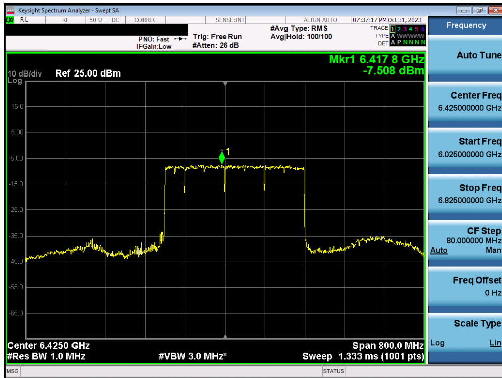
Plot 7-114. Power Spectral Density Plot MIMO ANT1 (320MHz BW 802.11ax/be (MRU) (UNII Band 5/6/7) – Ch. 95) – LPI – 3x996+484T
