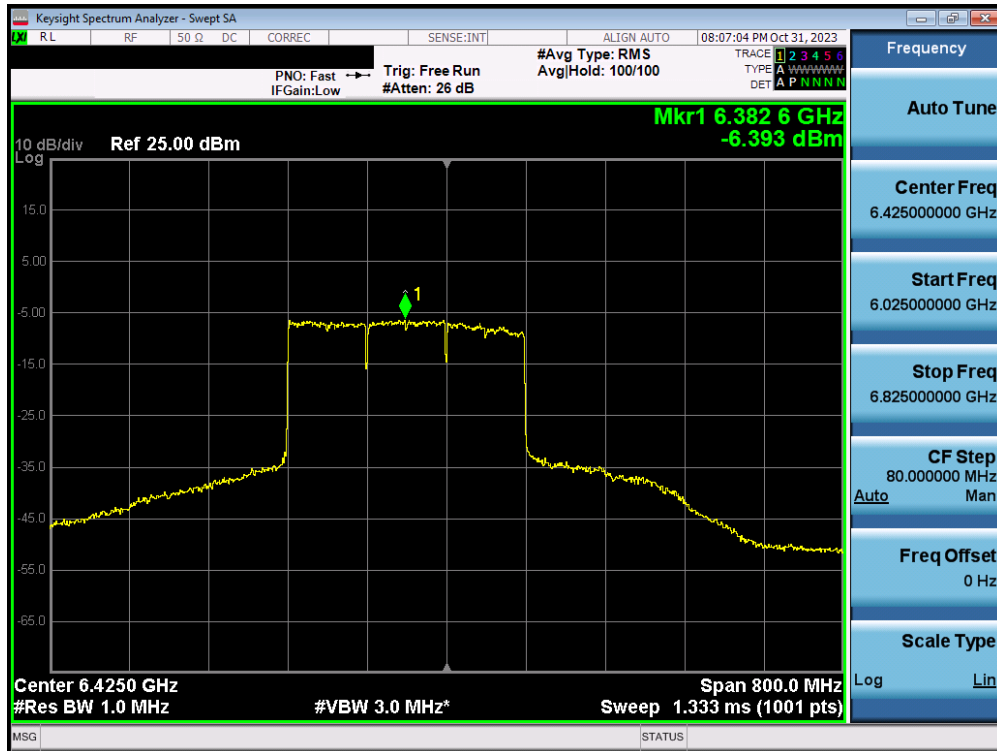
Plot 7-201. Power Spectral Density Plot MIMO ANT2 (320MHz BW 802.11ax/be (MRU) (UNII Band 5/6/7) – Ch. 95) – LPI – 3x996T
