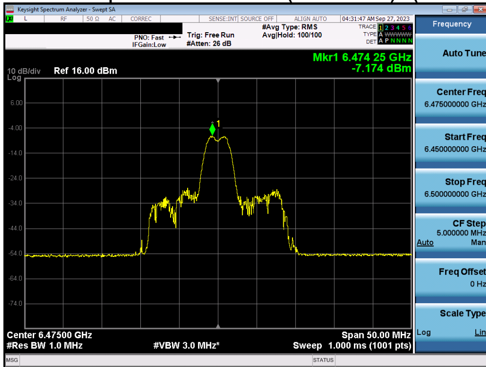
Plot 7-103. Power Spectral Density Plot MIMO ANT1 (20MHz BW 802.11ax/be (26 Tones) (UNII Band 6) – Ch. 105) – LPI
