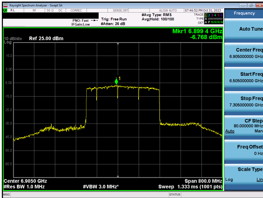
Plot 7-148. Power Spectral Density Plot MIMO ANT1 (320MHz BW 802.11ax/be (MRU) (UNII Band 7/8) – Ch. 191) – LPI – 3x996+484T
