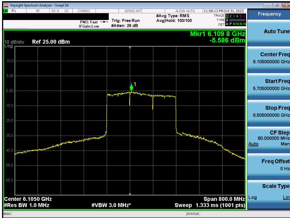
Plot 7-189. Power Spectral Density Plot MIMO ANT2 (320MHz BW 802.11ax/be (MRU) (UNII Band 5) – Ch. 31) – SP – 3x996T
