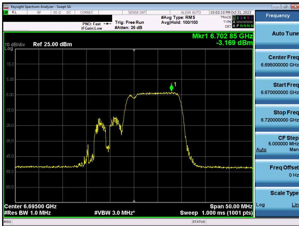
Plot 7-204. Power Spectral Density Plot MIMO ANT2 (20MHz BW 802.11ax/be (MRU) (UNII Band 7) – Ch. 149) – LPI – 106+26T
