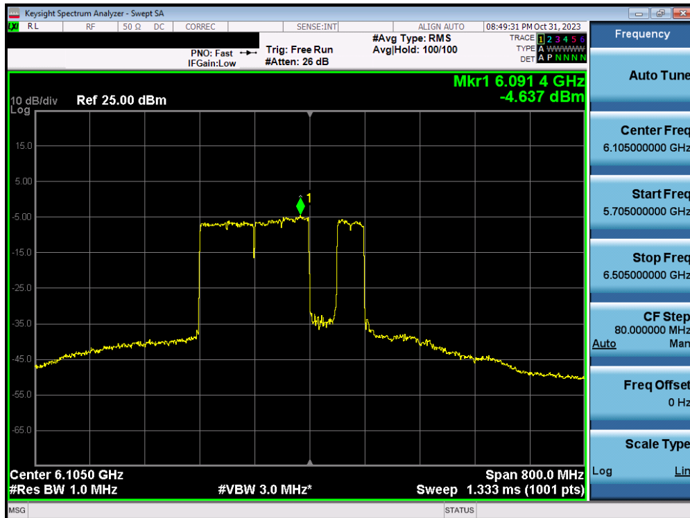
Plot 7-90. Power Spectral Density Plot MIMO ANT1 (320MHz BW 802.11ax/be (MRU) (UNII Band 5) – Ch. 31) – LPI – 2x996+484T
