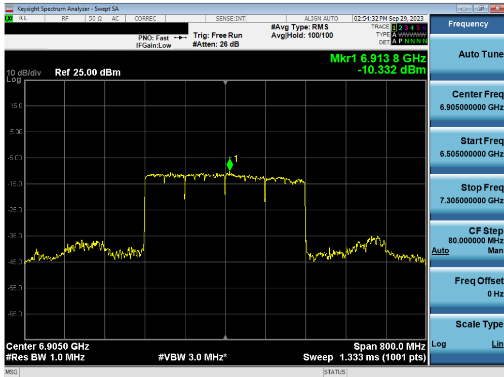
Plot 7-119. Power Spectral Density MIMO ANT2 (320MHz 802.11ax/be (UNII Band 7/8) – Ch. 191) - LPI
