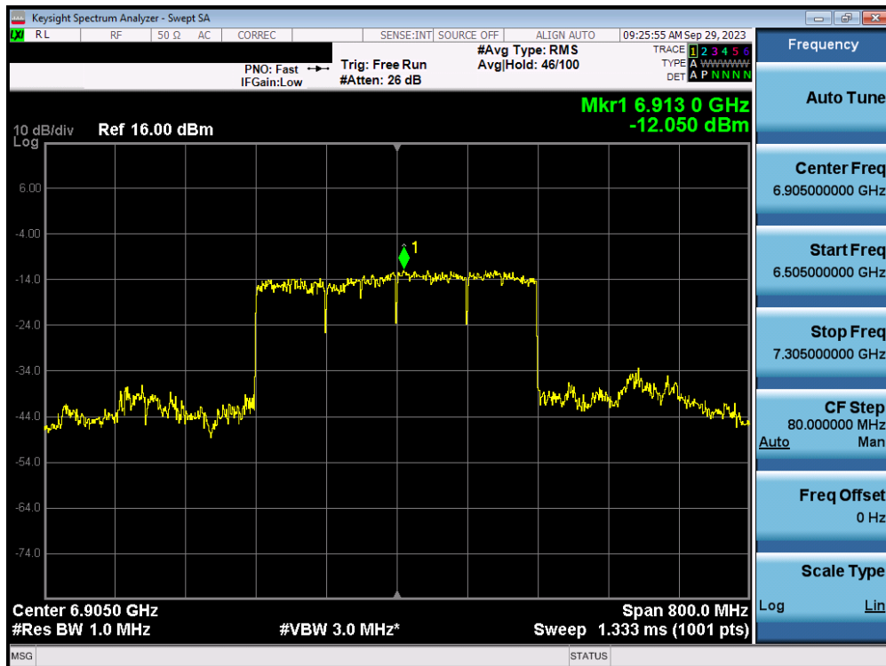
Plot 7-84. Power Spectral Density MIMO ANT1 (320MHz 802.11ax/be (UNII Band 7/8) – Ch. 191) - LPI
