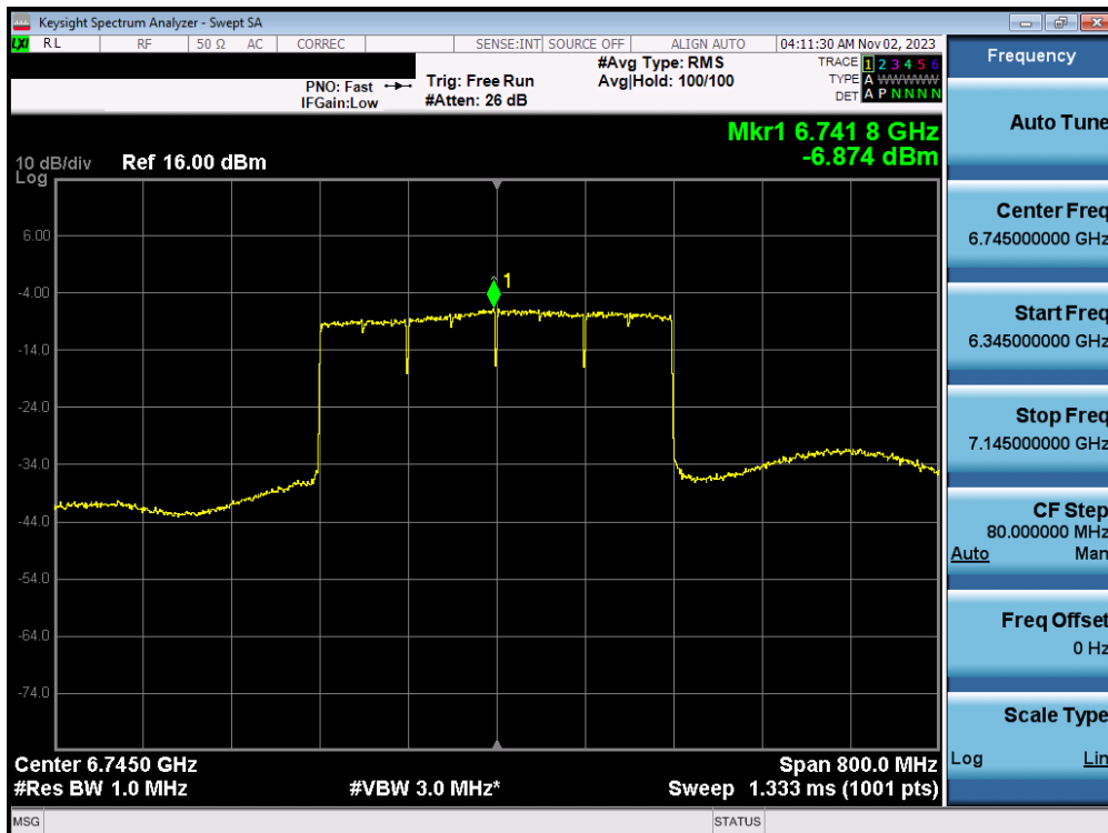
Plot 7-78. Power Spectral Density MIMO ANT1 (320MHz 802.11ax/be (UNII Band 6/7) – Ch. 159) - SP
