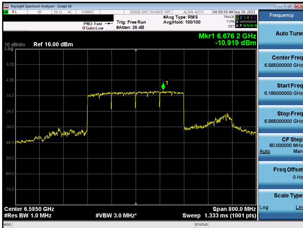
Plot 7-72. Power Spectral Density MIMO ANT1 (320MHz 802.11ax/be (UNII Band 6/7) – Ch. 127) - LPI
