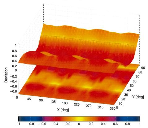
Probe isotropy for E<sub>tot</sub>: probe rotated  $\phi=0^\circ$  to 360°, tilted from field propagation direction  $\vec{k}$  Parallel to the field propagation ( $\psi=0^\circ-90^\circ$ ) at 30 GHz: deviation within  $\pm 0.37$  dB Parallel to the field propagation ( $\psi=0^\circ-90^\circ$ ) at 60 GHz: deviation within  $\pm 0.44$  dB
