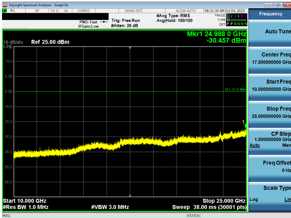
Plot 7-158. Conducted Spurious Plot (Bluetooth, 1Mbps – Ch. 78) – Dual ANT1
