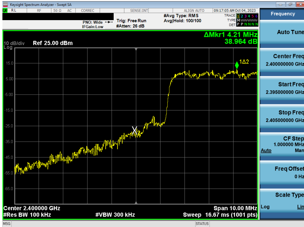
Plot 7-123. Band Edge Plot (Bluetooth with Hopping Enabled, 3 Mbps – Ch. 0) – Dual ANT2
