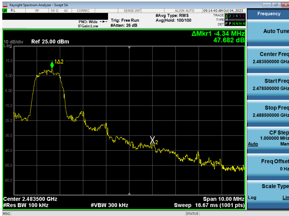
Plot 7-122. Band Edge Plot (Bluetooth with Hopping Disabled, 3 Mbps – Ch. 78) – Dual ANT2
