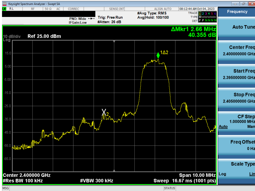
Plot 7-117. Band Edge Plot (Bluetooth with Hopping Disabled, 3 Mbps – Ch. 0) – Dual ANT1
