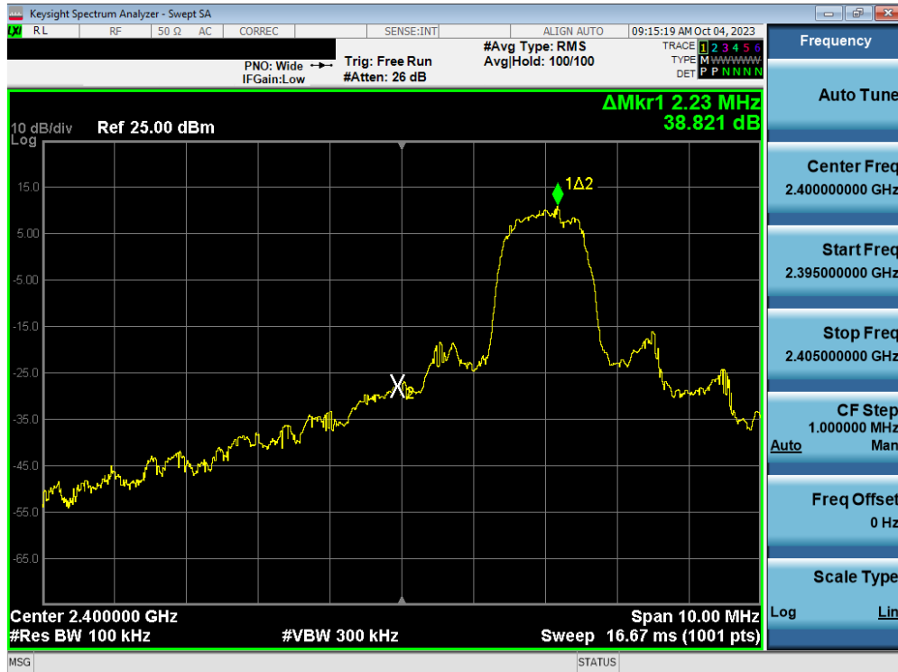
Plot 7-121. Band Edge Plot (Bluetooth with Hopping Disabled, 3 Mbps – Ch. 0) – Dual ANT2
