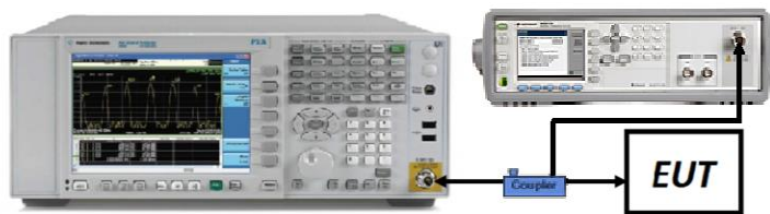
Figure 7-5. Test Instrument & Measurement Setup
