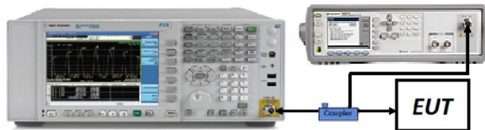
Figure 7-7. Test Instrument & Measurement Setup
