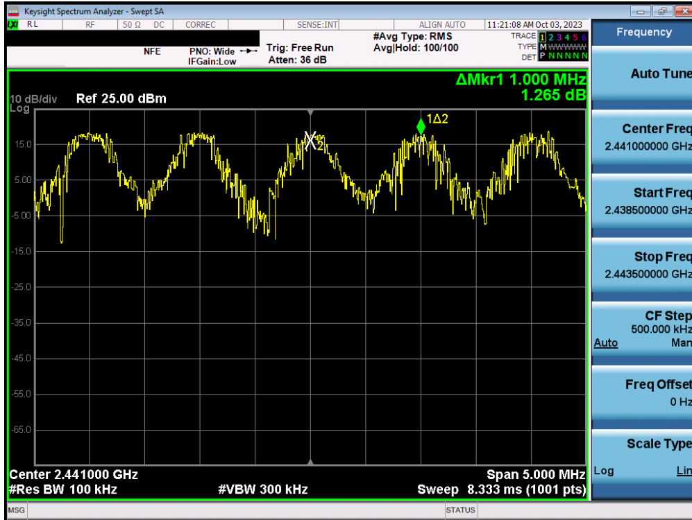
Plot 7-125. Channel Spacing Plot (Bluetooth) – ANT1
