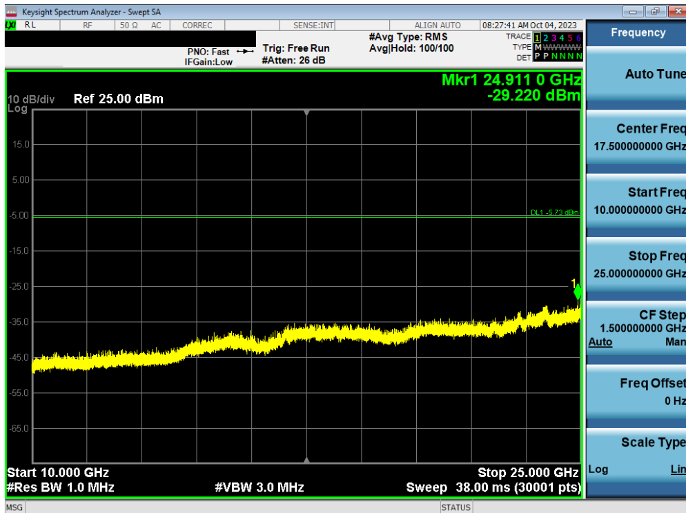
Plot 7-156. Conducted Spurious Plot (Bluetooth, 1Mbps – Ch. 39) – Dual ANT1
