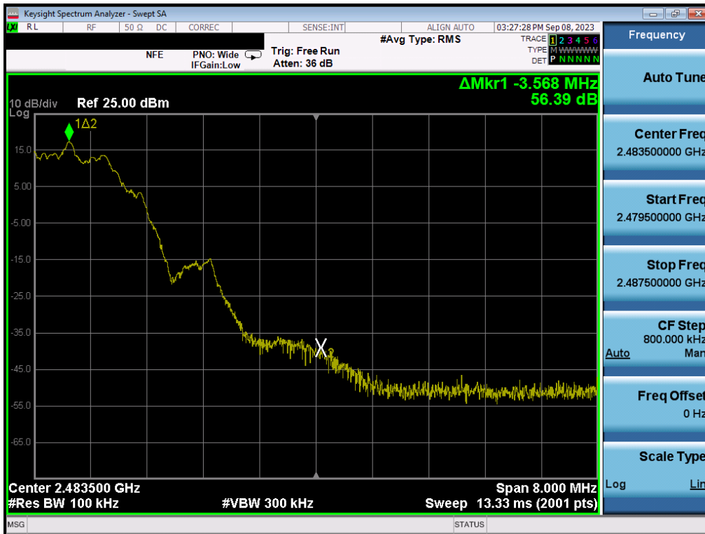
Plot 7-116. Band Edge Plot (Bluetooth (LE), 2Mbps – Ch. 39) – ANT1
