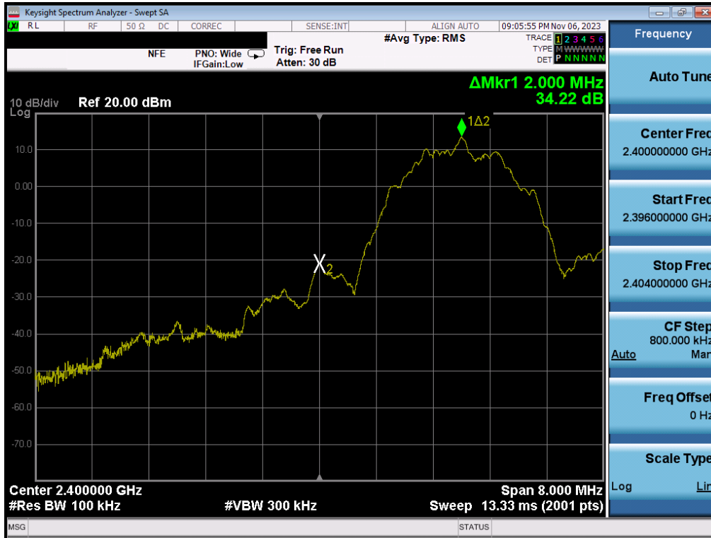
Plot 7-127. Band Edge Plot (Bluetooth (LE), 2Mbps – Ch. 0) – Dual ANT1
