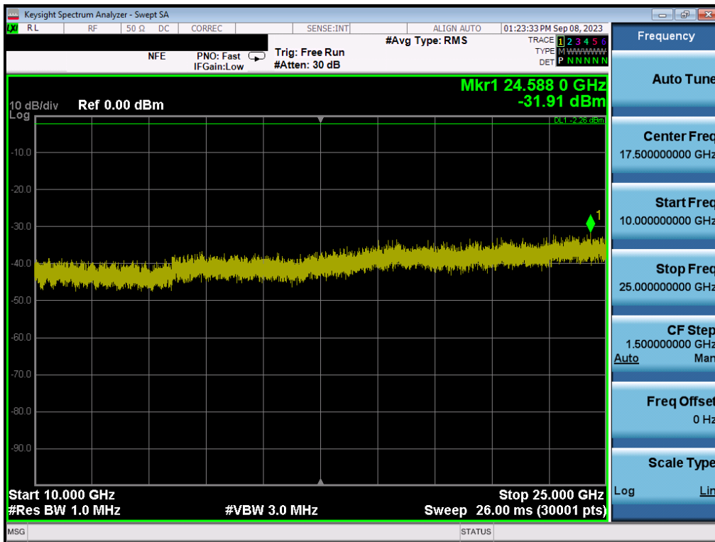
Plot 7-142. Conducted Spurious Plot (Bluetooth (LE), 1Mbps – Ch. 19) – ANT2
