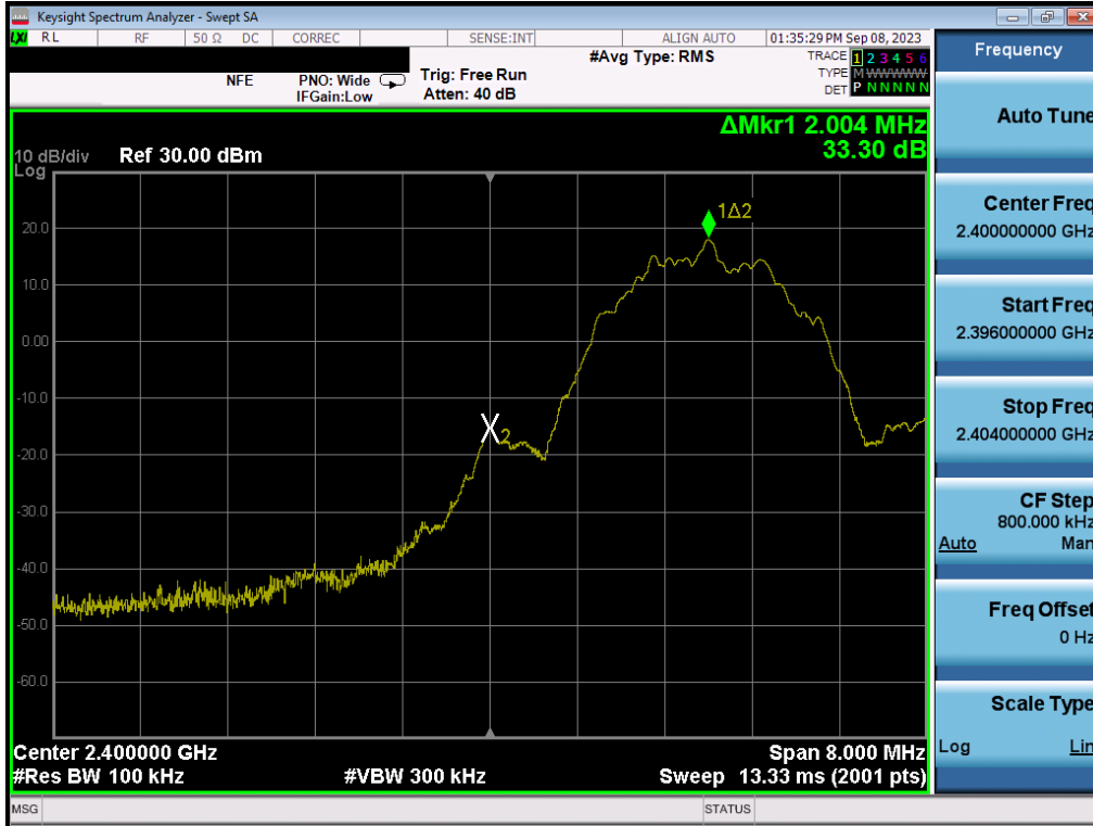
Plot 7-123. Band Edge Plot (Bluetooth (LE), 2Mbps – Ch. 0) – ANT2
