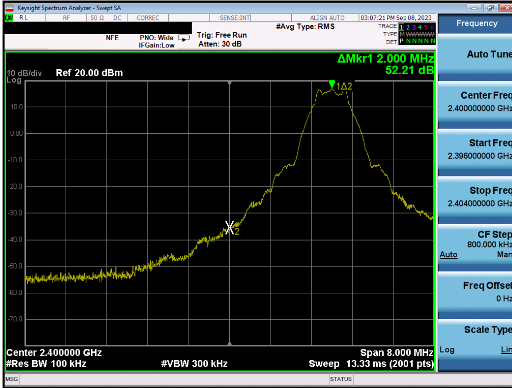
Plot 7-113. Band Edge Plot (Bluetooth (LE), 1Mbps – Ch. 0) – ANT1
