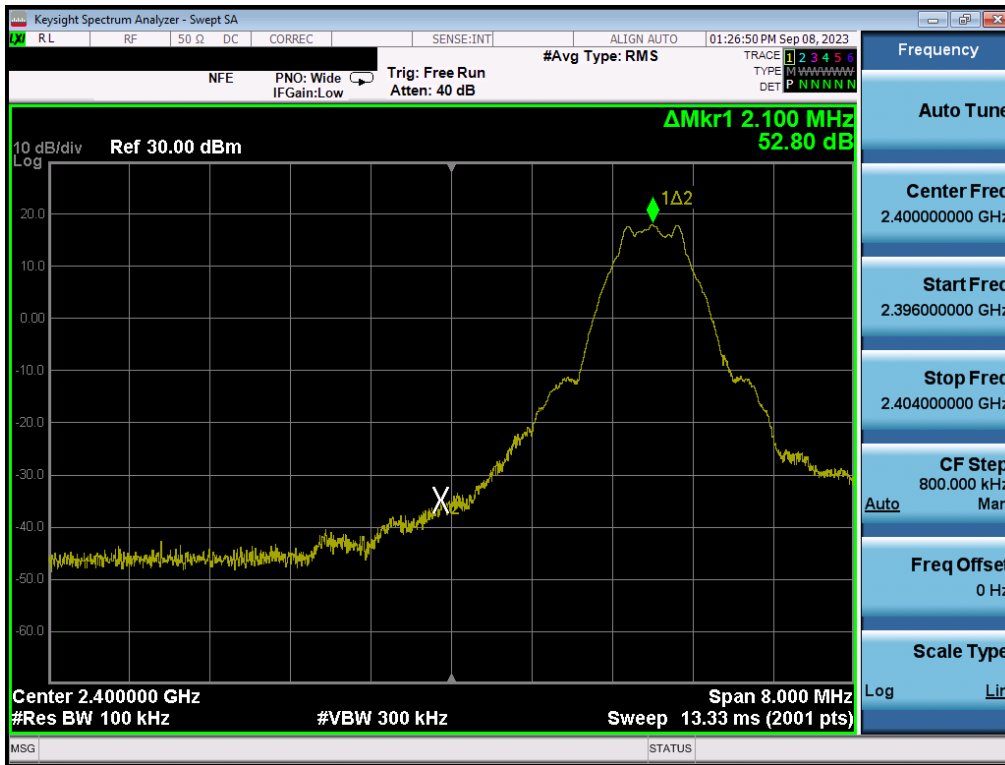
Plot 7-121. Band Edge Plot (Bluetooth (LE), 1Mbps – Ch. 0) – ANT2
