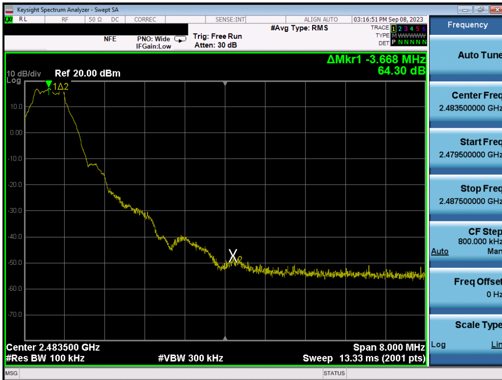
Plot 7-114. Band Edge Plot (Bluetooth (LE), 1Mbps – Ch. 39) – ANT1
