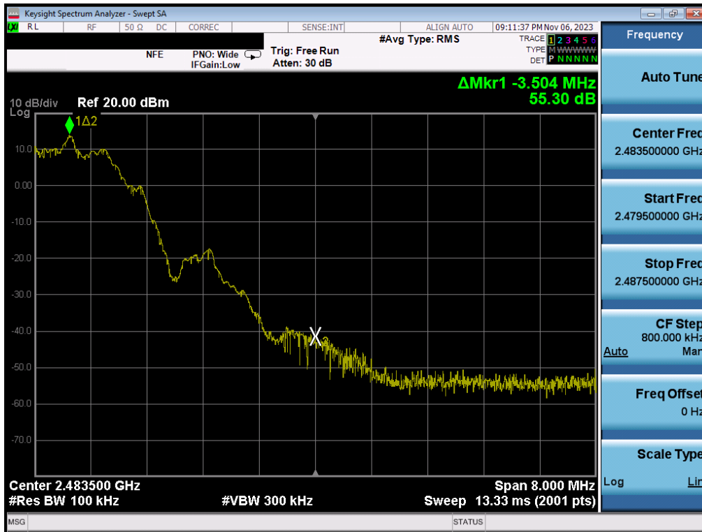
Plot 7-128. Band Edge Plot (Bluetooth (LE), 2Mbps – Ch. 39) – Dual ANT1
