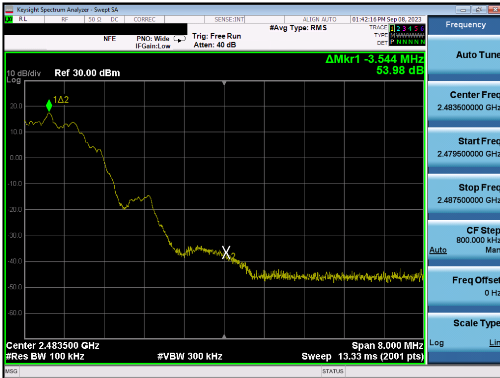
Plot 7-124. Band Edge Plot (Bluetooth (LE), 2Mbps – Ch. 39) – ANT2
