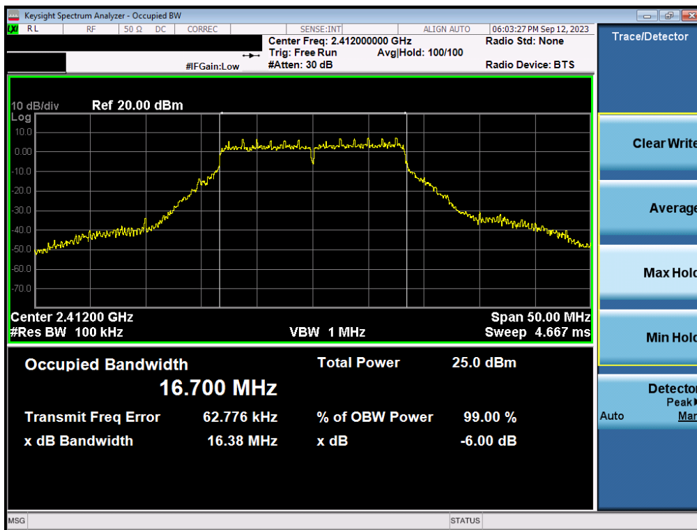
Plot 7-4. 6dB Bandwidth Plot SISO ANT1 (802.11g – Ch. 1)
