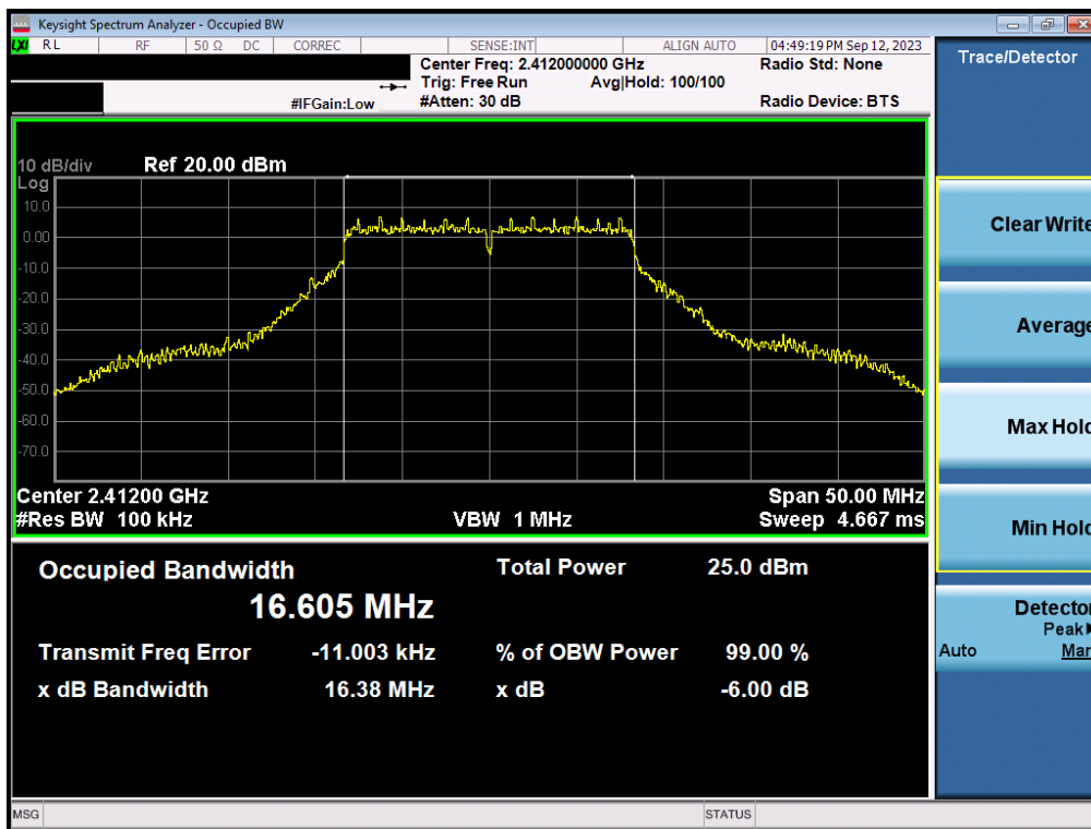
Plot 7-16. 6dB Bandwidth Plot SISO ANT2 (802.11g – Ch. 1)
