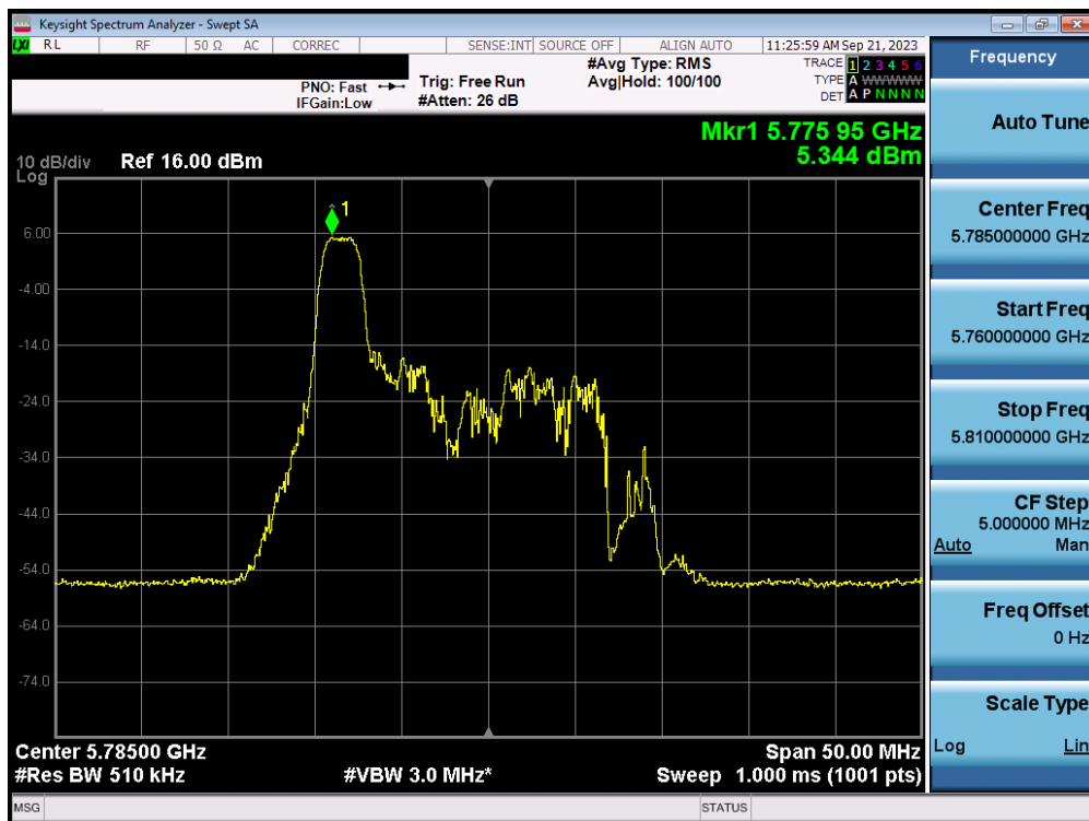
Plot 7-84. Power Spectral Density Plot MIMO ANT1 (20MHz BW 802.11be – 26 Tones (UNII Band 3) – Ch. 157)
