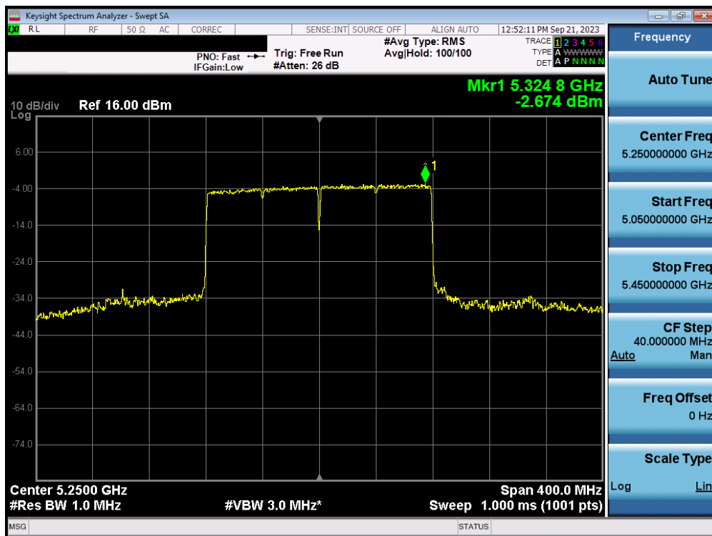
Plot 7-94. Power Spectral Density Plot MIMO ANT1 (160MHz BW 802.11be – 2x996 Tones (UNII Band 1/2A) – Ch. 50)
