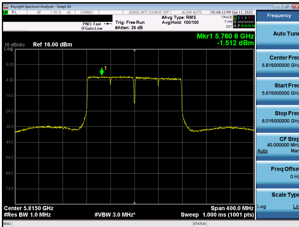
Plot 7-163. Power Spectral Density Plot MIMO ANT2 (160MHz BW 802.11ac (UNII Band 3/4) – Ch. 163)
