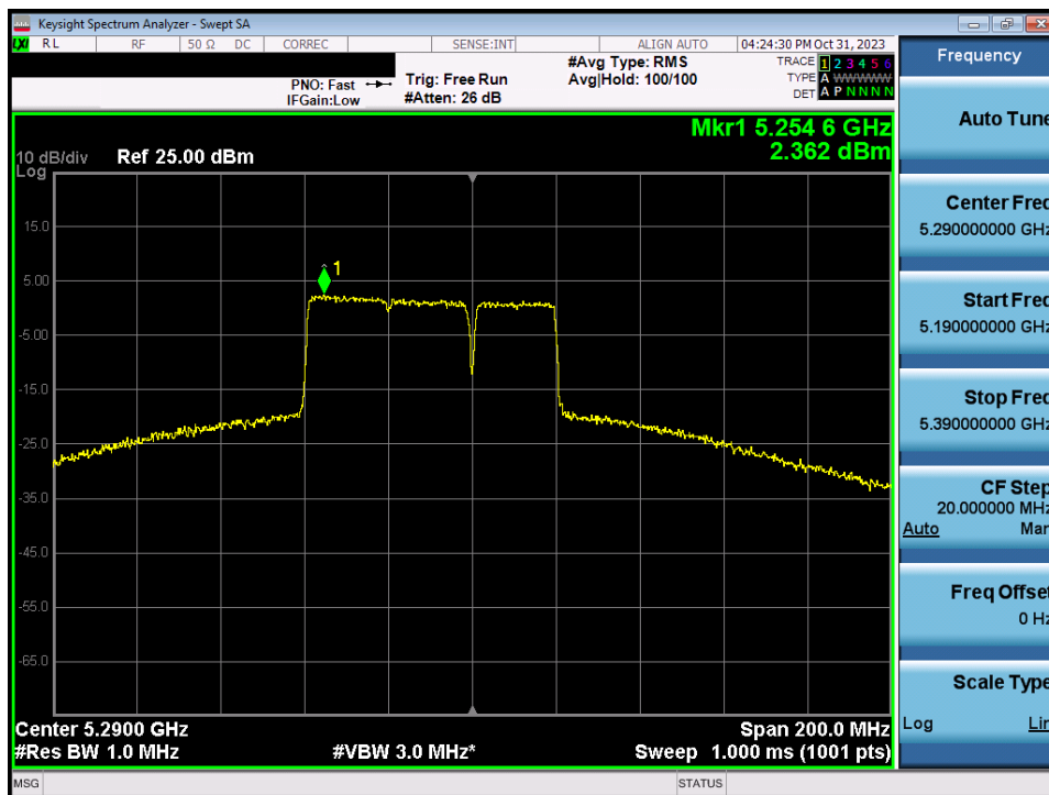
Plot 7-168. Power Spectral Density Plot MIMO ANT1 (80MHz BW 802.11be (UNII Band 2A) – Ch. 58)
