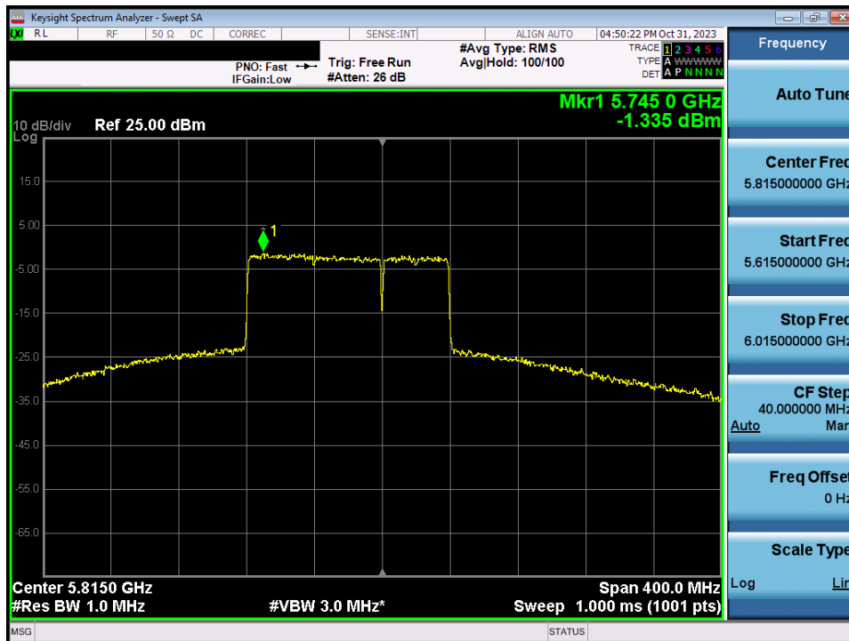
Plot 7-174. Power Spectral Density Plot MIMO ANT1 (160MHz BW 802.11be (UNII Band 3/4) – Ch. 163)
