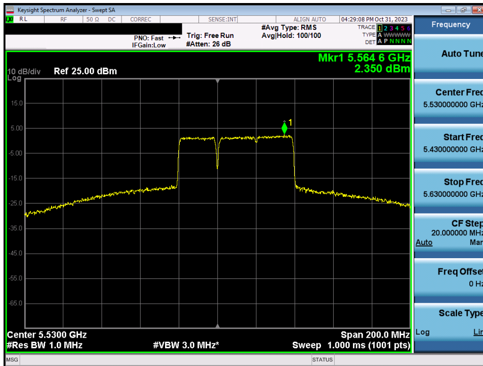
Plot 7-180. Power Spectral Density Plot MIMO ANT2 (80MHz BW 802.11be (UNII Band 2C) – Ch. 106)
