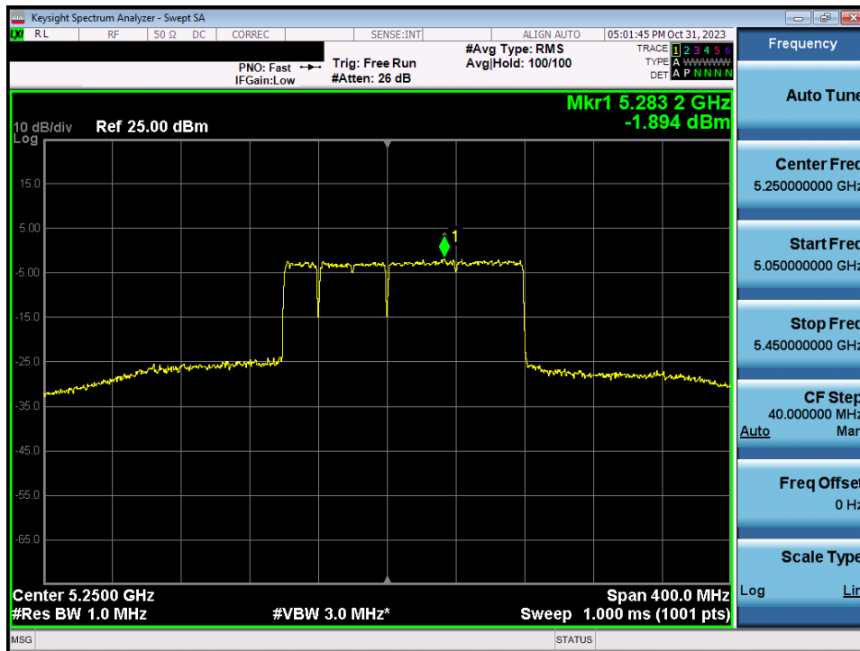
Plot 7-178. Power Spectral Density Plot MIMO ANT2 (160MHz BW 802.11be (UNII Band 1/2A) – Ch. 50)
