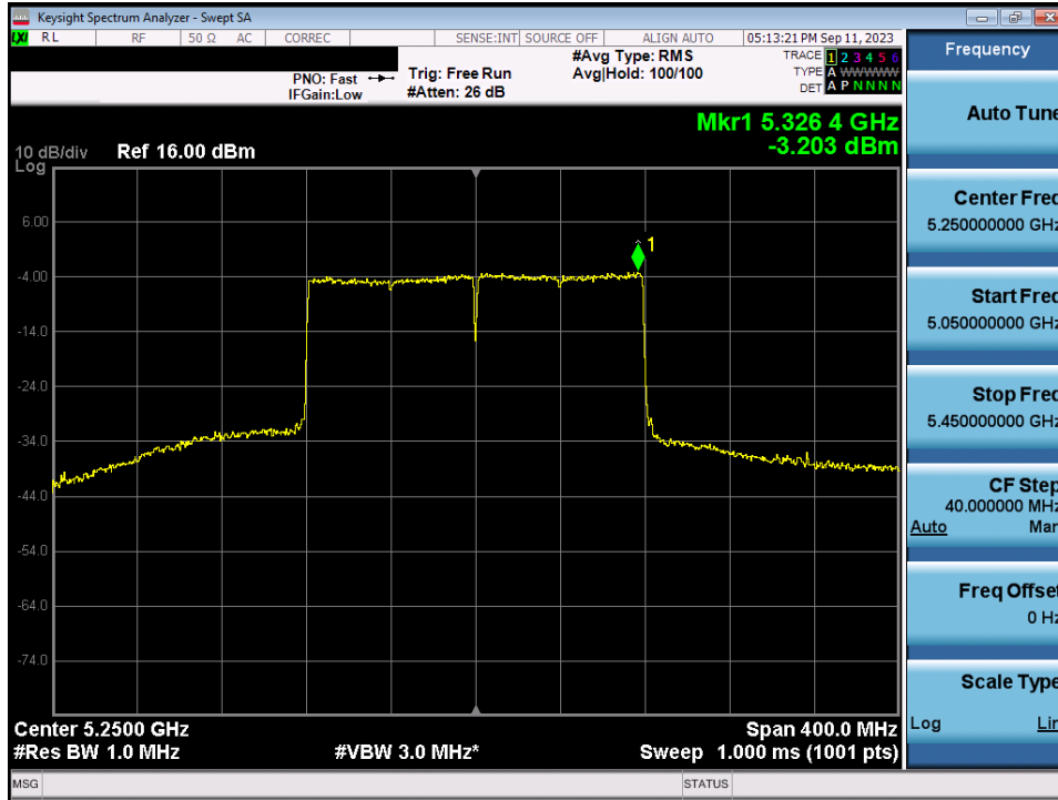
Plot 7-132. Power Spectral Density Plot MIMO ANT2 (160MHz BW 802. 11ax/be (UNII Band 1/2A) – Ch. 50)
