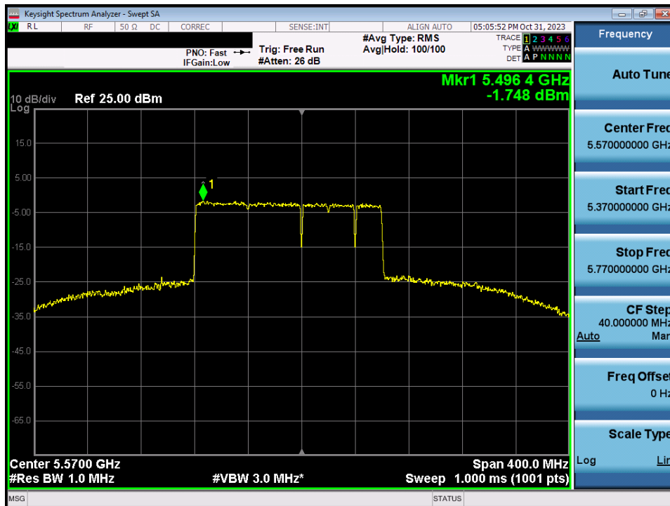
Plot 7-182. Power Spectral Density Plot MIMO ANT2 (160MHz BW 802.11be (UNII Band 2C) – Ch. 114)
