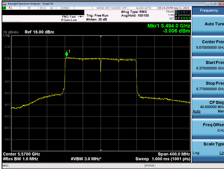
Plot 7-148. Power Spectral Density Plot MIMO ANT2 (160MHz BW 802.11ax/be (UNII Band 2C) – Ch. 114)
