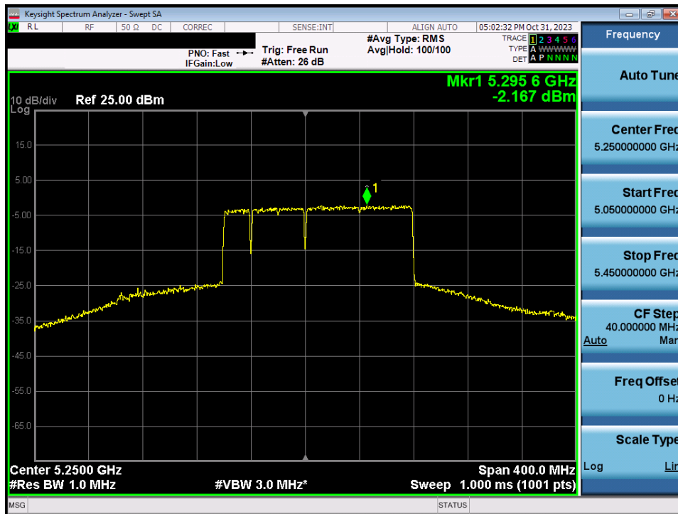
Plot 7-167. Power Spectral Density Plot MIMO ANT1 (160MHz BW 802.11be (UNII Band 1/2A) – Ch. 50)
