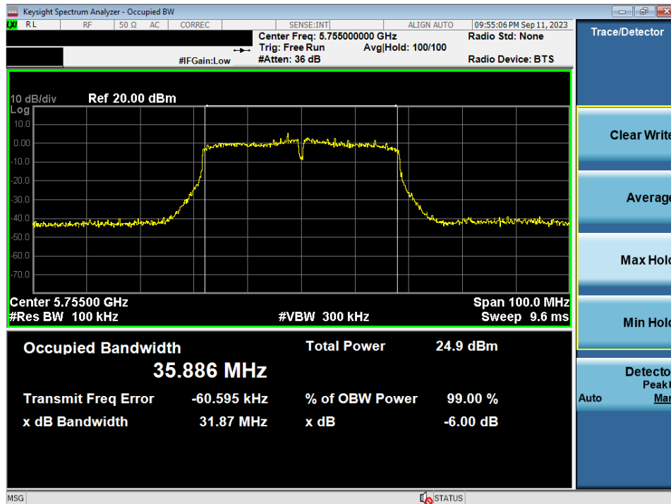
Plot 7-54. 6dB Bandwidth Plot MIMO ANT1 (40MHz BW 802.11n (UNII Band 3) – Ch. 151)
