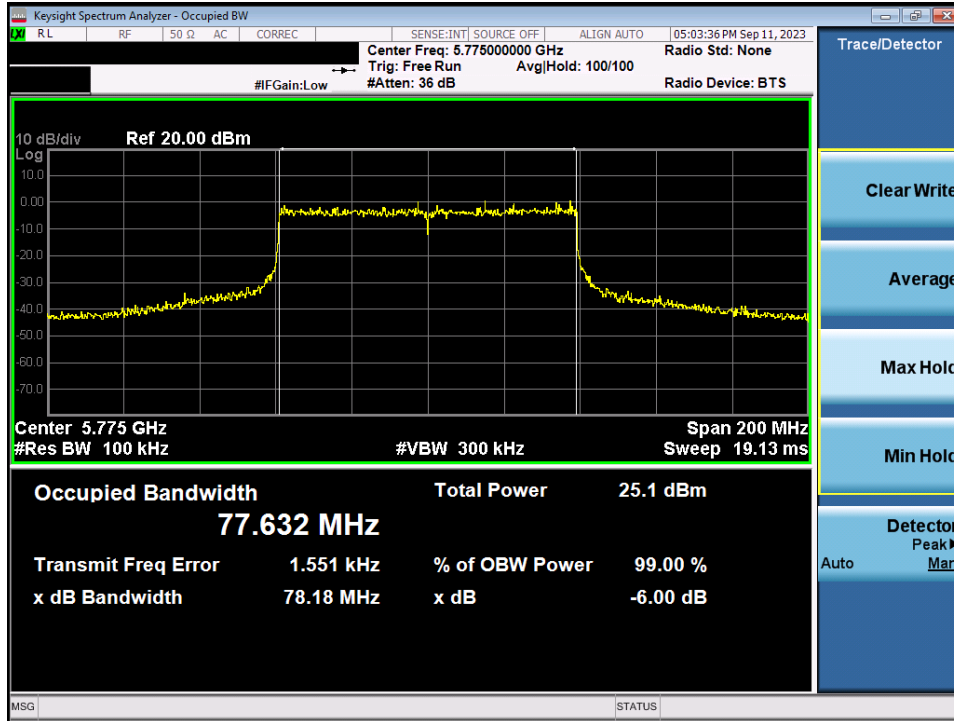
Plot 7-73. 6dB Bandwidth Plot MIMO ANT2 (80MHz BW 802.11ax/be (UNII Band 3) – Ch. 155)
