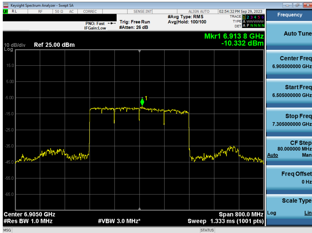
Plot 7-120. Power Spectral Density MIMO ANT2 (320MHz 802.11ax/be (UNII Band 7/8) – Ch. 191) - LPI
