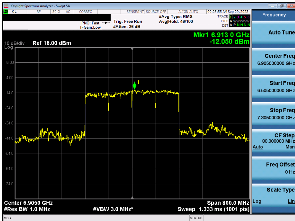
Plot 7-85. Power Spectral Density MIMO ANT1 (320MHz 802.11ax/be (UNII Band 7/8) – Ch. 191) - LPI
