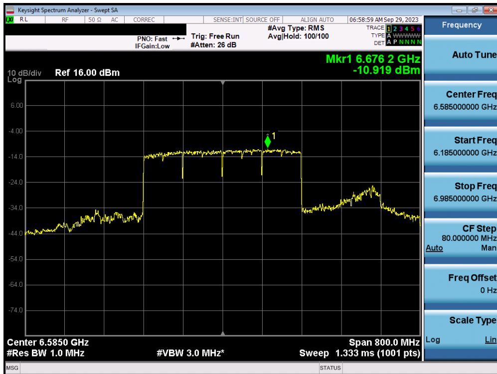
Plot 7-73. Power Spectral Density MIMO ANT1 (320MHz 802.11ax/be (UNII Band 6/7) – Ch. 127) - LPI
