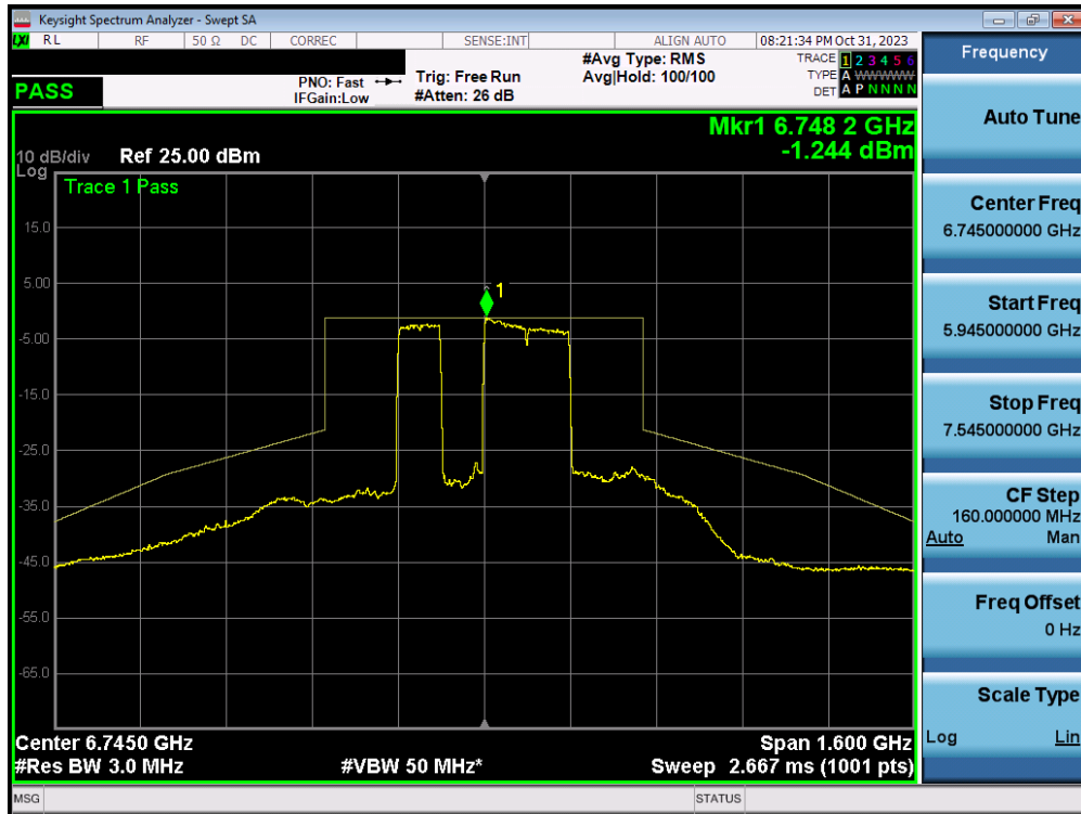
Plot 7-385. In-Band Emission Plot MIMO ANT2 (320MHz BW 802.11ax/be (MRU) (UNII Band 6/7) – Ch. 127) – LPI – 3x996T
