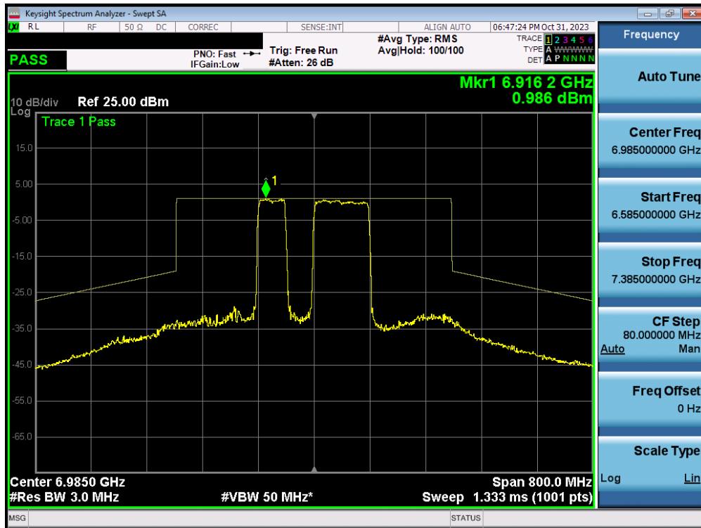
Plot 7-404. In-Band Emission Plot MIMO ANT2 (160MHz BW 802.11ax/be (MRU) (UNII Band 8) – Ch. 207) – LPI – 966+484T
