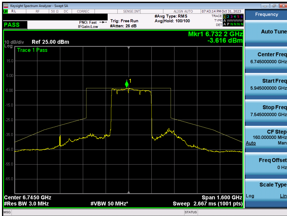
Plot 7-386. In-Band Emission Plot MIMO ANT2 (320MHz BW 802.11ax/be (MRU) (UNII Band 6/7) – Ch. 127) – LPI – 3x996+484T
