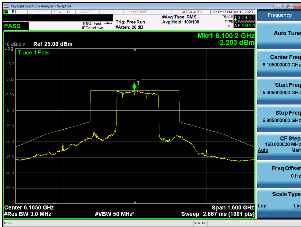
Plot 7-352. In-Band Emission Plot MIMO ANT2 (320MHz BW 802.11ax/be (MRU) (UNII Band 5) – Ch. 31) – LPI – 3x996+484T
