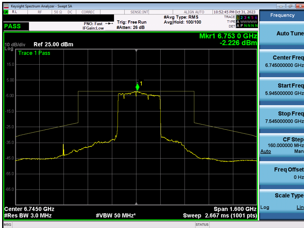
Plot 7-396. In-Band Emission Plot MIMO ANT2 (320MHz BW 802.11ax/be (MRU) (UNII Band 7) – Ch. 159) – SP – 3x996+484T
