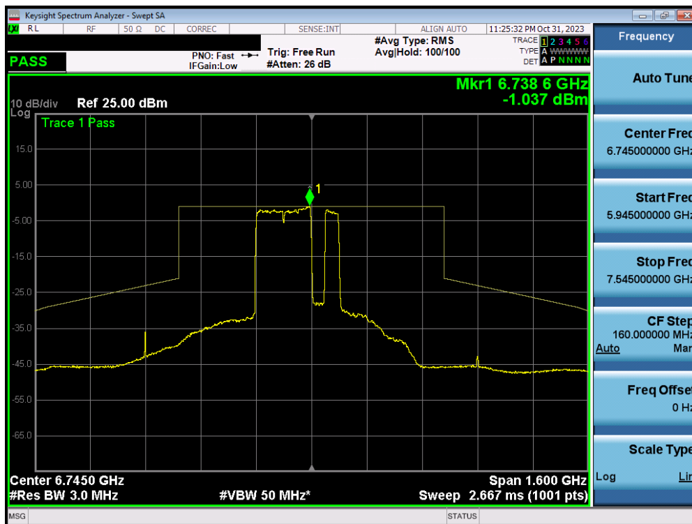
Plot 7-394. In-Band Emission Plot MIMO ANT2 (320MHz BW 802.11ax/be (MRU) (UNII Band 7) – Ch. 159) – SP – 2x996+484T
