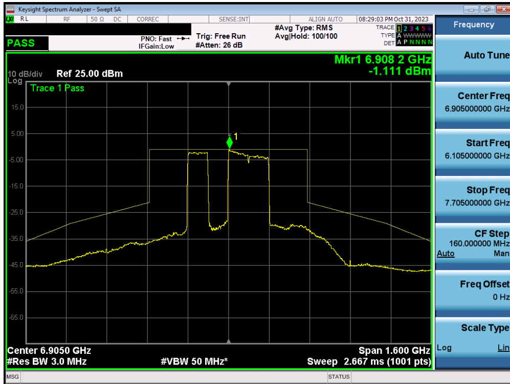
Plot 7-407. In-Band Emission Plot MIMO ANT2 (320MHz BW 802.11ax/be (MRU) (UNII Band 7/8) – Ch. 191) – LPI – 3x996T
