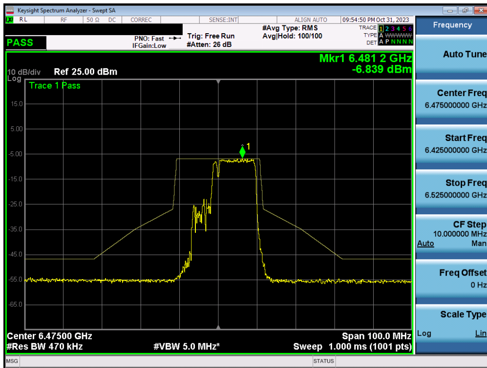
Plot 7-364. In-Band Emission Plot MIMO ANT2 (20MHz BW 802.11ax/be (MRU) (UNII Band 6) – Ch. 105) – LPI – 106+26T
