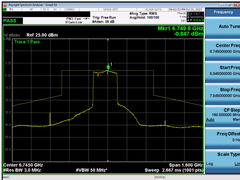
Plot 7-384. In-Band Emission Plot MIMO ANT2 (320MHz BW 802.11ax/be (MRU) (UNII Band 6/7) – Ch. 159) – LPI – 2x996+484T
