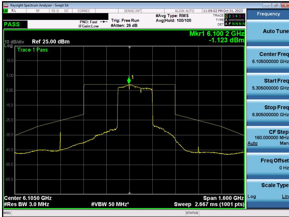
Plot 7-361. In-Band Emission Plot MIMO ANT2 (320MHz BW 802.11ax/be (MRU) (UNII Band 5) – Ch. 31) – SP – 3x996T
