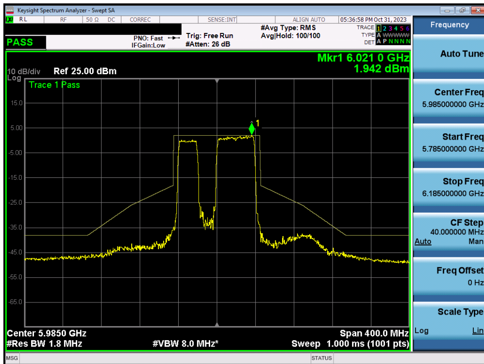
Plot 7-346. In-Band Emission Plot MIMO ANT2 (80MHz BW 802.11ax/be (MRU) (UNII Band 5) – Ch. 39) – LPI – 484+242T
