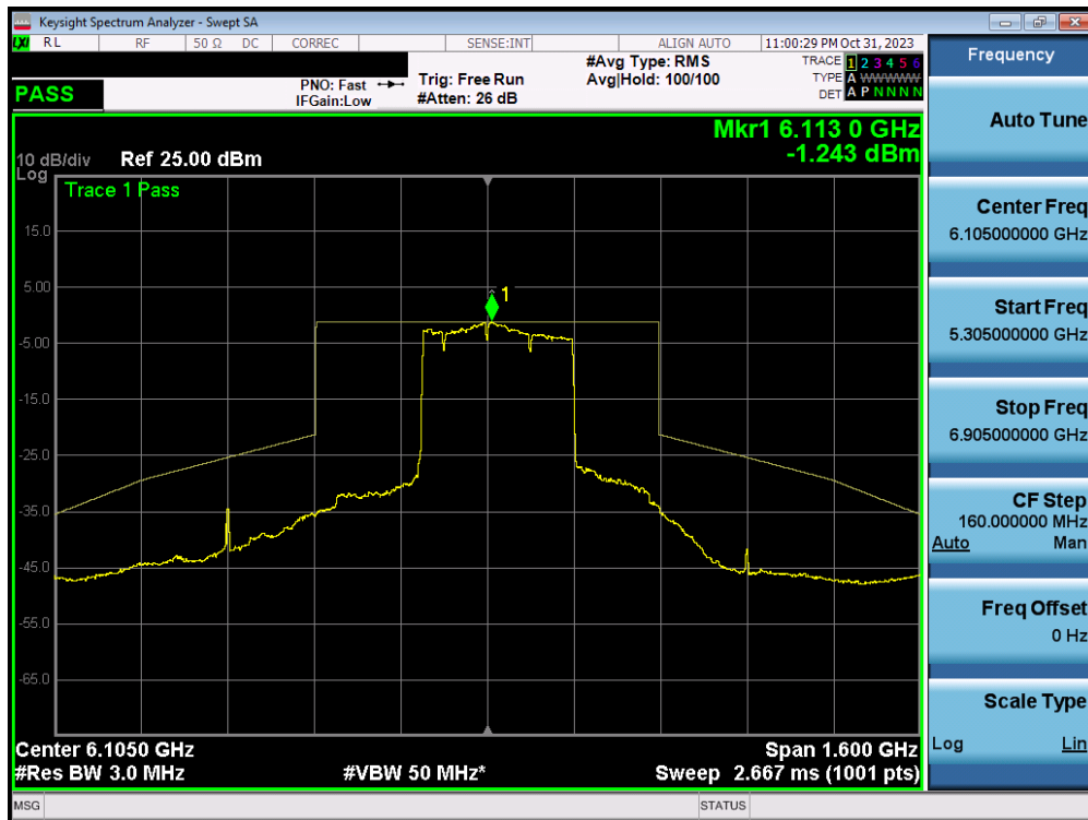
Plot 7-362. In-Band Emission Plot MIMO ANT2 (320MHz BW 802.11ax/be (MRU) (UNII Band 5) – Ch. 31) – SP – 3x996+484T
