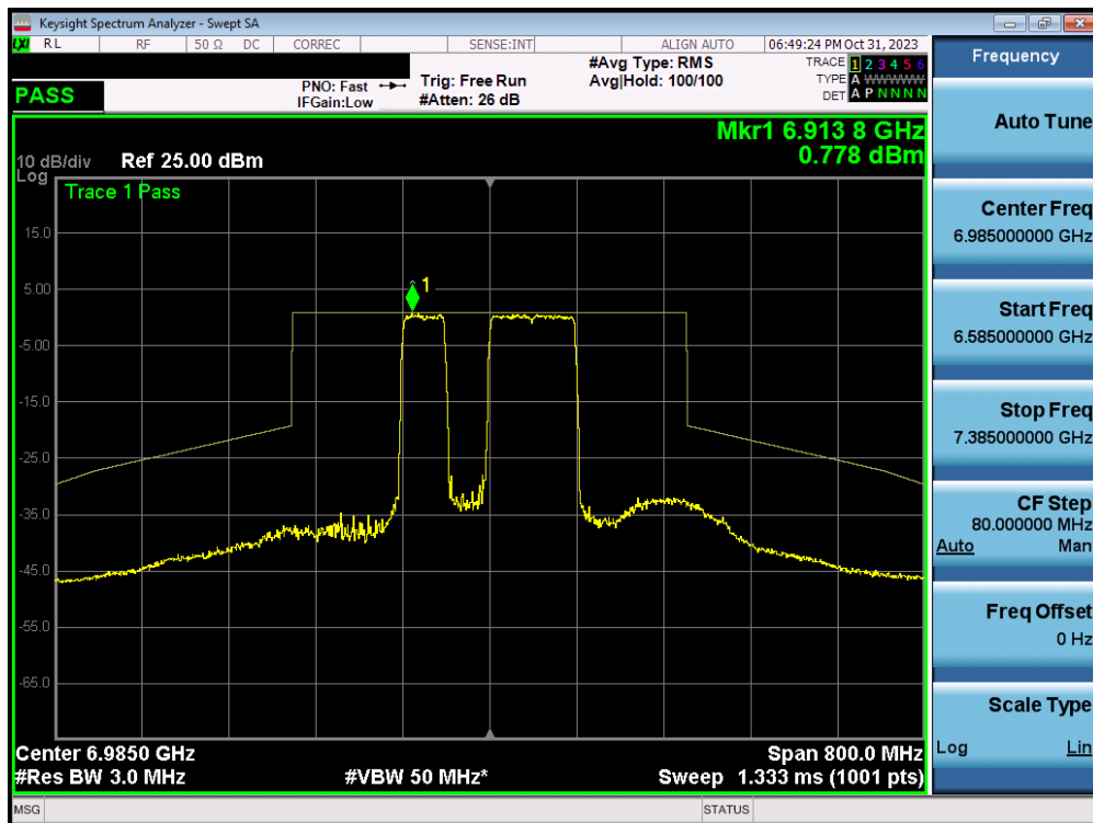
Plot 7-321. In-Band Emission Plot MIMO ANT1 (160MHz BW 802.11ax/be (MRU) (UNII Band 8) – Ch. 207) – LPI – 996+484T
