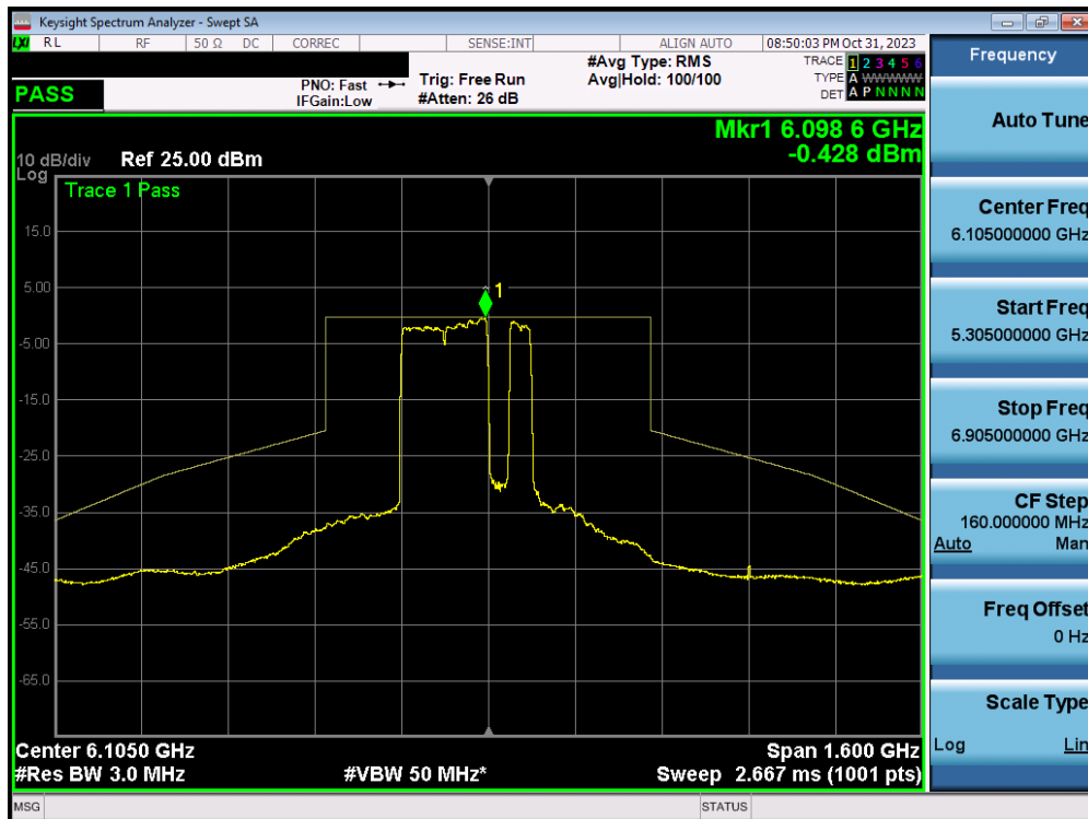
Plot 7-267. In-Band Emission Plot MIMO ANT1 (320MHz BW 802.11ax/be (MRU) (UNII Band 5) – Ch. 31) – LPI – 2x996+484T
