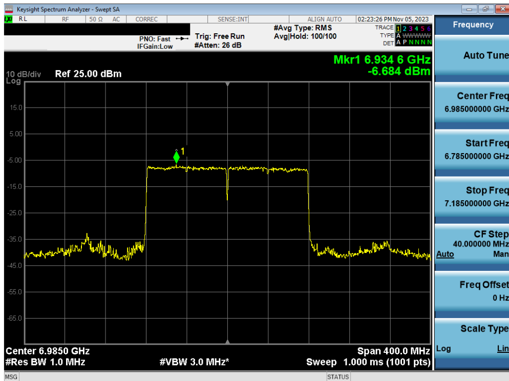
Plot 7-256. Power Spectral Density Plot MIMO ANT2 (160MHz BW 802.11ax/be (Full Tone) (UNII Band 8) – Ch. 207) – LPI
