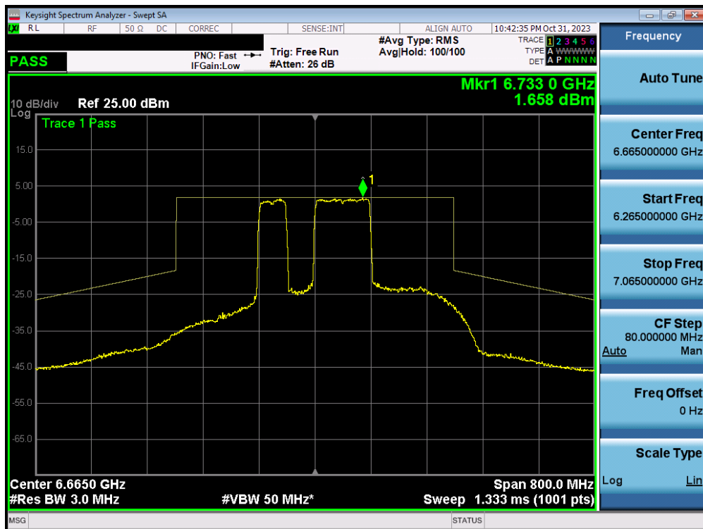
Plot 7-309. In-Band Emission Plot MIMO ANT1 (160MHz BW 802.11ax/be (MRU) (UNII Band 7) – Ch. 143) – SP – 996+484T
