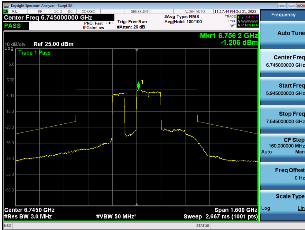
Plot 7-312. In-Band Emission Plot MIMO ANT1 (320MHz BW 802.11ax/be (MRU) (UNII Band 7) – Ch. 159) – SP – 3x996T
