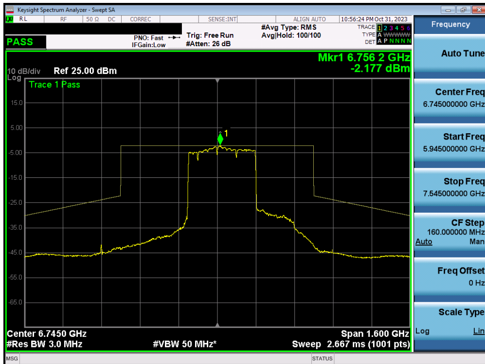
Plot 7-313. In-Band Emission Plot MIMO ANT1 (320MHz BW 802.11ax/be (MRU) (UNII Band 7) – Ch. 159) – SP – 3x996+484T
