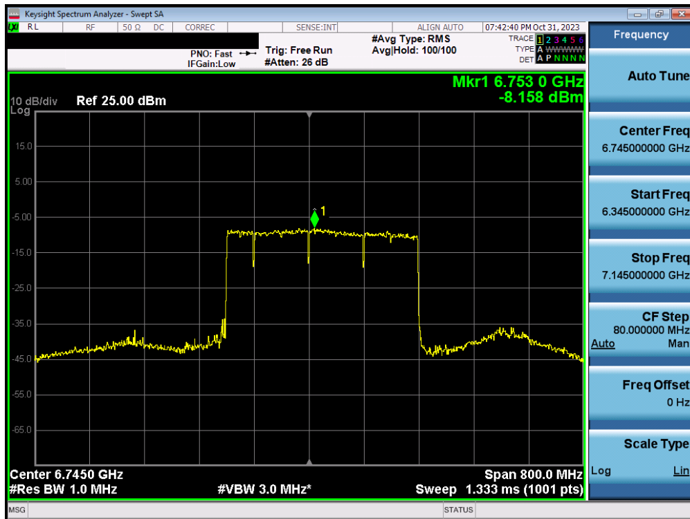
Plot 7-215. Power Spectral Density Plot MIMO ANT2 (320MHz BW 802.11ax/be (MRU) (UNII Band 7) – Ch. 159) – LPI – 3x996+484T
