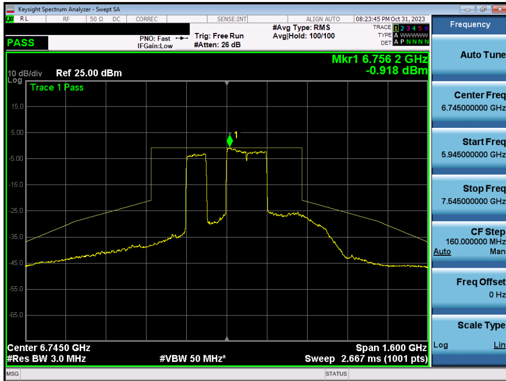
Plot 7-302. In-Band Emission Plot MIMO ANT1 (320MHz BW 802.11ax/be (MRU) (UNII Band 6/7) – Ch. 127) – LPI – 3x996T
