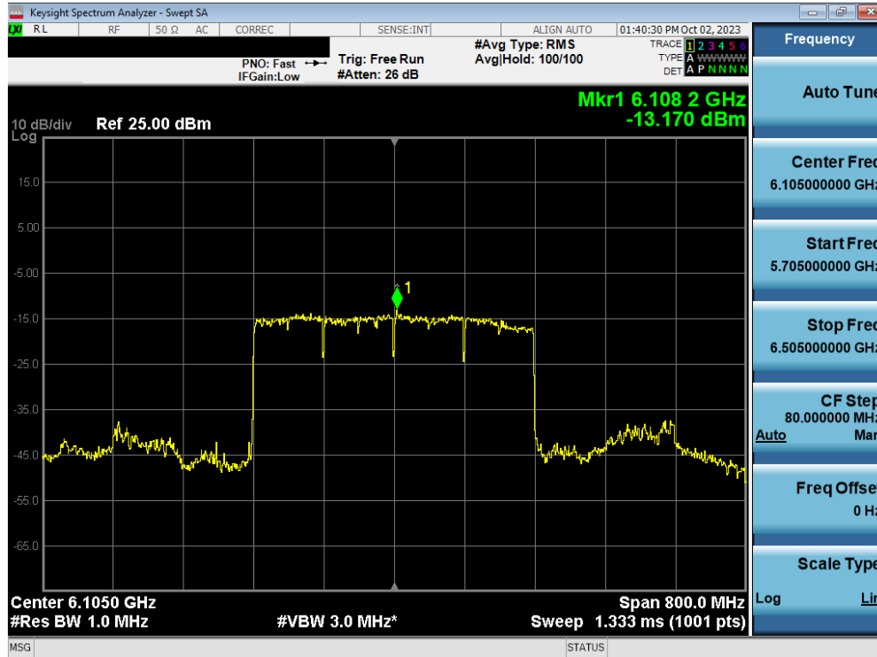
Plot 7-242. Power Spectral Density Plot MIMO ANT2 (320MHz BW 802.11ax/be (26 Tones) (UNII Band 5) – Ch. 31) – LPI
