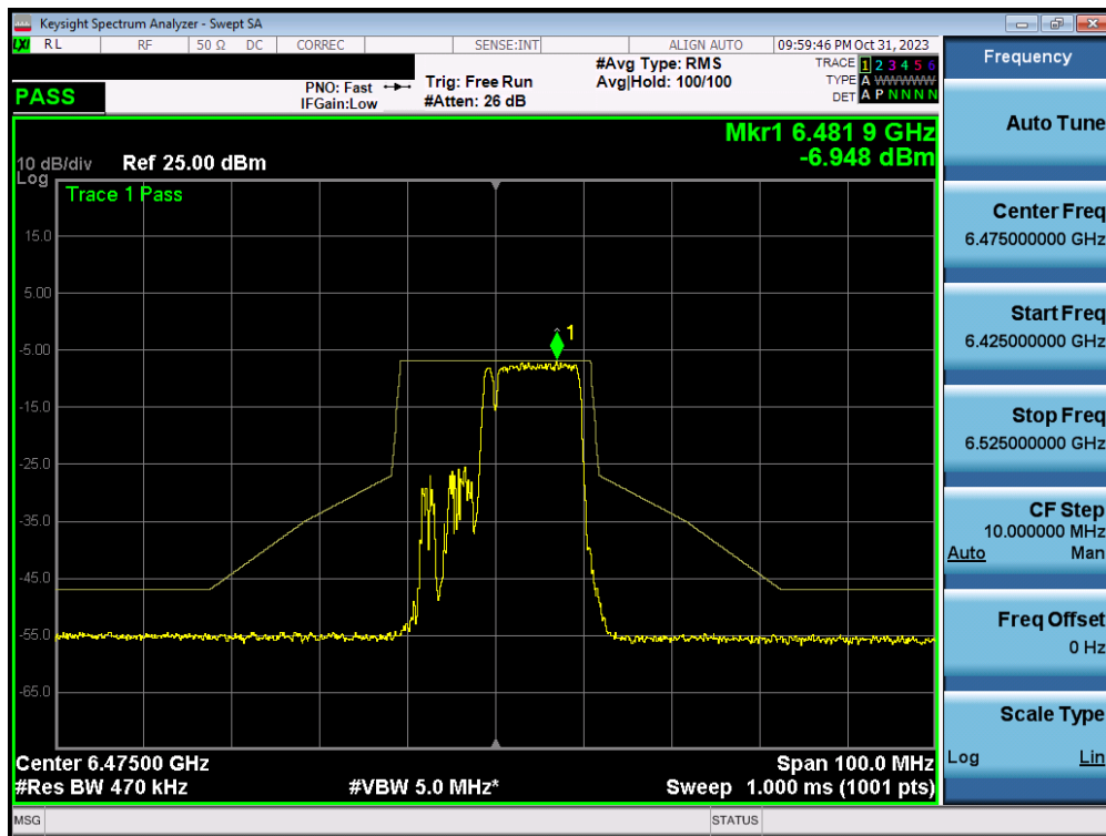
Plot 7-281. In-Band Emission Plot MIMO ANT1 (20MHz BW 802.11ax/be (MRU) (UNII Band 6) – Ch. 105) – LPI – 106+26T
