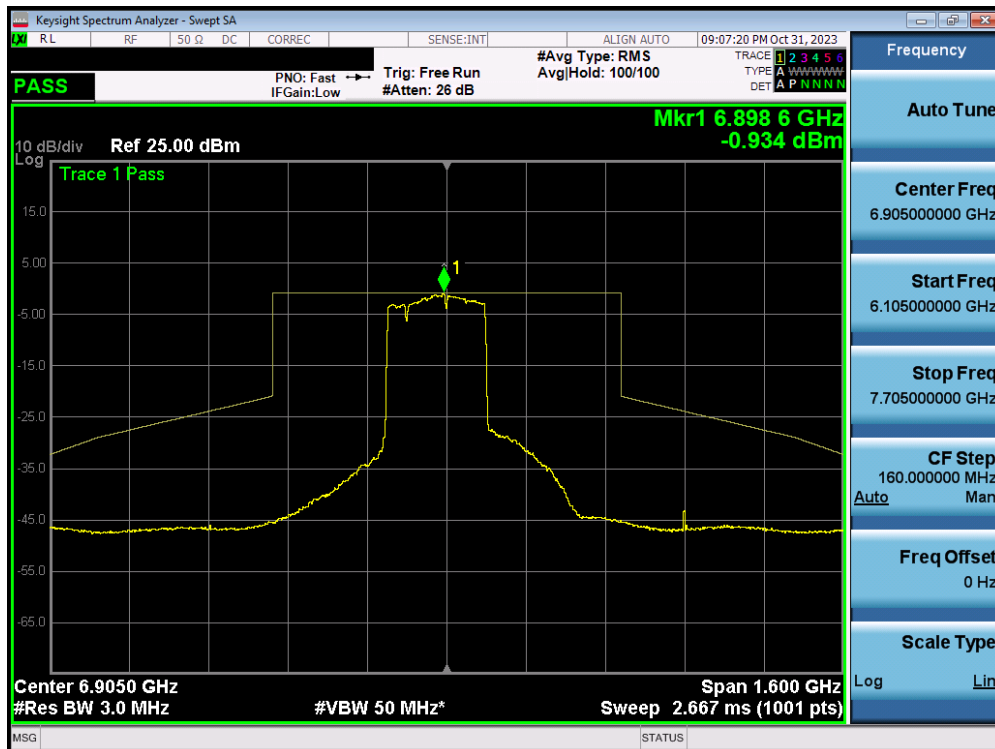
Plot 7-323. In-Band Emission Plot MIMO ANT1 (320MHz BW 802.11ax/be (MRU) (UNII Band 7/8) – Ch. 191) – LPI – 2x996+484T
