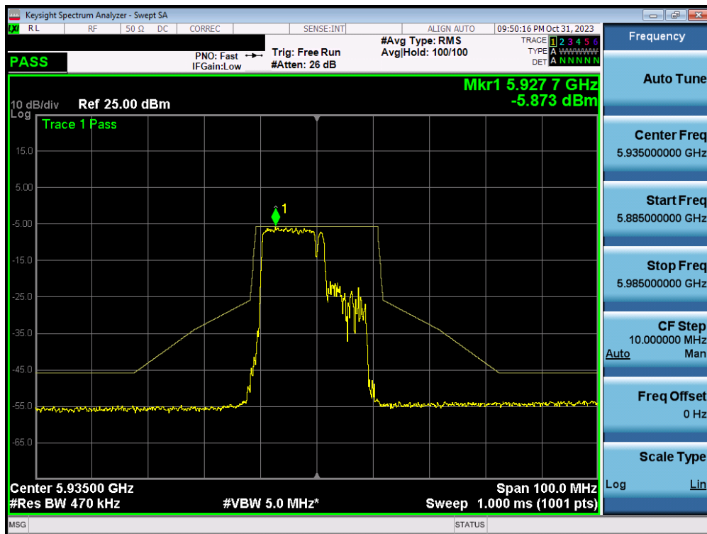
Plot 7-259. In-Band Emission Plot MIMO ANT1 (20MHz BW 802.11ax/be (MRU) (UNII Band 5) – Ch. 2) – LPI – 106+26T
