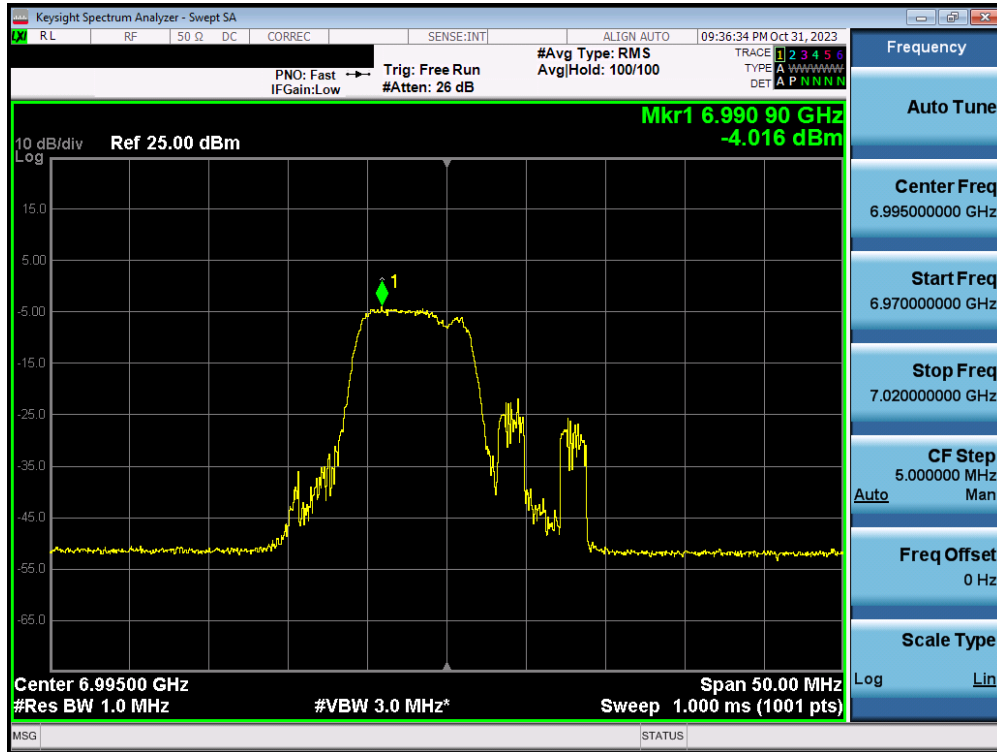
Plot 7-228. Power Spectral Density Plot MIMO ANT2 (20MHz BW 802.11ax/be (MRU) (UNII Band 8) – Ch. 209) – LPI – 52+26T
