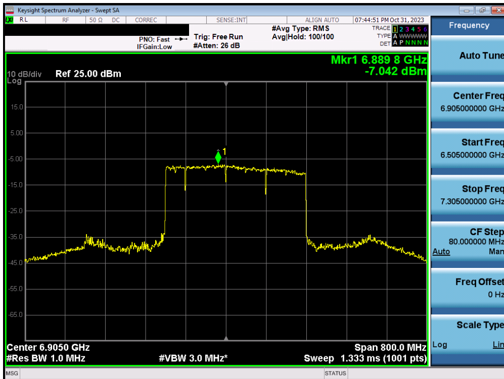
Plot 7-237. Power Spectral Density Plot MIMO ANT2 (320MHz BW 802.11ax/be (MRU) (UNII Band 7/8) – Ch. 191) – LPI – 3x996+484T
