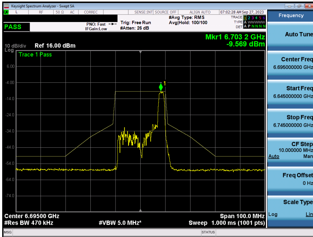
Plot 7-292. In-Band Emission Plot MIMO ANT1 (20MHz BW 802.11ax/be (26 Tones) (UNII Band 7) – Ch. 149) – LPI
