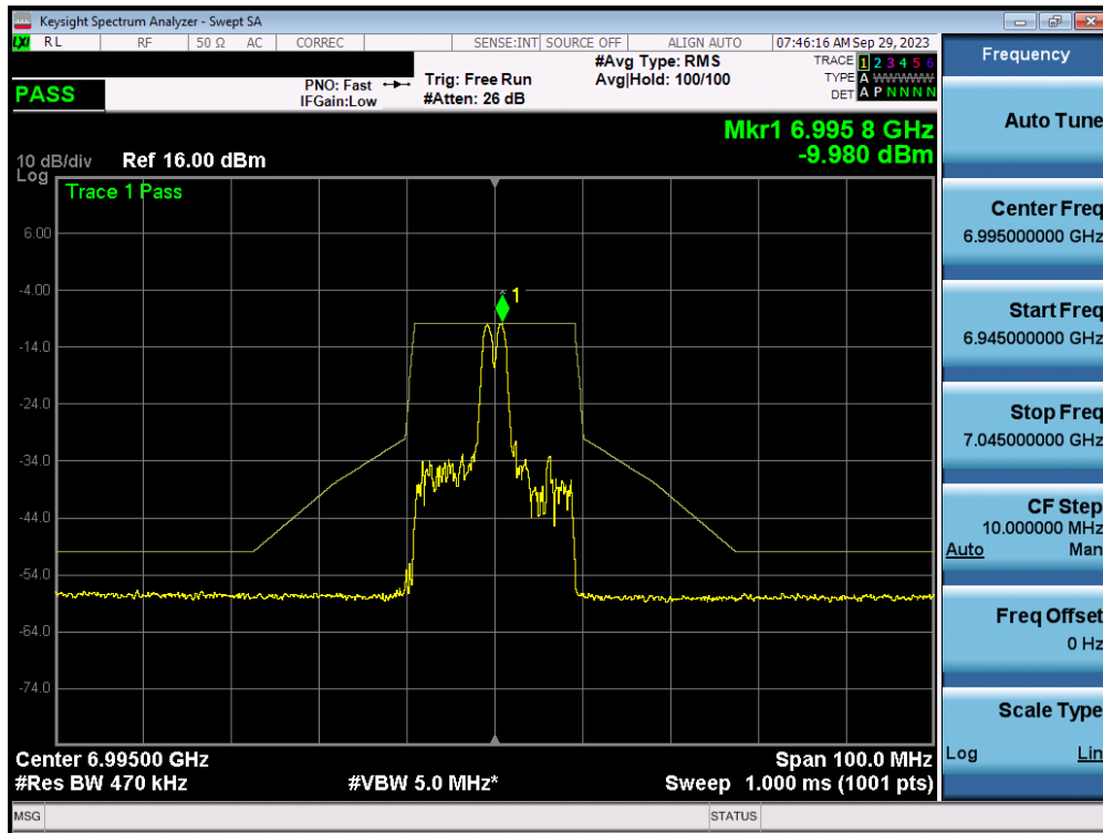
Plot 7-314. In-Band Emission Plot MIMO ANT1 (20MHz BW 802.11ax/be (26 Tones) (UNII Band 8) – Ch. 209) – LPI
