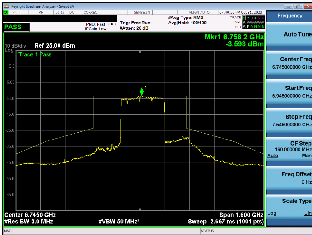
Plot 7-303. In-Band Emission Plot MIMO ANT1 (320MHz BW 802.11ax/be (MRU) (UNII Band 6/7) – Ch. 127) – LPI – 3x996+484T
