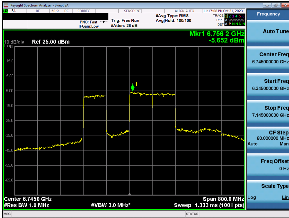
Plot 7-136. Power Spectral Density Plot MIMO ANT1 (320MHz BW 802.11ax/be (MRU) (UNII Band 7) – Ch. 159) – SP – 3x996T
