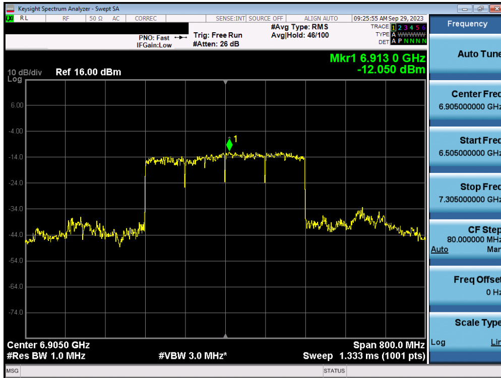
Plot 7-169. Power Spectral Density Plot MIMO ANT1 (320MHz BW 802.11ax/be (26 Tones) (UNII Band 8) – Ch. 191) – LPI
