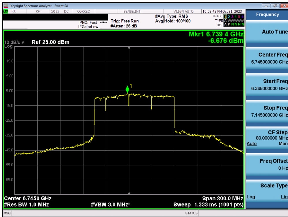
Plot 7-137. Power Spectral Density Plot MIMO ANT1 (320MHz BW 802.11ax/be (MRU) (UNII Band 7) – Ch. 159) – SP – 3x996+484T
