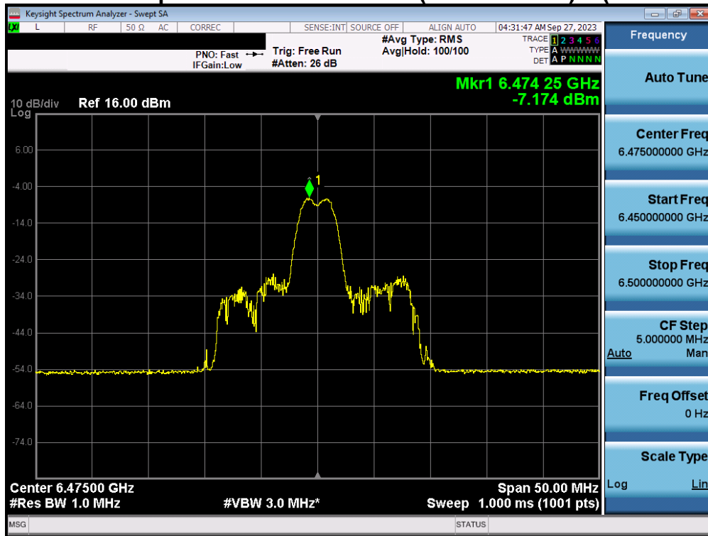
Plot 7-104. Power Spectral Density Plot MIMO ANT1 (20MHz BW 802.11ax/be (26 Tones) (UNII Band 6) – Ch. 105) – LPI
