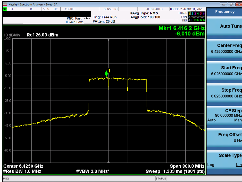
Plot 7-114. Power Spectral Density Plot MIMO ANT1 (320MHz BW 802.11ax/be (MRU) (UNII Band 5/6/7) – Ch. 95) – LPI – 3x996T
