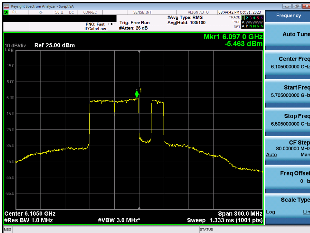
Plot 7-179. Power Spectral Density Plot MIMO ANT2 (320MHz BW 802.11ax/be (MRU) (UNII Band 5) – Ch. 31) – LPI – 2x996+484T
