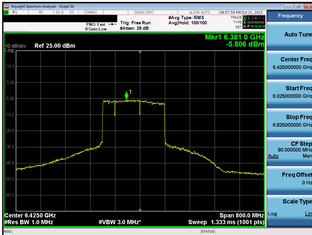
Plot 7-201. Power Spectral Density Plot MIMO ANT2 (320MHz BW 802.11ax/be (MRU) (UNII Band 5/6/7) – Ch. 95) – LPI – 2x996+484T
