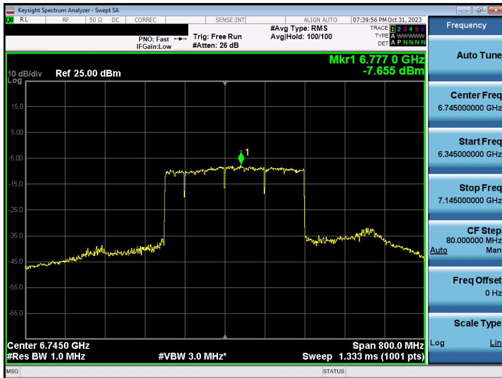
Plot 7-127. Power Spectral Density Plot MIMO ANT1 (320MHz BW 802.11ax/be (MRU) (UNII Band 6/7) – Ch. 127) – LPI – 3x996+484T
