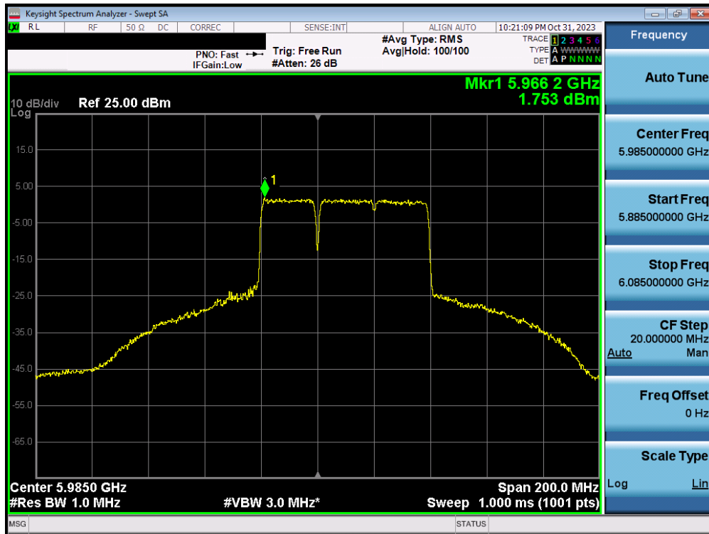
Plot 7-185. Power Spectral Density Plot MIMO ANT2 (80MHz BW 802.11ax/be (MRU) (UNII Band 5) – Ch. 7) – SP – 484+242T
