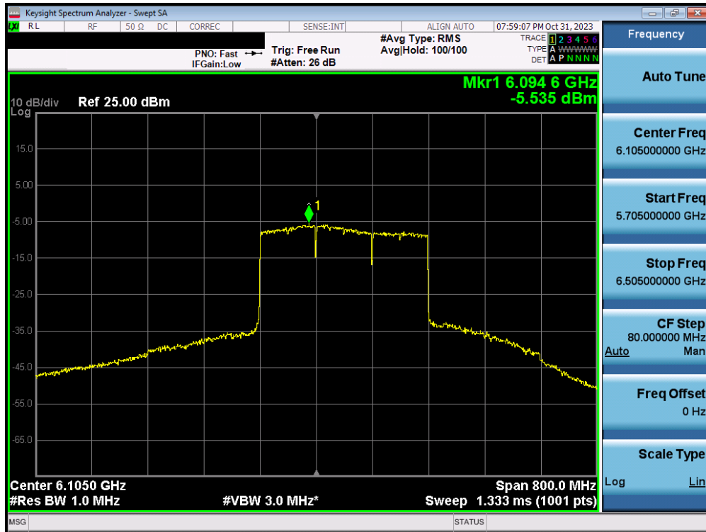
Plot 7-180. Power Spectral Density Plot MIMO ANT2 (320MHz BW 802.11ax/be (MRU) (UNII Band 5) – Ch. 31) – LPI
