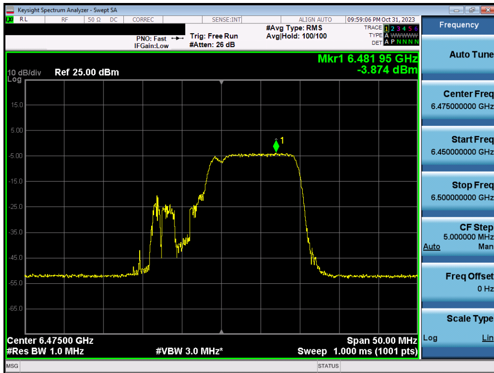
Plot 7-105. Power Spectral Density Plot MIMO ANT1 (20MHz BW 802.11ax/be (MRU) (UNII Band 6) – Ch. 105) – LPI – 106+26T
