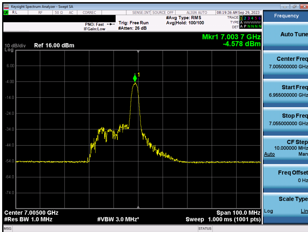
Plot 7-141. Power Spectral Density Plot MIMO ANT1 (40MHz BW 802.11ax/be (26 Tones) (UNII Band 8) – Ch. 211) – LPI
