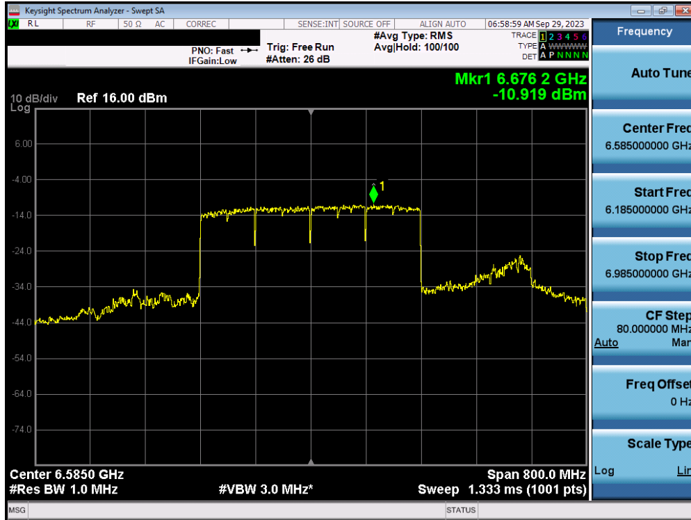
Plot 7-164. Power Spectral Density Plot MIMO ANT1 (320MHz BW 802.11ax/be (26 Tones) (UNII Band 6/7) – Ch. 127) – LPI
