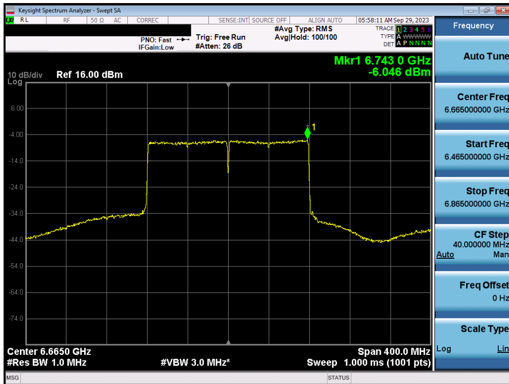
Plot 7-163. Power Spectral Density Plot MIMO ANT1 (160MHz BW 802.11ax/be (Full Tone) (UNII Band 7) – Ch. 143) – LPI
