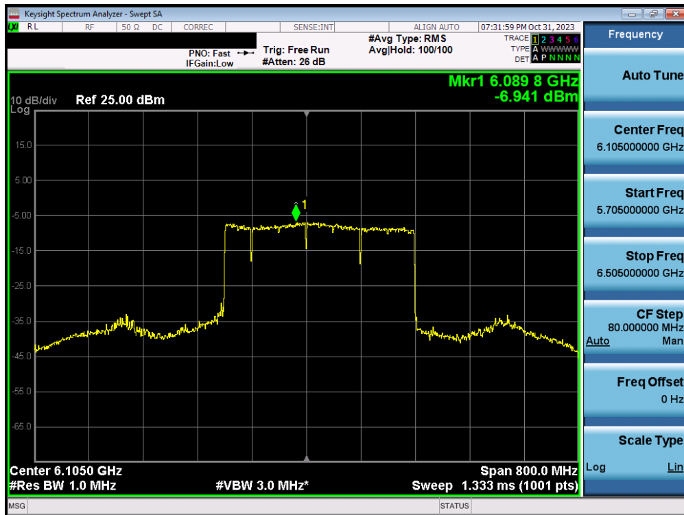
Plot 7-181. Power Spectral Density Plot MIMO ANT2 (320MHz BW 802.11ax/be (MRU) (UNII Band 5) – Ch. 31) – LPI – 3x996+484T
