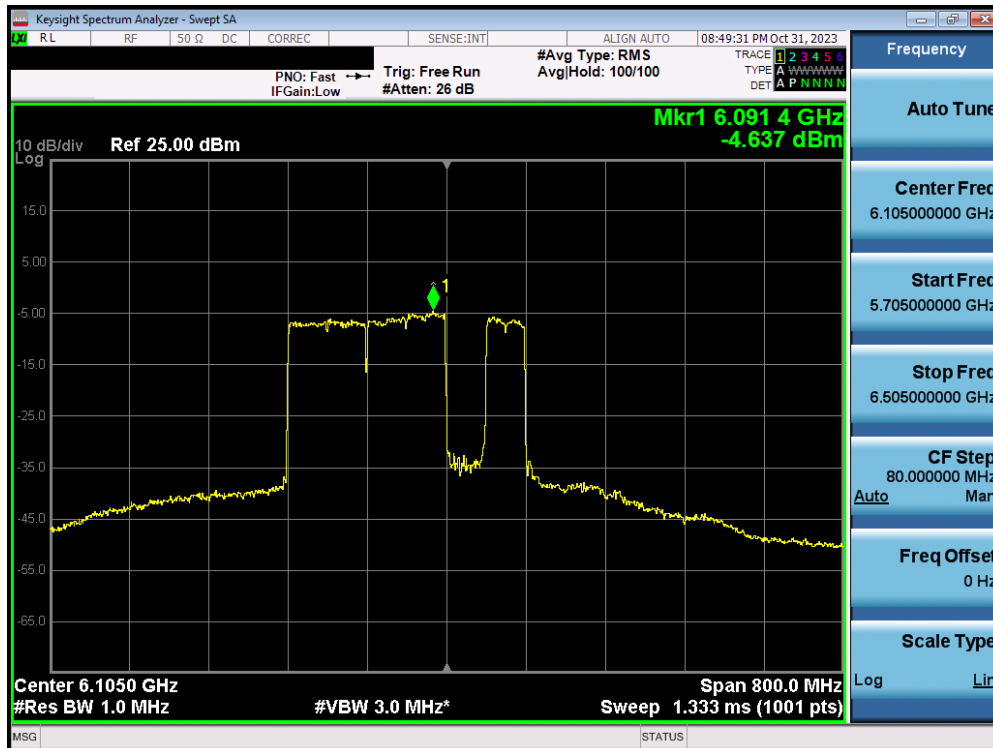
Plot 7-91. Power Spectral Density Plot MIMO ANT1 (320MHz BW 802.11ax/be (MRU) (UNII Band 5) – Ch. 31) – LPI – 2x996+484T
