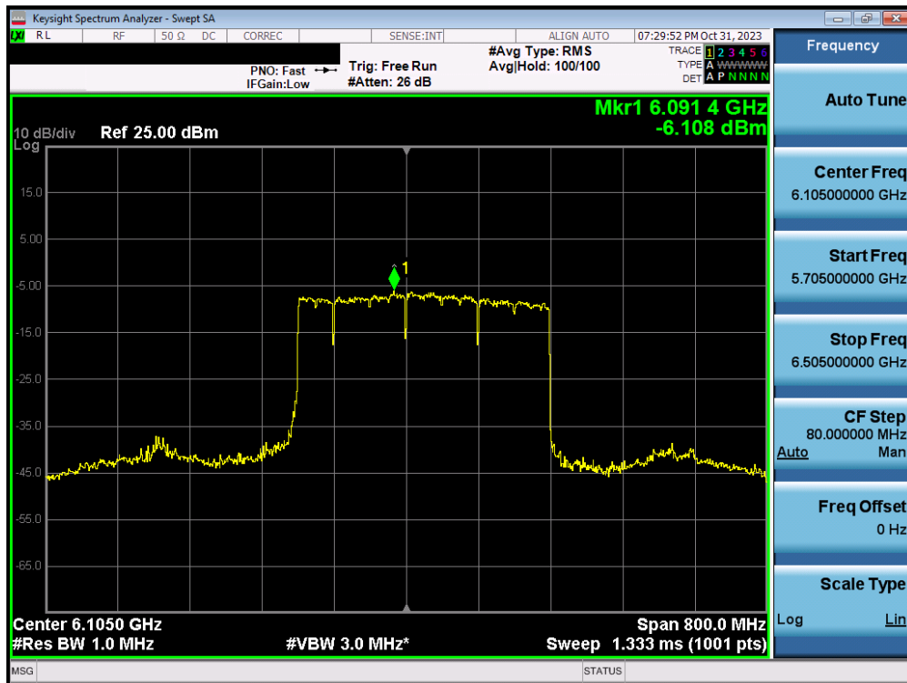
Plot 7-93. Power Spectral Density Plot MIMO ANT1 (320MHz BW 802.11ax/be (MRU) (UNII Band 5) – Ch. 31) – LPI – 3x996+484T
