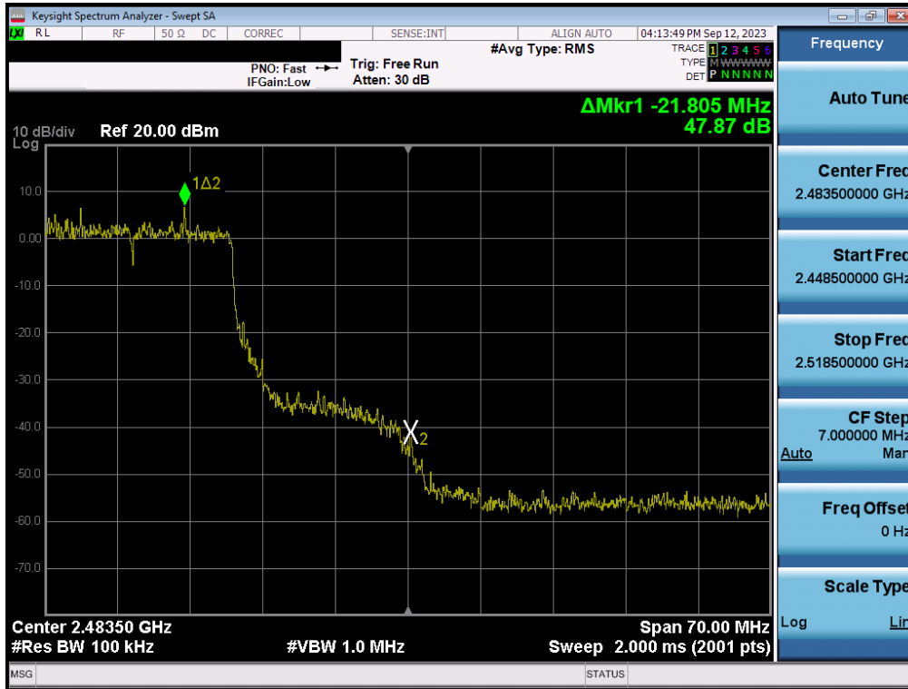
Plot 7-149. Band Edge Plot MIMO ANT2 (802.11be (2.4GHz) – Ch. 10)
