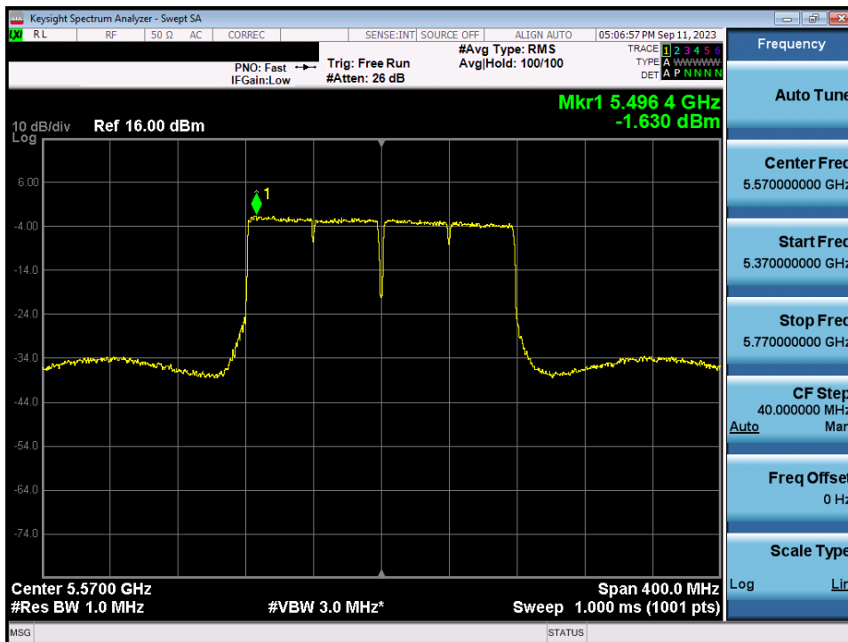
Plot 7-147. Power Spectral Density Plot MIMO ANT2 (160MHz BW 802.11ac (UNII Band 2C) – Ch. 114)
