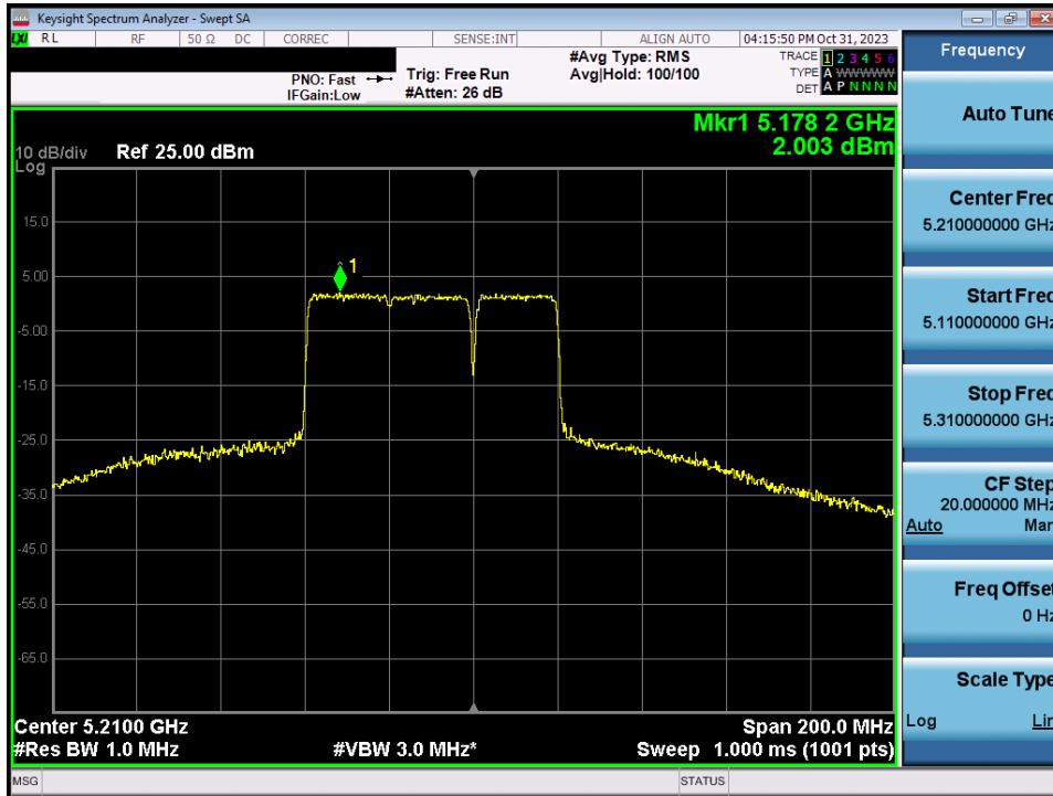
Plot 7-165. Power Spectral Density Plot MIMO ANT1 (80MHz BW 802.11be (UNII Band 1) – Ch. 42)
