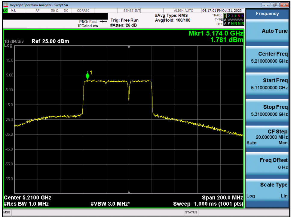
Plot 7-176. Power Spectral Density Plot MIMO ANT2 (80MHz BW 802.11be (UNII Band 1) – Ch. 42)
