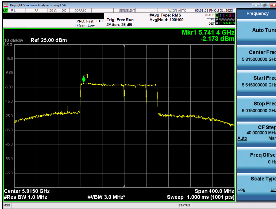
Plot 7-175. Power Spectral Density Plot MIMO ANT1 (160MHz BW 802.11be (UNII Band 3/4) – Ch. 163)
