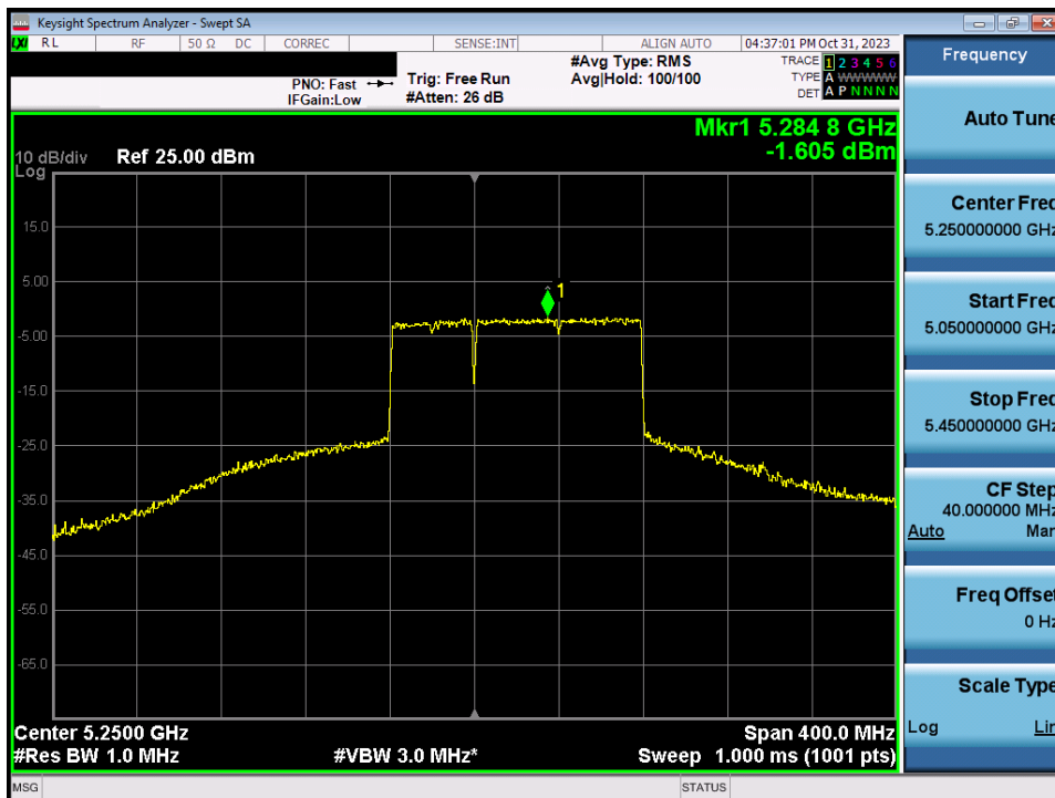
Plot 7-166. Power Spectral Density Plot MIMO ANT1 (160MHz BW 802.11be (UNII Band 1/2A) – Ch. 50)
