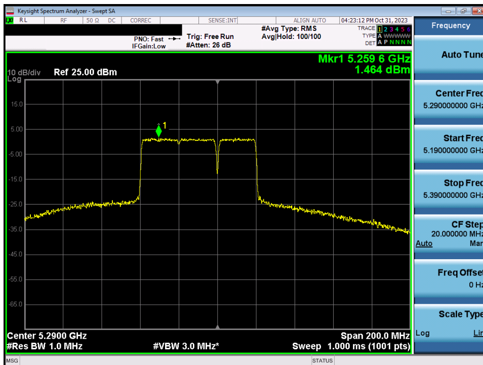
Plot 7-179. Power Spectral Density Plot MIMO ANT2 (80MHz BW 802.11be (UNII Band 2A) – Ch. 58)
