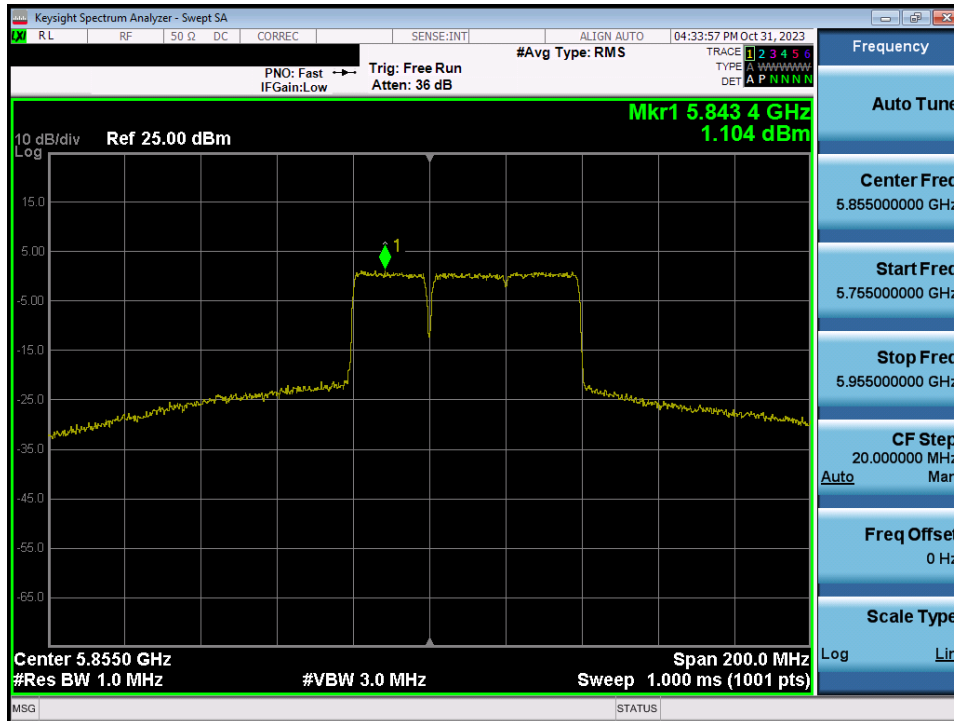
Plot 7-184. Power Spectral Density Plot MIMO ANT2 (80MHz BW 802.11be (UNII Band 3/4) – Ch. 171)
