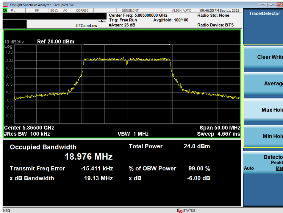
Plot 7-60. 6dB Bandwidth Plot MIMO ANT1 (20MHz BW 802.11ax/be (UNII Band 4) – Ch. 173)
