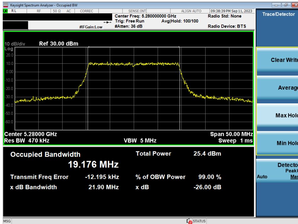
Plot 7-12. 26dB Bandwidth Plot MIMO ANT1 (20MHz BW 802.11ax/be (UNII Band 2A) – Ch. 56)
