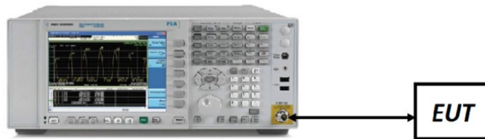
Figure 7-3. Test Instrument & Measurement Setup
