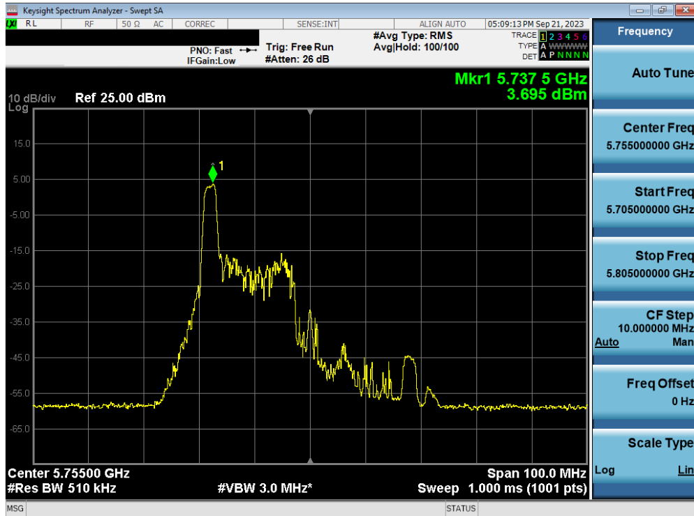
Plot 7-121. Power Spectral Density Plot MIMO ANT2 (40MHz BW 802.11be – 26 Tones (UNII Band 3) – Ch. 151)
