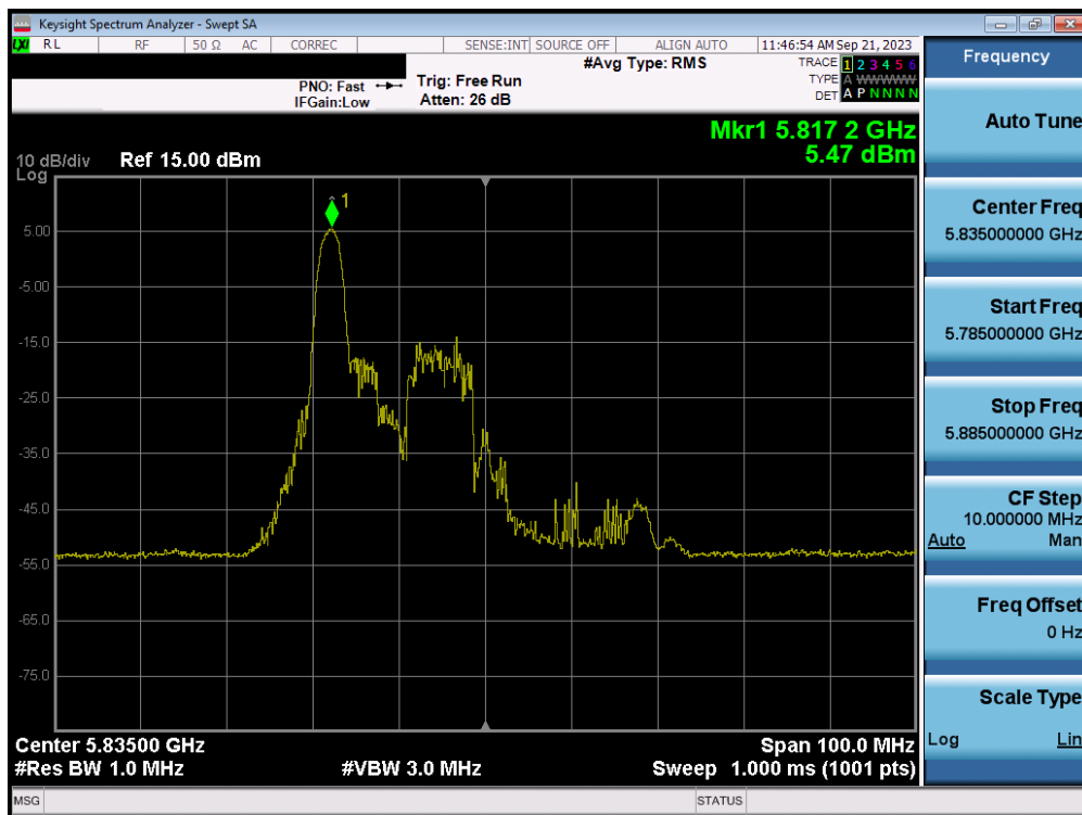
Plot 7-88. Power Spectral Density Plot MIMO ANT1 (40MHz BW 802.11be – 26 Tones (UNII Band 3/4) – Ch. 167)
