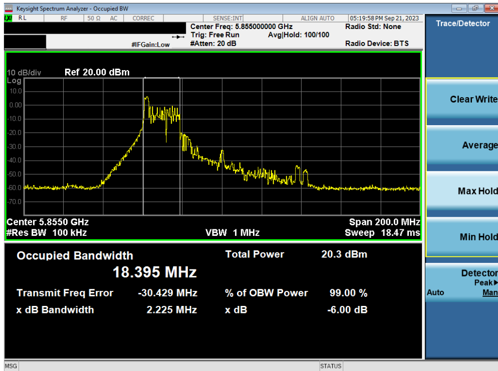
Plot 7-64. 6dB Bandwidth Plot MIMO ANT2 (80MHz BW 802.11be – 26 Tones (UNII Band 3/4) – Ch. 171)
