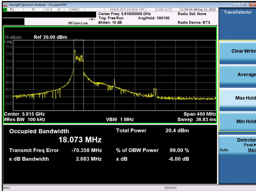
Plot 7-51. 6dB Bandwidth Plot MIMO ANT1 (160MHz(U) BW 802.11be – 26 Tones (UNII Band 3/4) – Ch. 163)
