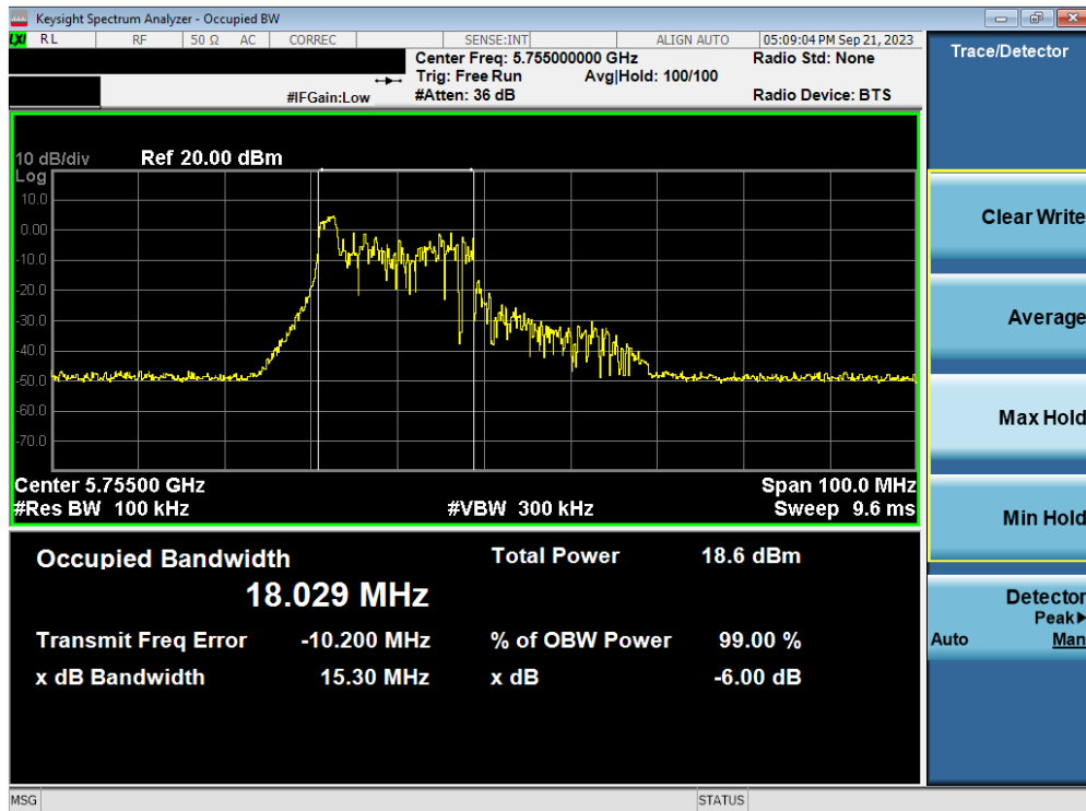
Plot 7-60. 6dB Bandwidth Plot MIMO ANT2 (40MHz BW 802.11be – 26 Tones (UNII Band 3) – Ch. 151)
