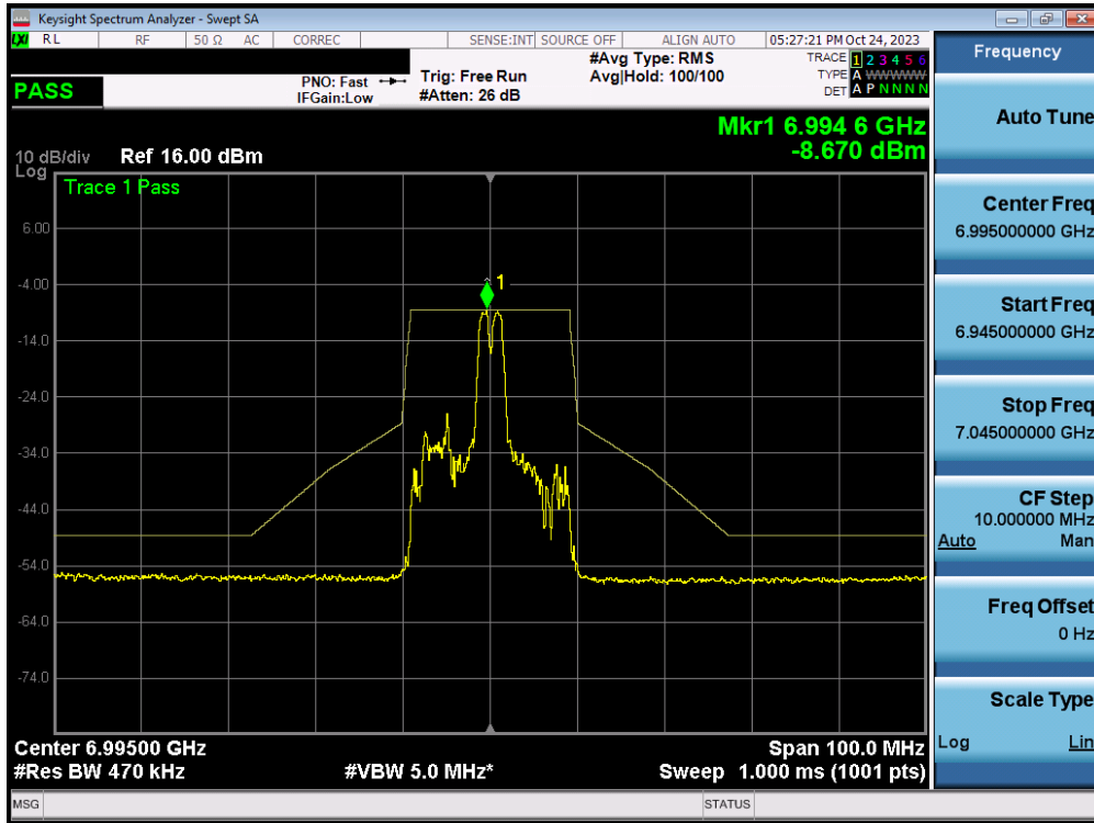
Plot 7-446. In-Band Emission Plot MIMO ANT2 (20MHz BW 802.11ax/be (26 Tones) (UNII Band 8) – Ch. 209) – LPI
