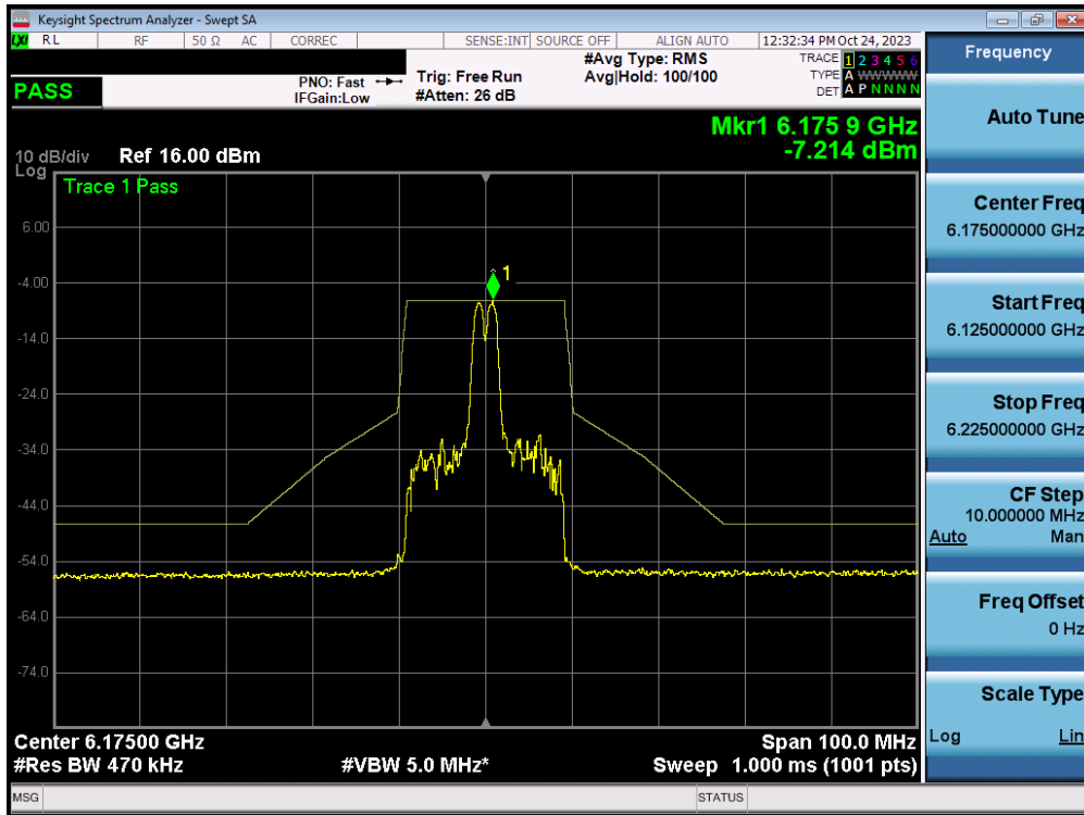
Plot 7-386. In-Band Emission Plot MIMO ANT2 (20MHz BW 802.11ax/be (26 Tones) (UNII Band 5) – Ch. 45) – LPI
