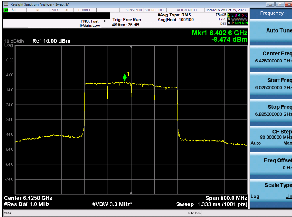
Plot 7-268. Power Spectral Density Plot MIMO ANT2 (320MHz BW 802.11ax/be (Full Tones) (UNII Band 5/6/7) – Ch. 95) – LPI
