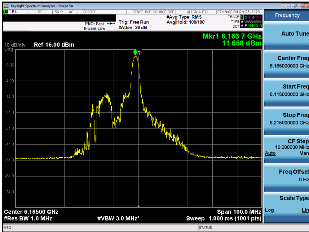
Plot 7-197. Power Spectral Density Plot MIMO ANT2 (40MHz BW 802.11ax/be (26 Tones) (UNII Band 5) – Ch. 43) – SP
