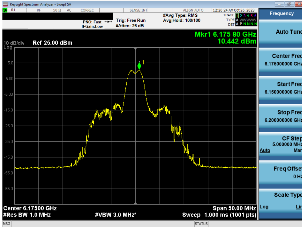
Plot 7-92. Power Spectral Density Plot MIMO ANT1 (20MHz BW 802.11ax/be (26 Tones) (UNII Band 5) – Ch. 45) – SP
