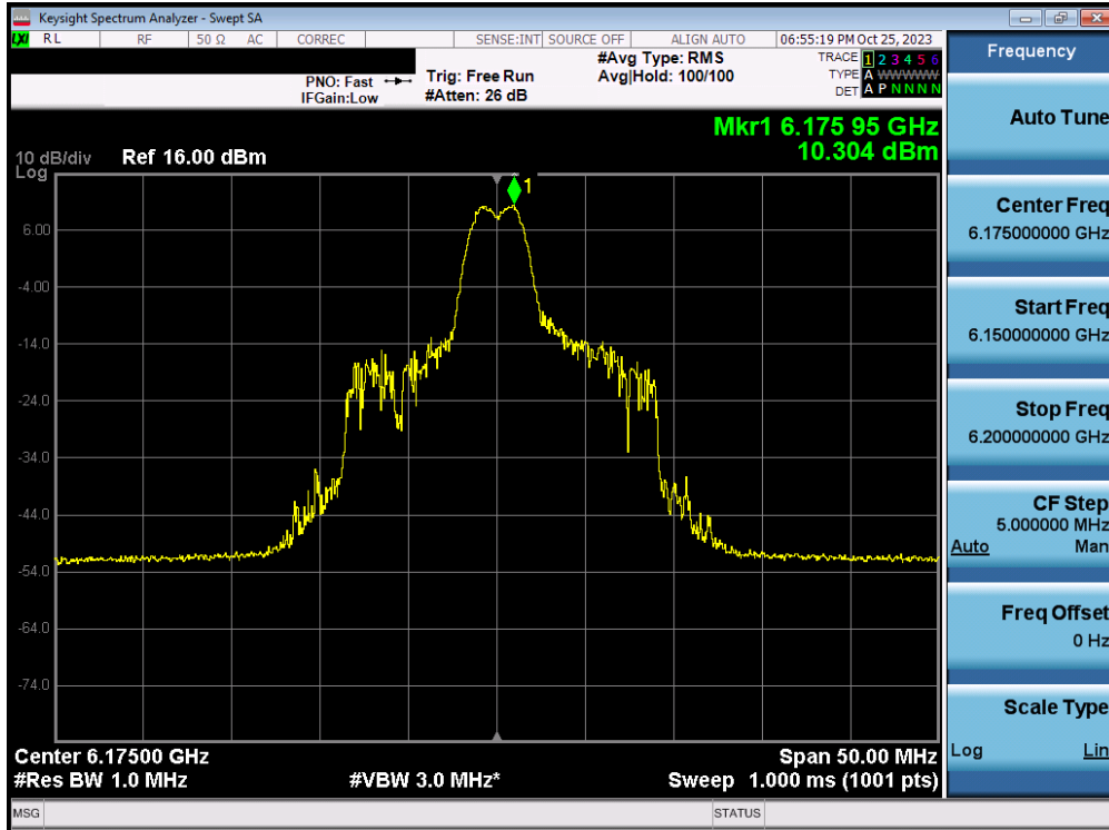
Plot 7-194. Power Spectral Density Plot MIMO ANT2 (20MHz BW 802.11ax/be (26 Tones) (UNII Band 5) – Ch. 45) – SP
