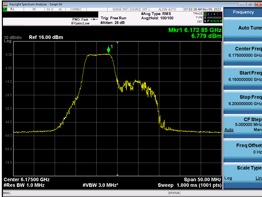
Plot 7-196. Power Spectral Density Plot MIMO ANT2 (20MHz BW 802.11ax/be (MRU) (UNII Band 5) – Ch. 45) – SP – 52+26T
