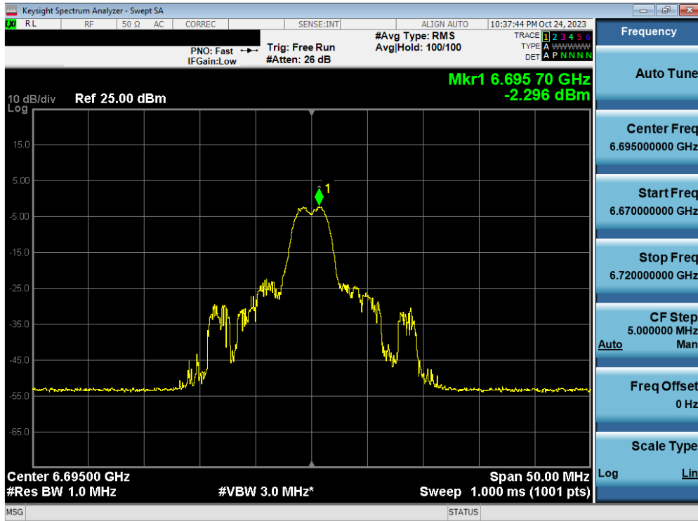
Plot 7-116. Power Spectral Density Plot MIMO ANT1 (20MHz BW 802.11ax/be (26 Tones) (UNII Band 7) – Ch. 149) – LPI
