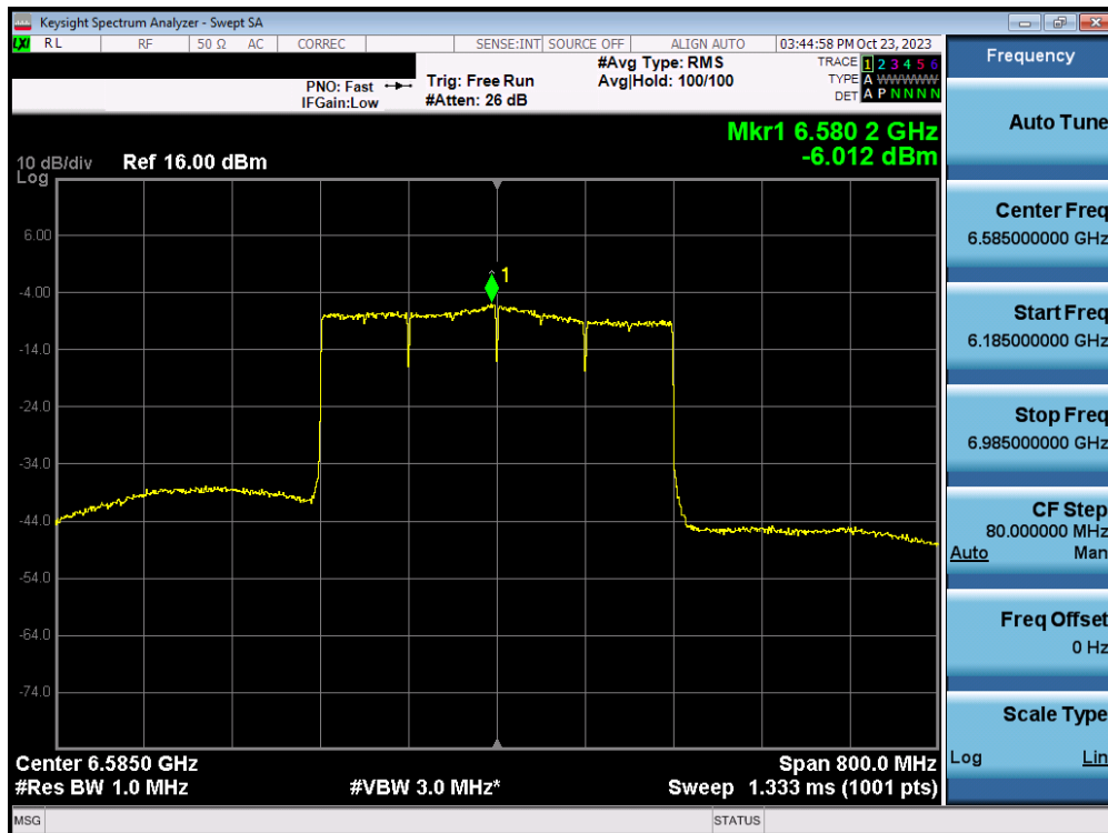
Plot 7-99. Power Spectral Density MIMO ANT2 (320MHz 802.11be (UNII Band 6/7) – Ch. 127) - LPI
