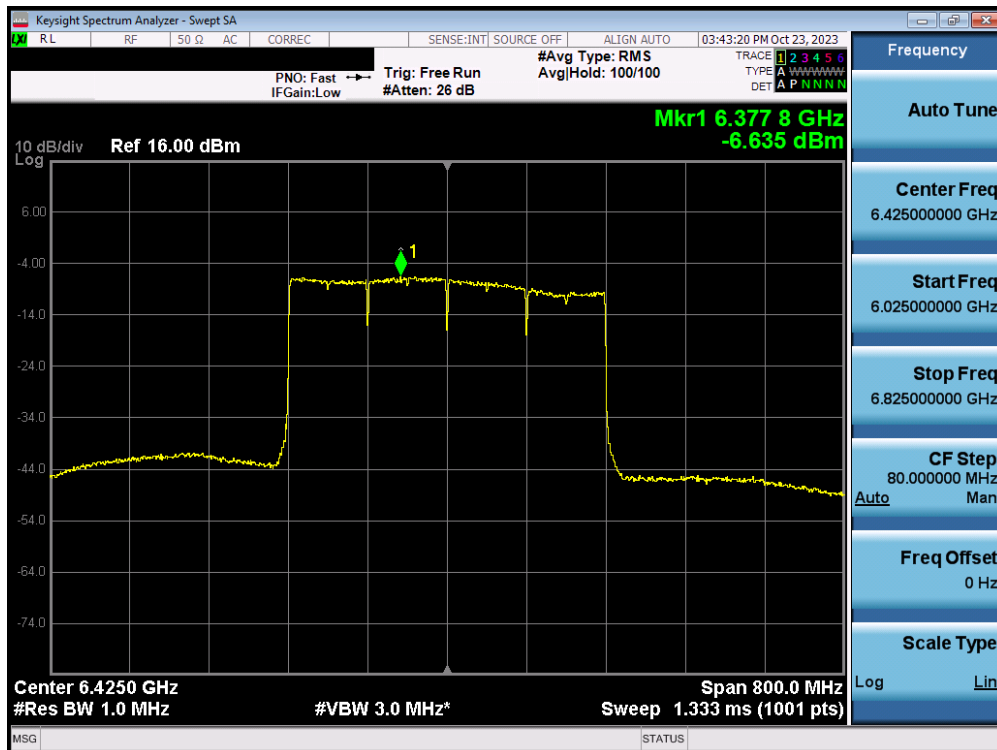
Plot 7-93. Power Spectral Density MIMO ANT2 (320MHz 802.11be (UNII Band 5/6/7) – Ch. 95) - LPI
