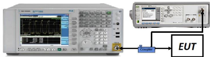
Figure 7-1. Test Instrument & Measurement Setup
