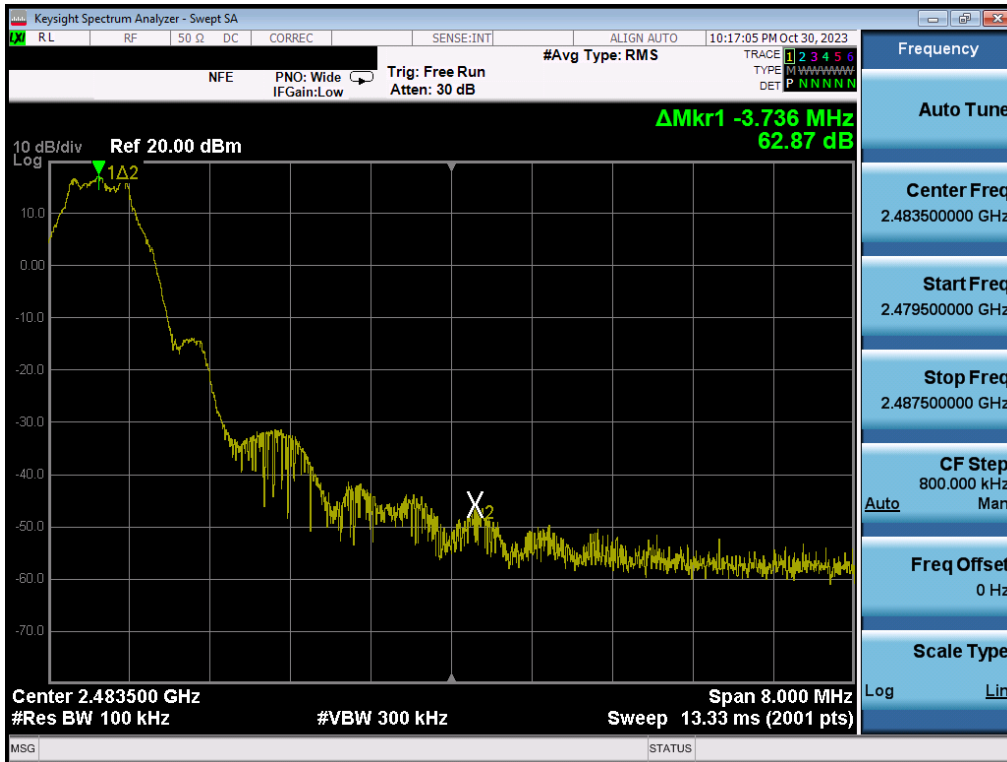
Plot 7-112. Band Edge Plot (Bluetooth (LE), 1Mbps – Ch. 39) – SISO ANT2
