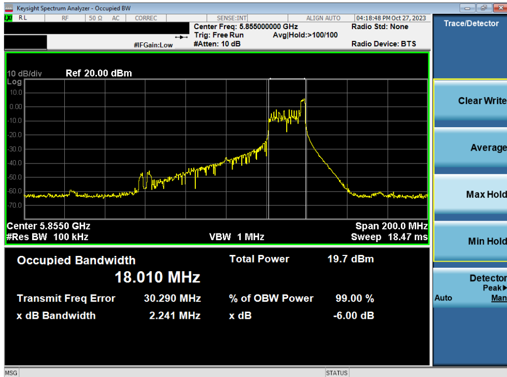
Plot 7-50. 6dB Bandwidth Plot MIMO ANT1 (80MHz BW 802.11be – 26 Tones (UNII Band 3/4) – Ch. 171)
