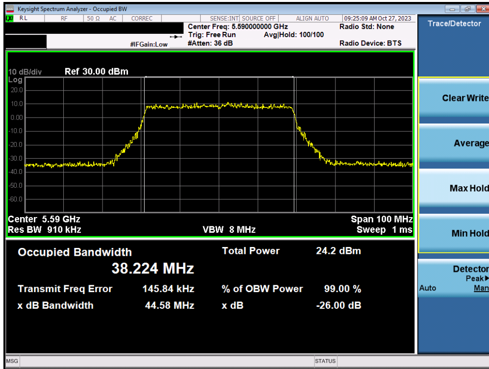
Plot 7-46. 26dB Bandwidth Plot MIMO ANT2 (40MHz BW 802.11ax/be (UNII Band 2C) – Ch. 118)
