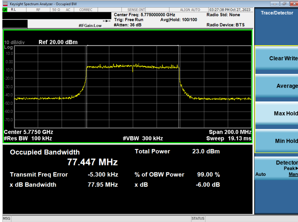
Plot 7-57. 6dB Bandwidth Plot MIMO ANT1 (80MHz BW 802.11ax/be (UNII Band 3) – Ch. 155)
