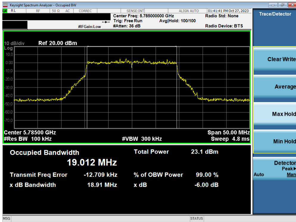
Plot 7-53. 6dB Bandwidth Plot MIMO ANT1 (20MHz BW 802.11ax/be (UNII Band 3) – Ch. 157)
