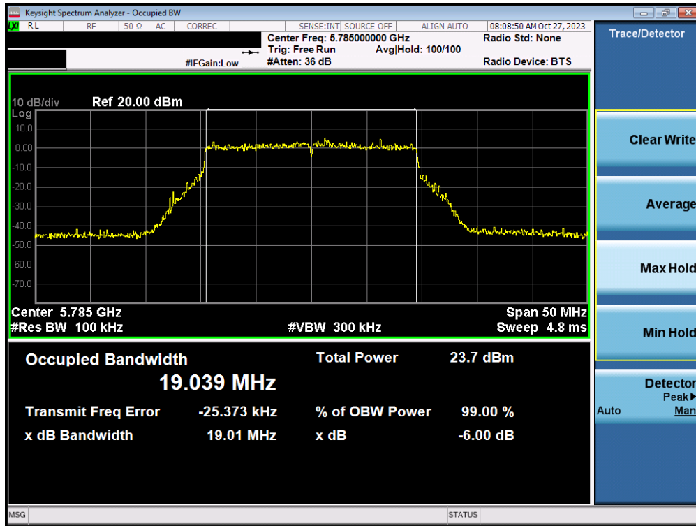
Plot 7-69. 6dB Bandwidth Plot MIMO ANT2 (20MHz BW 802.11ax/be (UNII Band 3) – Ch. 157)
