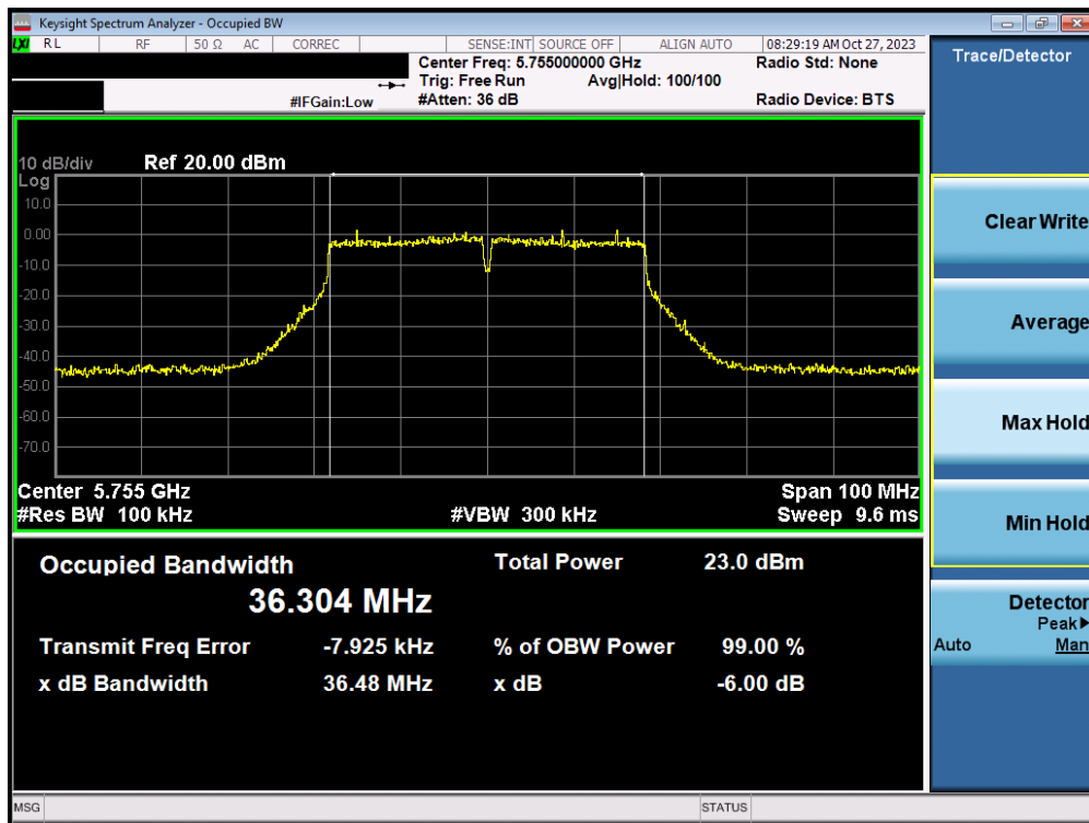
Plot 7-70. 6dB Bandwidth Plot MIMO ANT2 (40MHz BW 802.11n (UNII Band 3) – Ch. 151)
