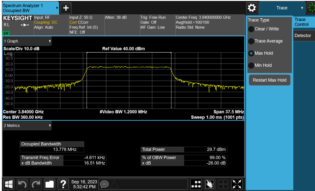
Plot 7-31. Occupied Bandwidth Plot (NR Band n77PC3 - 15MHz QPSK - Full RB - Ant1)
