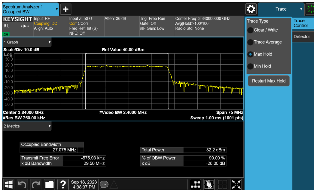
Plot 7-24. Occupied Bandwidth Plot (NR Band n77PC3 - 30MHz \pi/2 BPSK - Full RB - Ant1)
