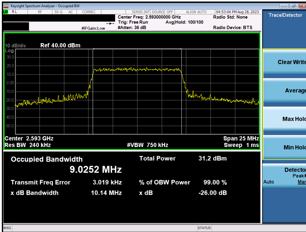
Plot 7-8. Occupied Bandwidth Plot (LTE Band 41(PC2) - 10MHz 16-QAM - Full RB - Ant1)
