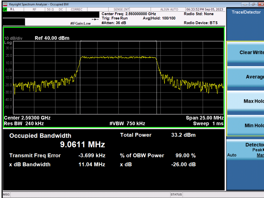
Plot 7-15. Occupied Bandwidth Plot (LTE Band 41(PC2) - 10MHz QPSK - Full RB - Ant2)
