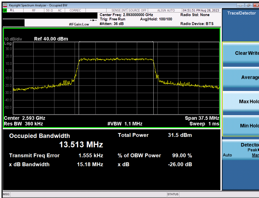
Plot 7-6. Occupied Bandwidth Plot (LTE Band 41(PC2) - 15MHz 16-QAM - Full RB - Ant1)
