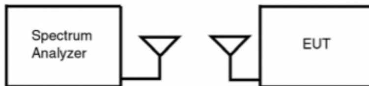
Figure 7-1. Test Instrument and Measurement Setup
