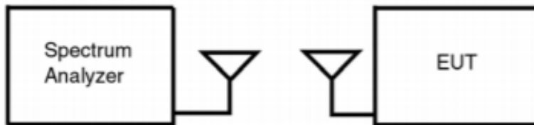
Figure 7-2. Test Instrument and Measurement Setup
