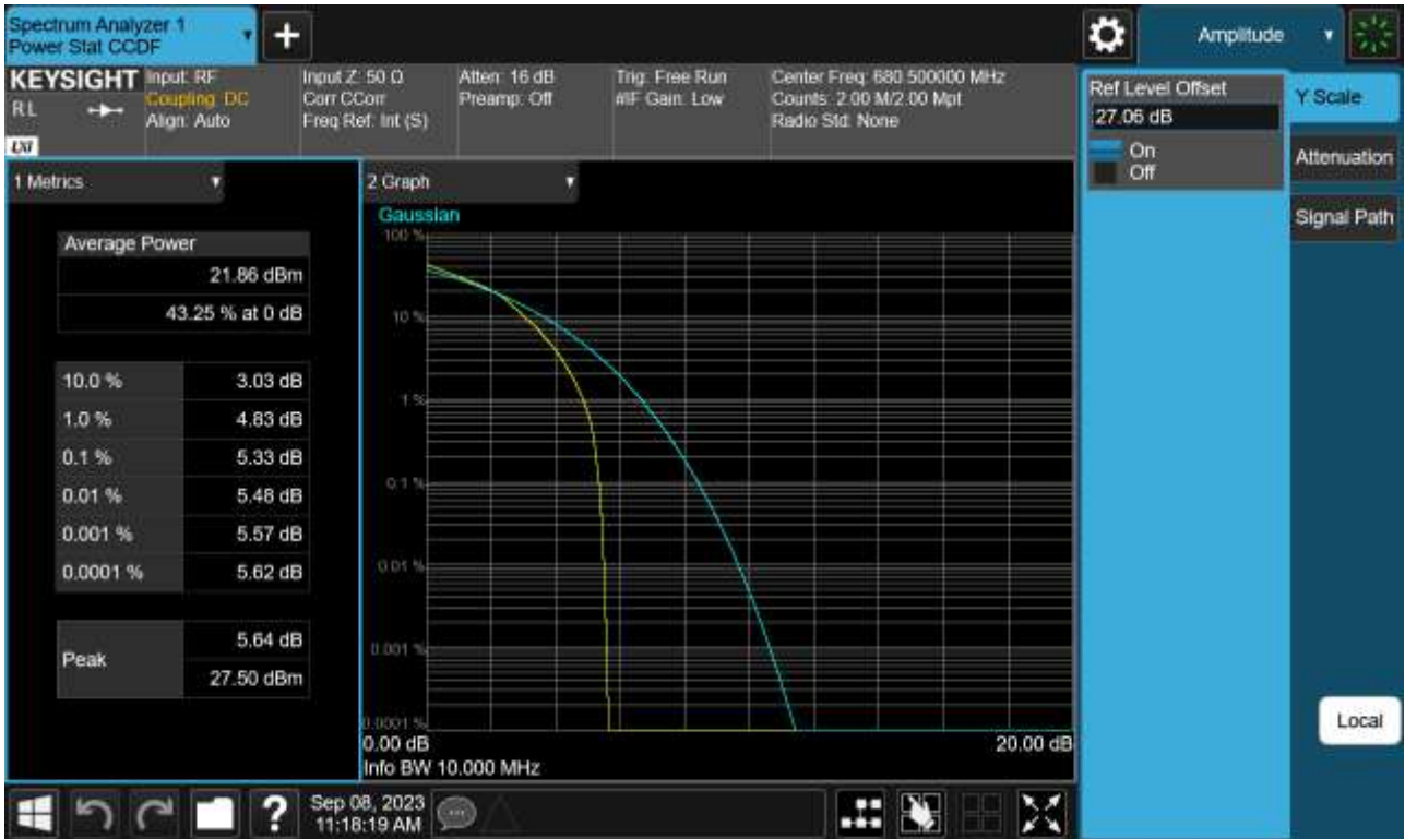
Sub6 n71. PAR Plot (10 M BW_Ch.349000_16QAM_Full RB)
