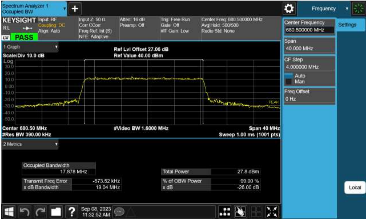
Sub6 n71. Occupied Bandwidth Plot (20 M BW Ch.136100 256QAM_ Full RB)
