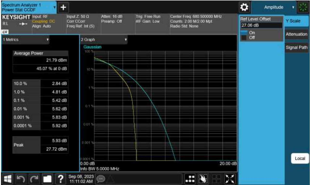
Sub6 n71. PAR Plot (5 M BW_Ch.349000_16QAM_Full RB)
