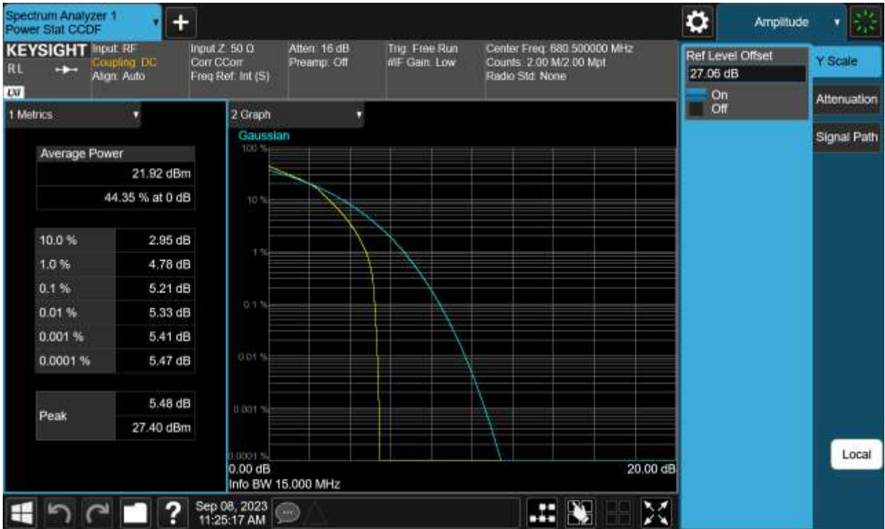
Sub6 n71. PAR Plot (15 M BW_Ch.349000_16QAM_Full RB)
