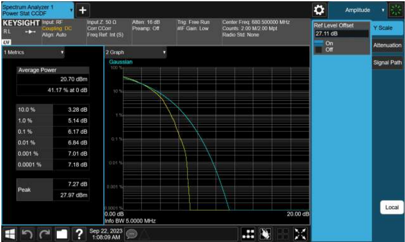
Sub6 n71. PAR Plot (5 M BW_Ch.349000_256QAM_Full RB)
