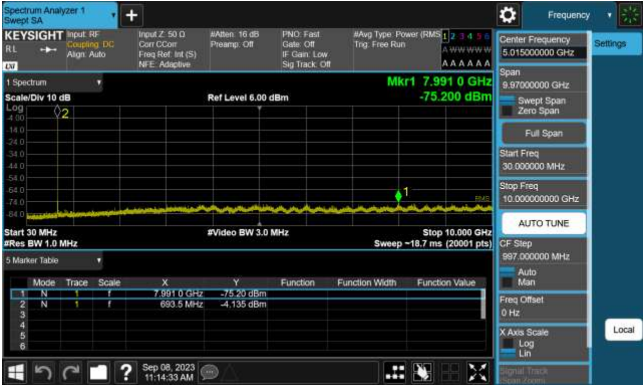
Sub6 n71. Conducted Spurious Plot _ (139100ch_5 MHz_BPSK_RB 1_1)
