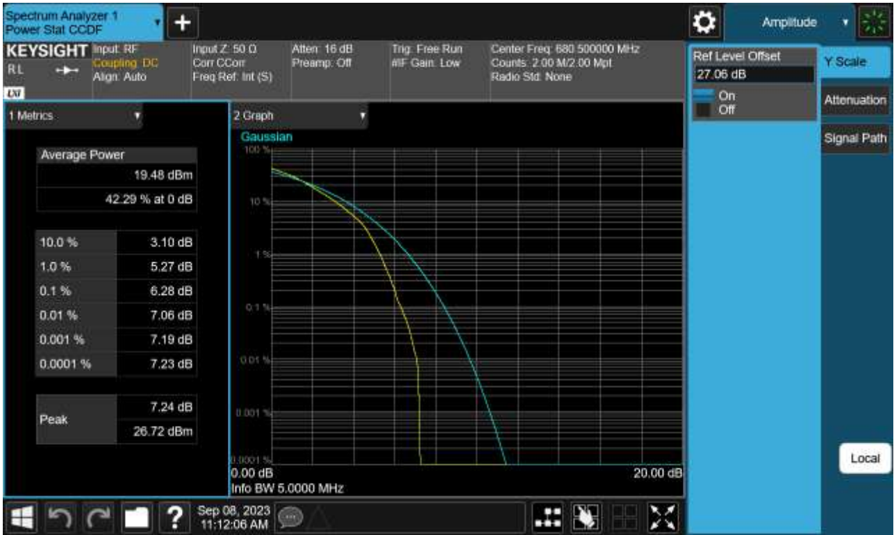
Sub6 n71. PAR Plot (5 M BW_Ch.349000_256QAM_Full RB)
