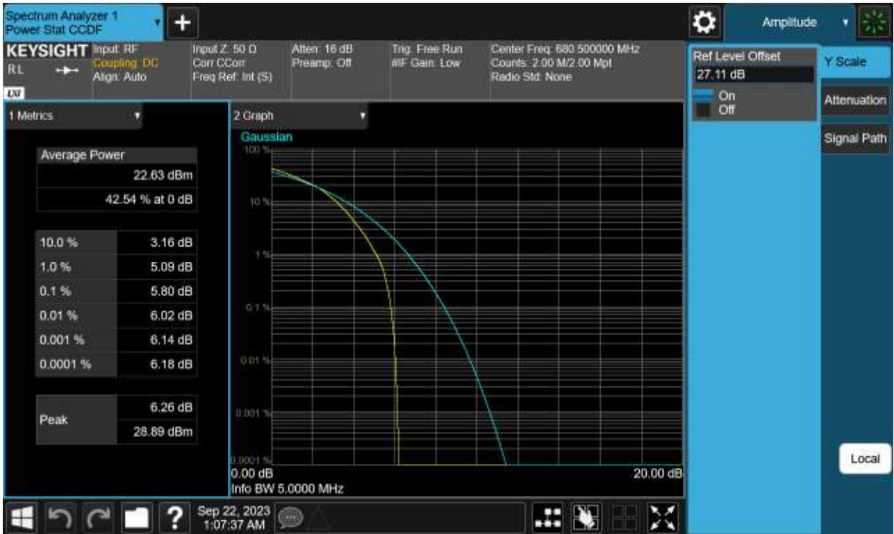
Sub6 n71. PAR Plot (5 M BW_Ch.349000_64QAM_Full RB)
