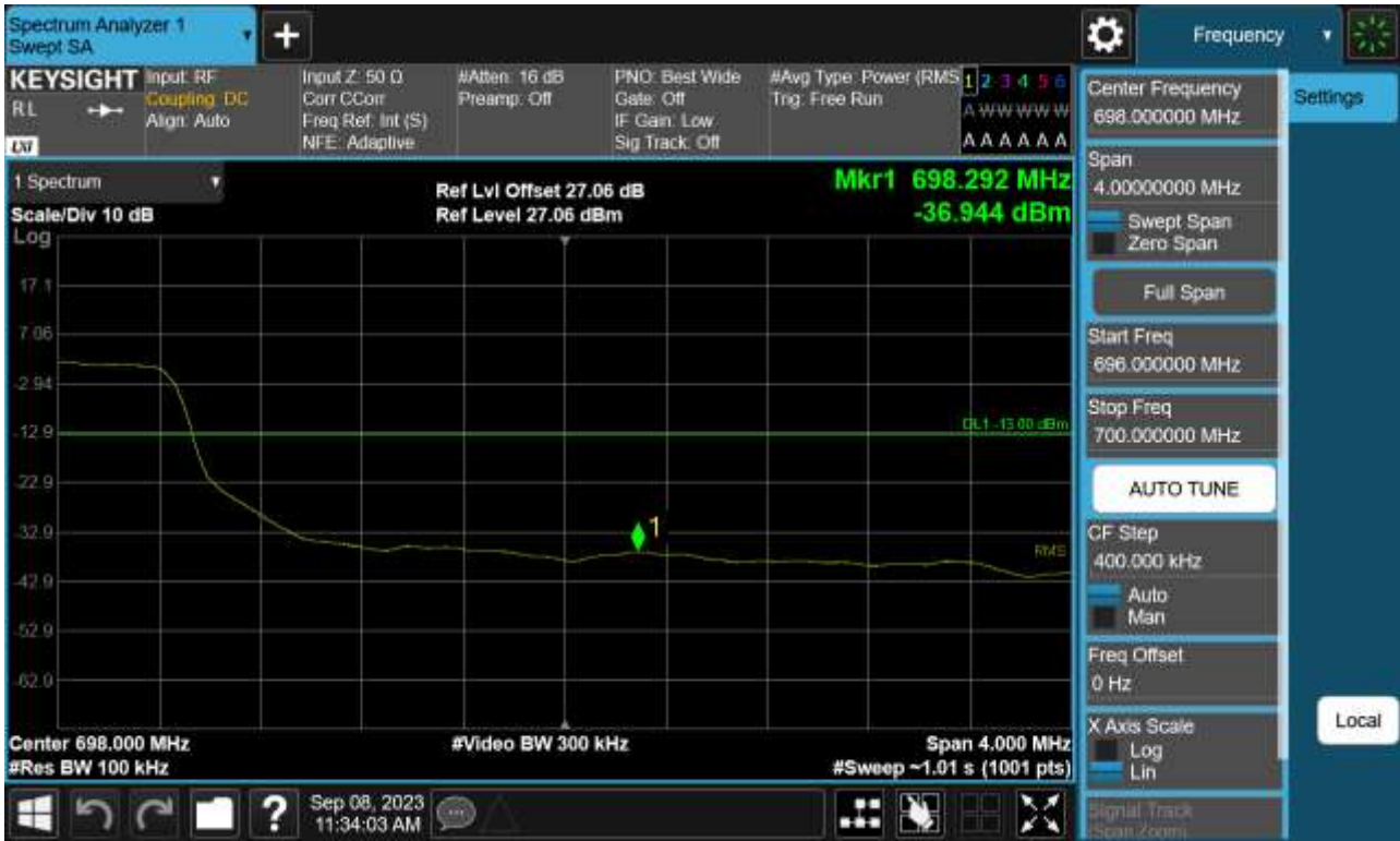
Sub6 n71. Upper Band Edge Plot (20 M BW Ch.137600 BPSK_ Full RB)
