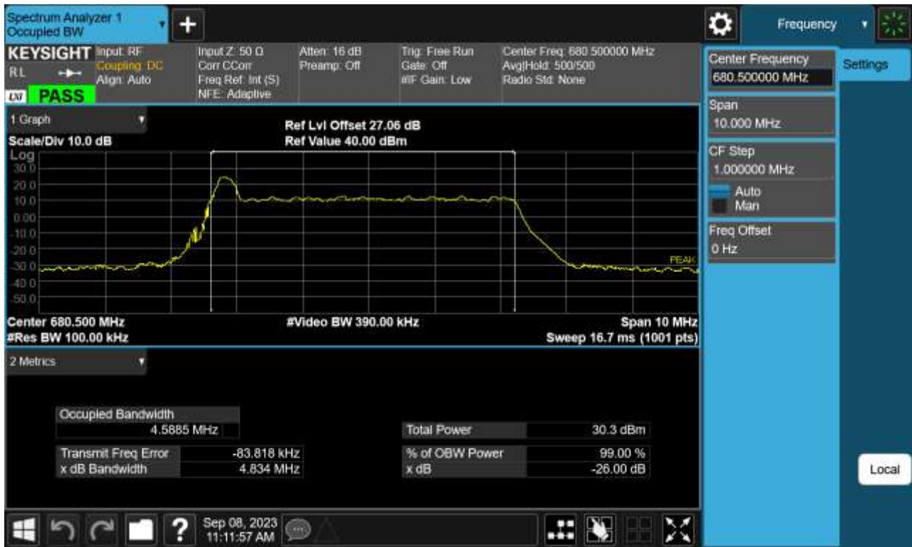
Sub6 n71. Occupied Bandwidth Plot (5 M BW Ch.136100 256QAM_ Full RB)
