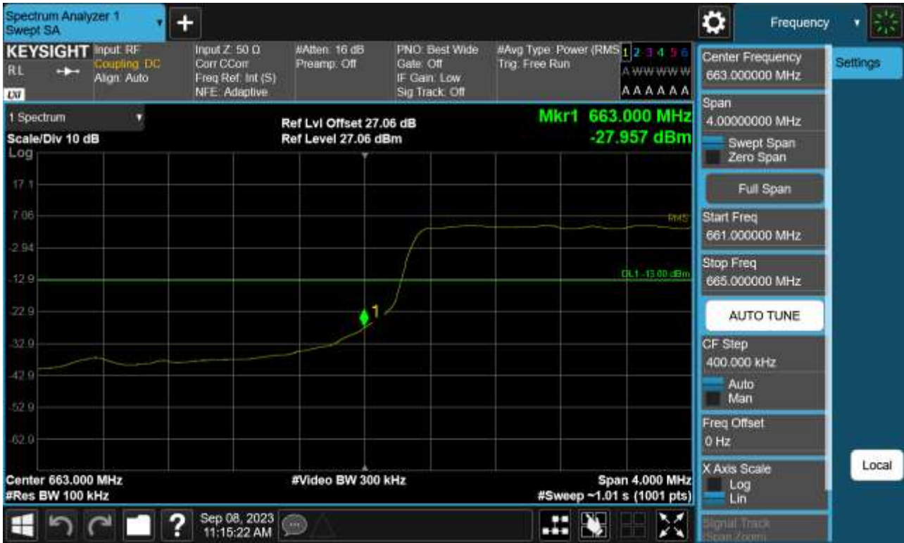
Sub6 n71. Lower Band Edge Plot (10 M BW Ch.133600 BPSK_ Full RB)
