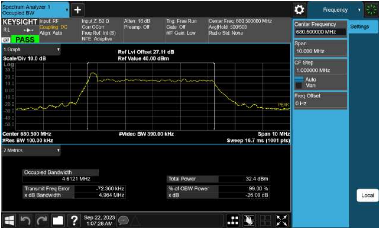
Sub6 n71. Occupied Bandwidth Plot (5 M BW Ch.136100 64QAM_ Full RB)
