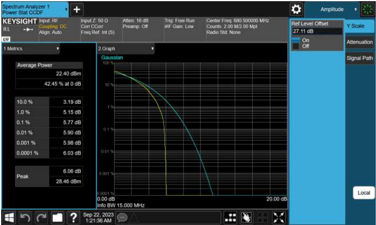
Sub6 n71. PAR Plot (15 M BW_Ch.349000_64QAM_Full RB)
