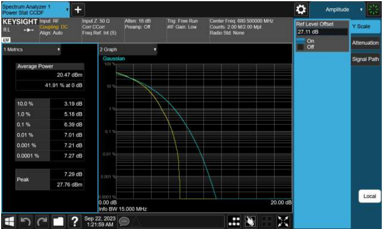
Sub6 n71. PAR Plot (15 M BW_Ch.349000_256QAM_Full RB)
