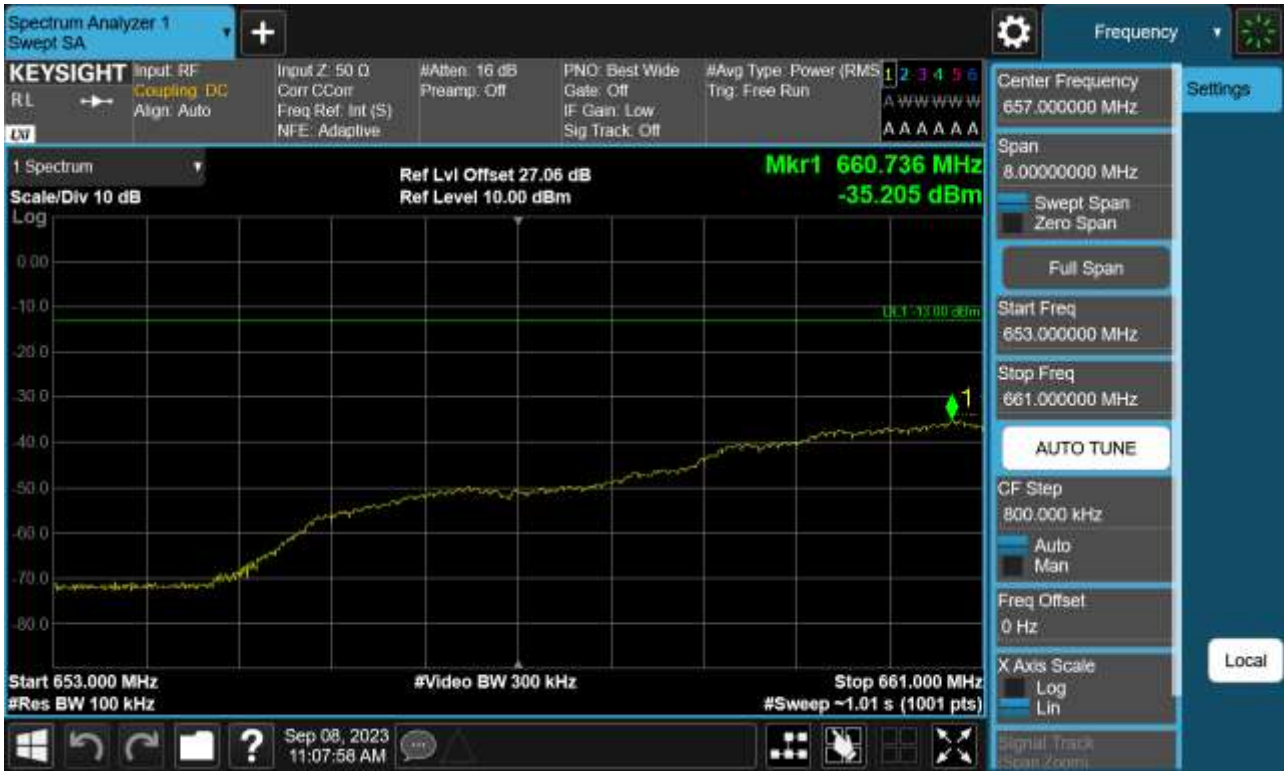
Sub6 n71. Lower Extended Band Edge Plot (5 M BW Ch.133100 BPSK_ Full RB)
