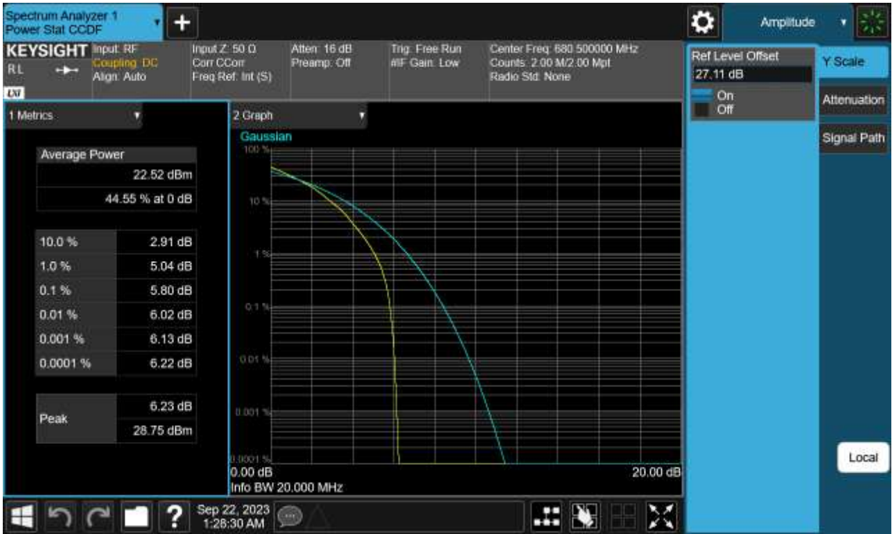
Sub6 n71. PAR Plot (20 M BW_Ch.349000_64QAM_Full RB)
