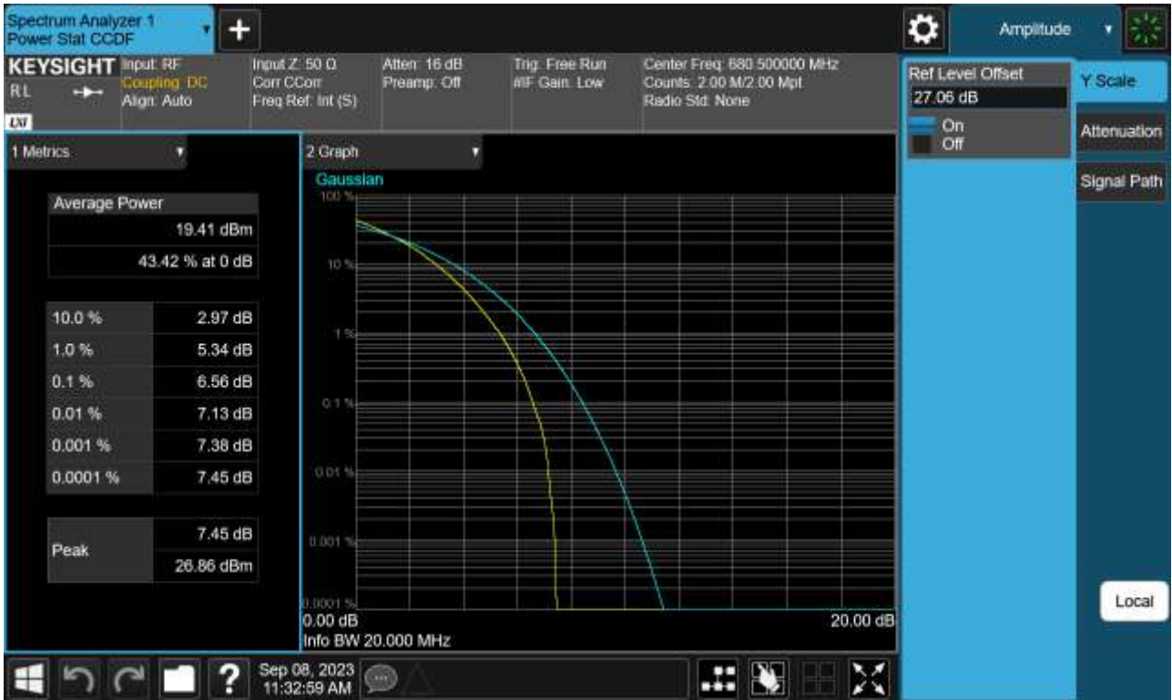
Sub6 n71. PAR Plot (20 M BW_Ch.349000_256QAM_Full RB)
