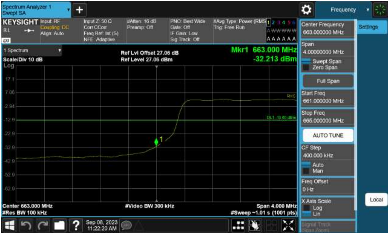
Sub6 n71. Lower Band Edge Plot (15 M BW Ch.134100 BPSK_ Full RB)
