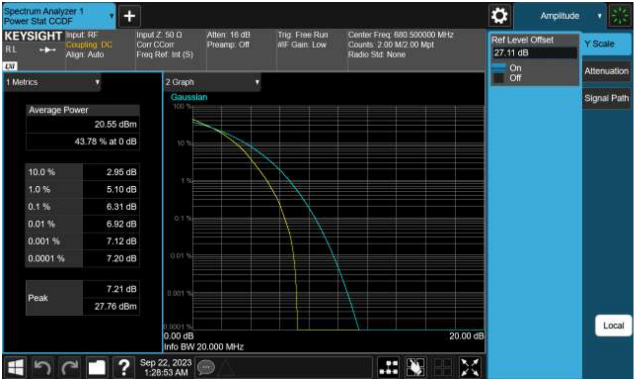
Sub6 n71. PAR Plot (20 M BW_Ch.349000_256QAM_Full RB)
