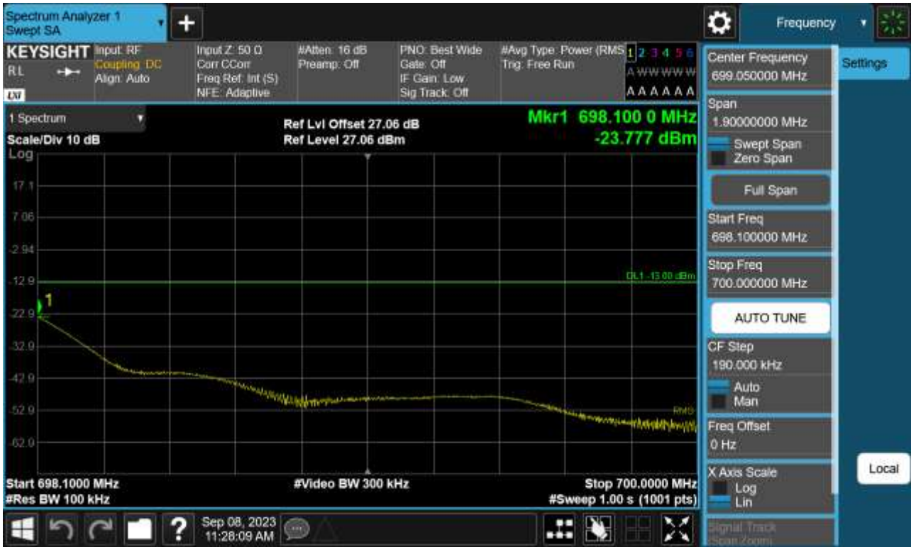
Sub6 n71. Upper Band Edge Plot (15 M BW Ch.138100 BPSK_RB1_Offset 78)_2
