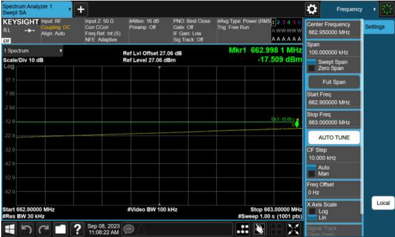
Sub6 n71. Lower Band Edge Plot (5 M BW Ch.133100 BPSK_RB1_Offset 0)_1
