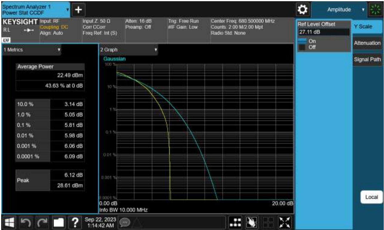
Sub6 n71. PAR Plot (10 M BW_Ch.349000_64QAM_Full RB)
