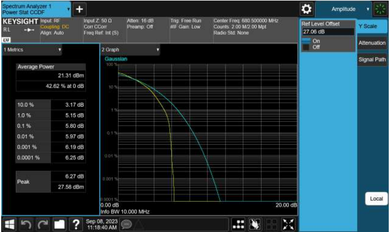
Sub6 n71. PAR Plot (10 M BW_Ch.349000_64QAM_Full RB)
