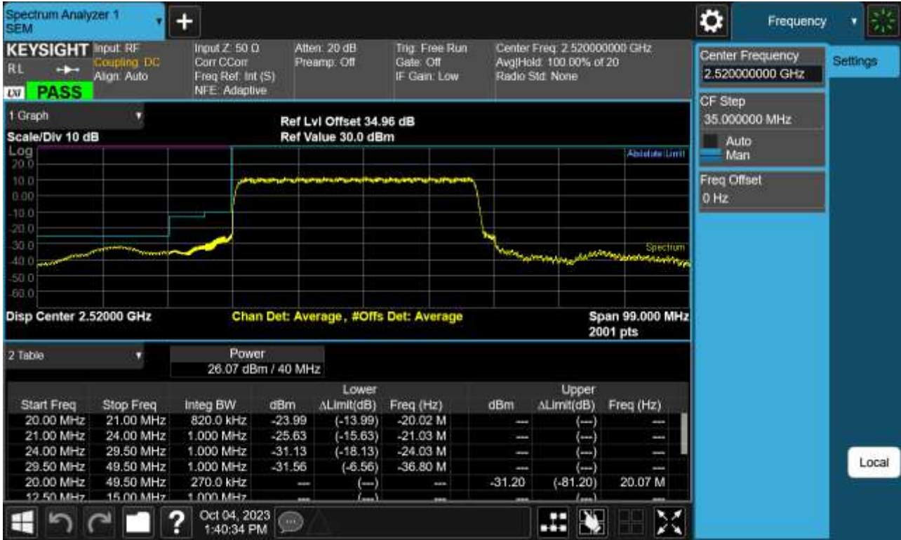
Sub6 n41. Low Channel Edge Plot (40 MHz Ch.504000 BPSK)-3
