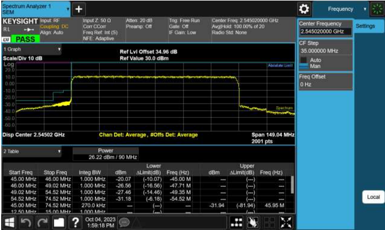
Sub6 n41. Low Channel Edge Plot (90 MHz Ch.509004 BPSK)-3
