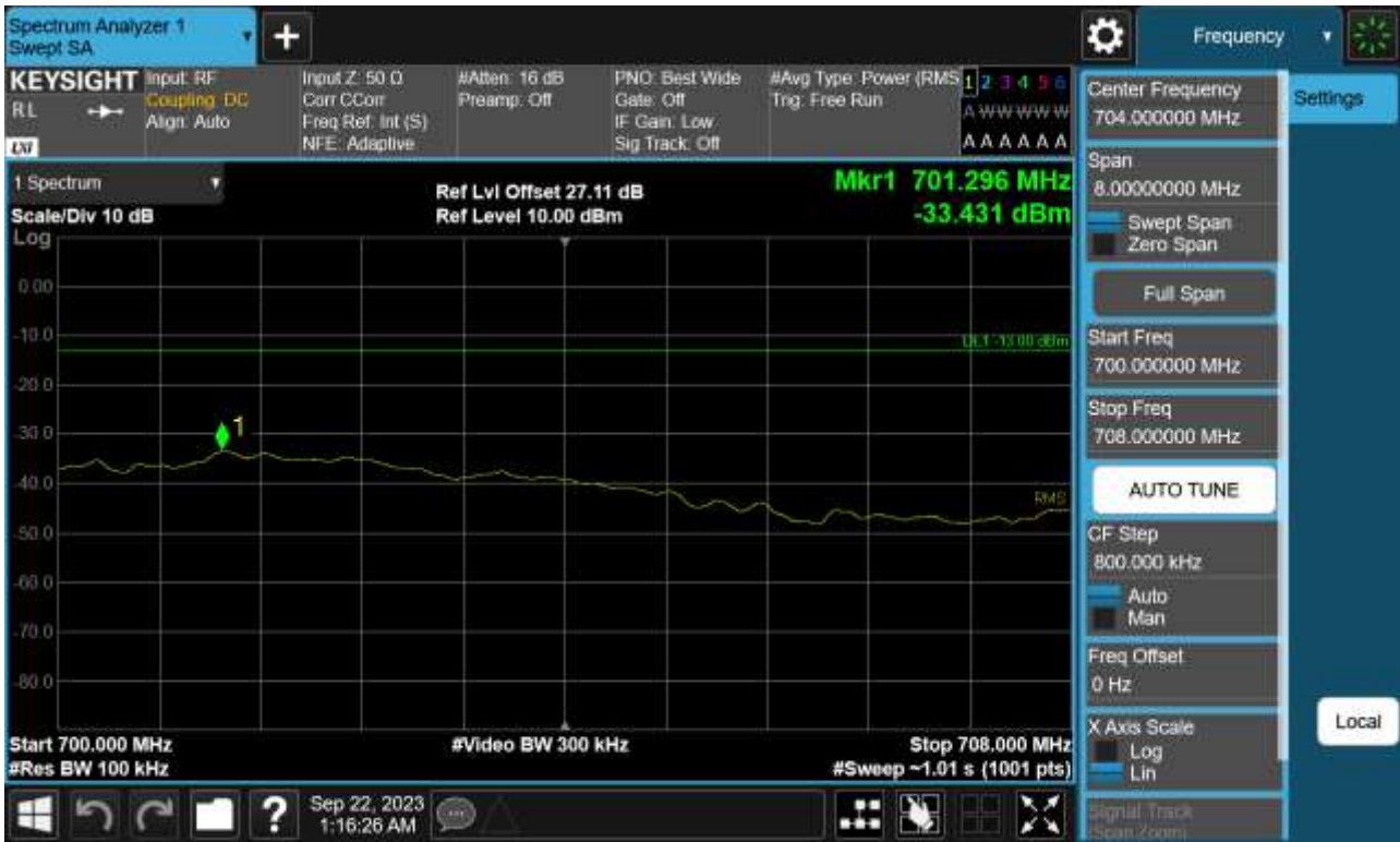
Sub6 n71. Upper Extended Band Edge Plot (10 M BW Ch.138600 BPSK_ Full RB)
