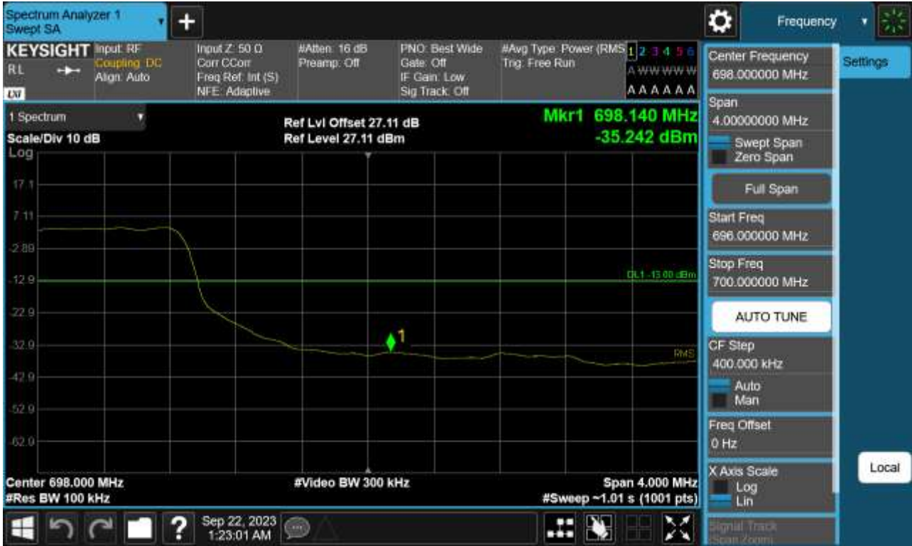
Sub6 n71. Upper Band Edge Plot (15 M BW Ch.138100 BPSK_ Full RB)
