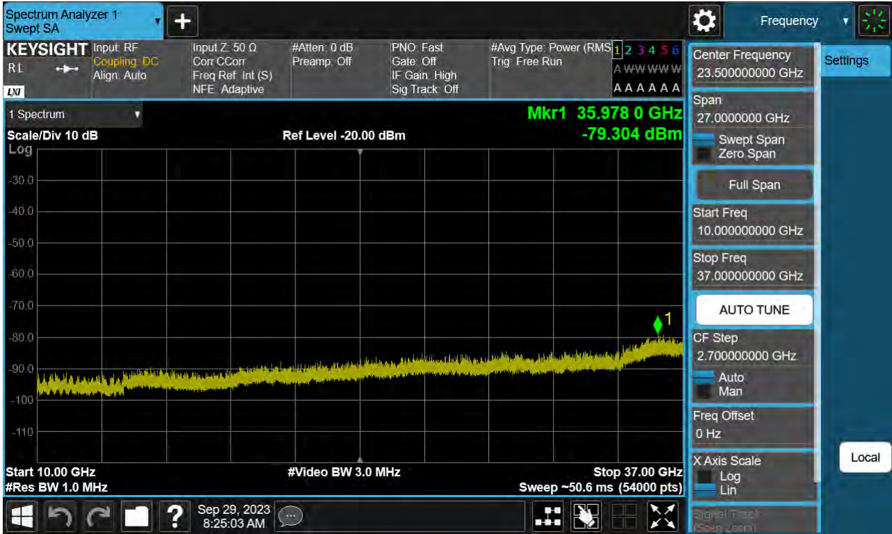
Sub6 n48. Conducted Spurious Plot 2 (15 MHz Ch. 637168 BPSK RB 1, Offset 1)
