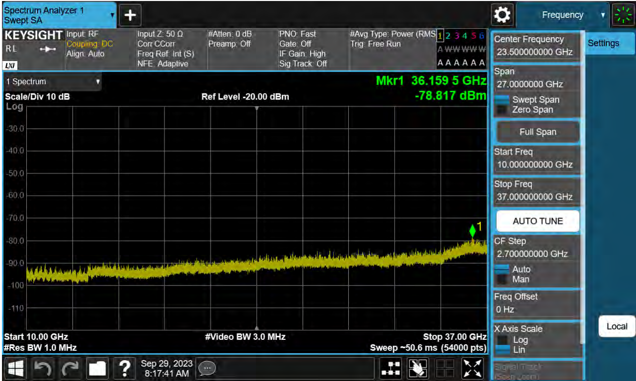
Sub6 n48. Conducted Spurious Plot 2 (10 MHz Ch. 646332 BPSK RB 1, Offset 1)
