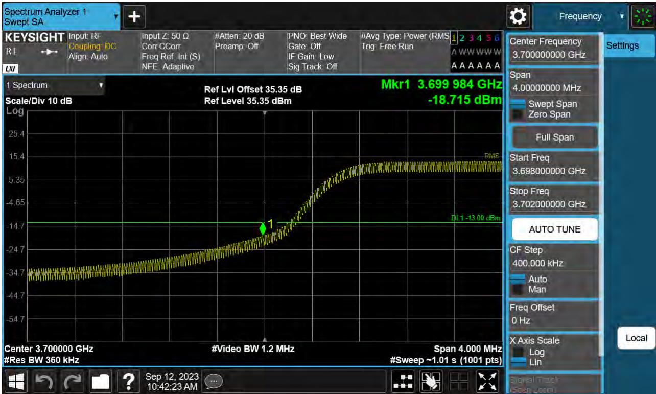
Sub6 n77(78). Low Band Edge Plot (10 M BW Ch.647000 BPSK FullRB)(1)
