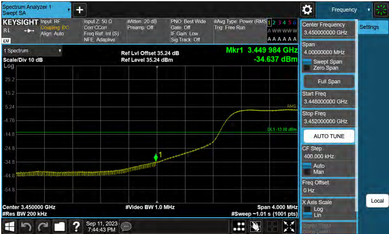
Sub6 n77(78). Low Band Edge Plot (50 M BW Ch.631668 BPSK FullRB)(1)
