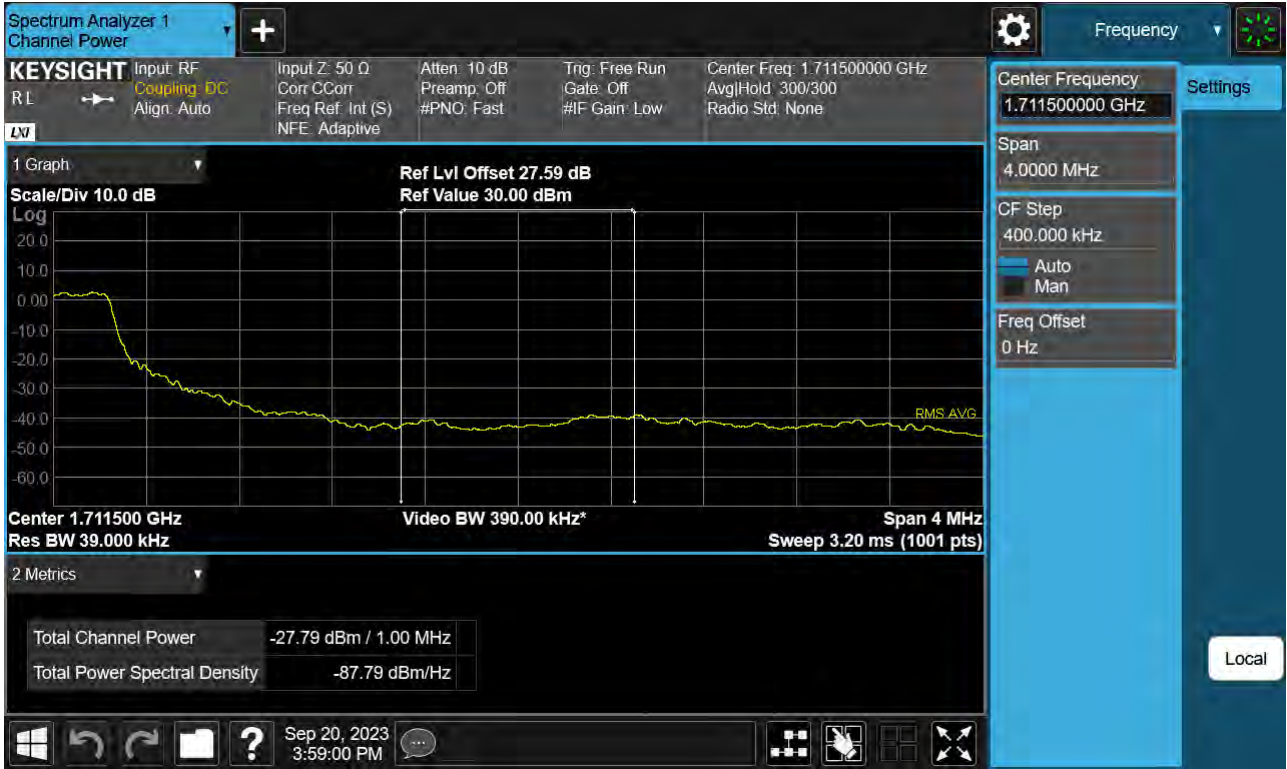
Sub6 n70. Upper Extended Band Edge Plot (5 M BW Ch.341500 BPSK_ Full RB) -3
