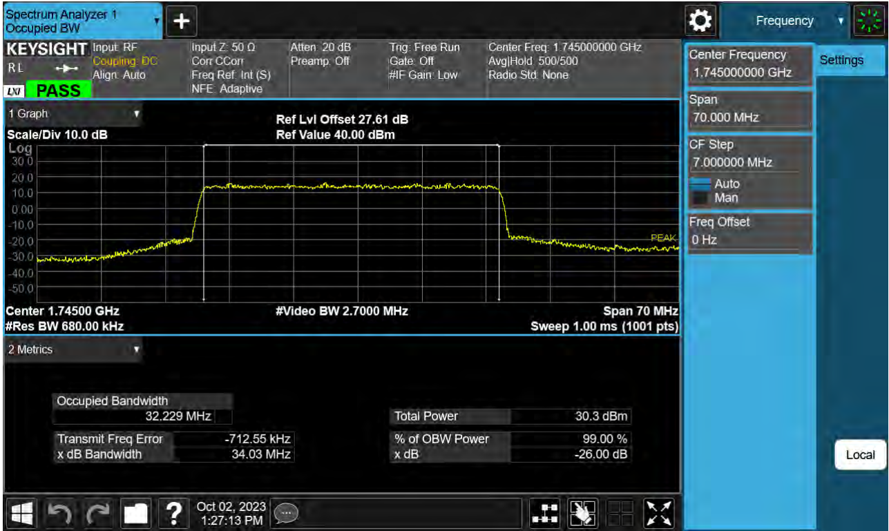
Sub6 n66. Occupied Bandwidth Plot (35 M BW Ch.349000 16QAM Full RB)
