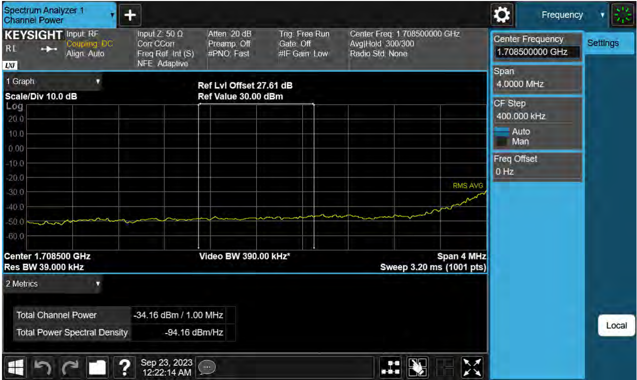
Sub6 n66. Lower Extended Band Edge Plot (30 M BW Ch.345000 BPSK_ Full RB) -3
