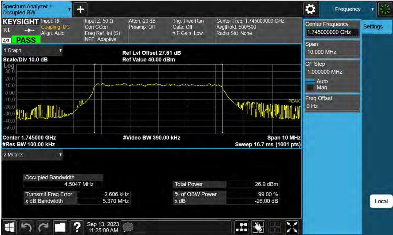
Sub6 n66. Occupied Bandwidth Plot (5 M BW Ch.349000 256QAM Full RB)
