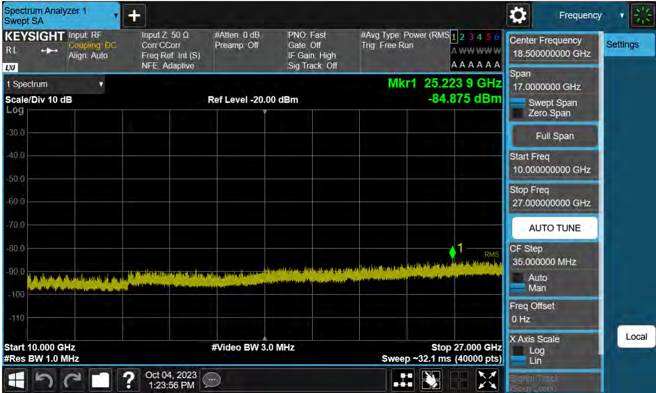
Sub6 n41. Conducted Spurious Plot 2 (15 MHz Ch.501504 BPSK RB 1)
