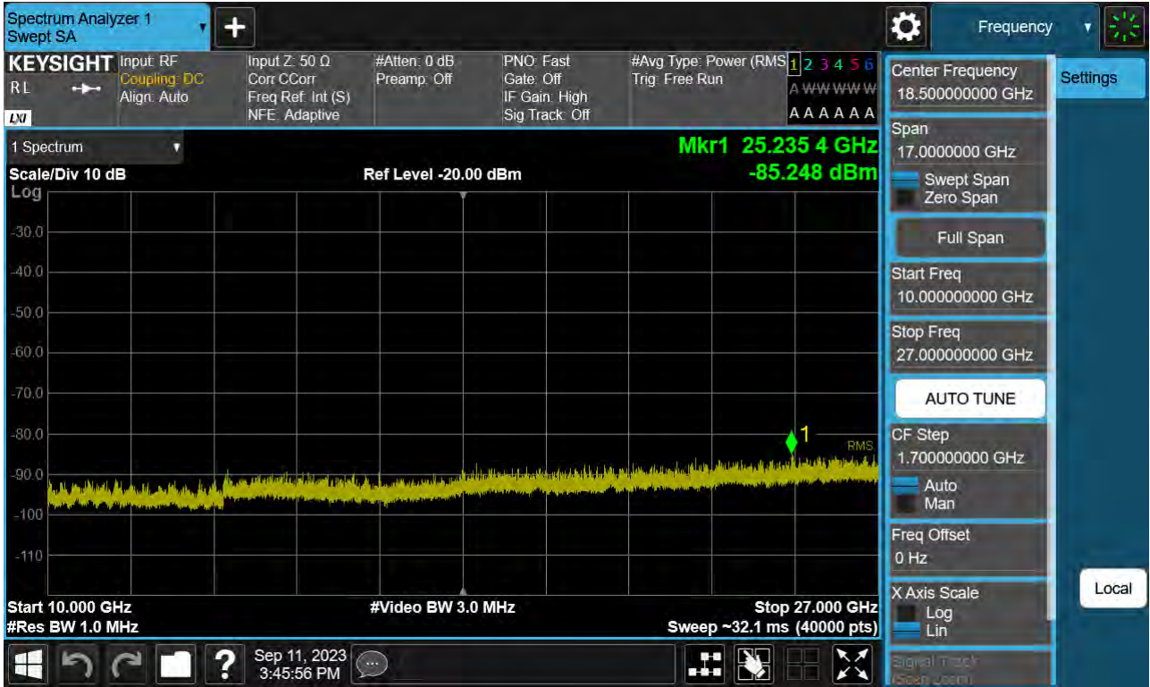
Sub6 n41. Conducted Spurious Plot 2 (40 MHz Ch.503202 BPSK RB 1)
