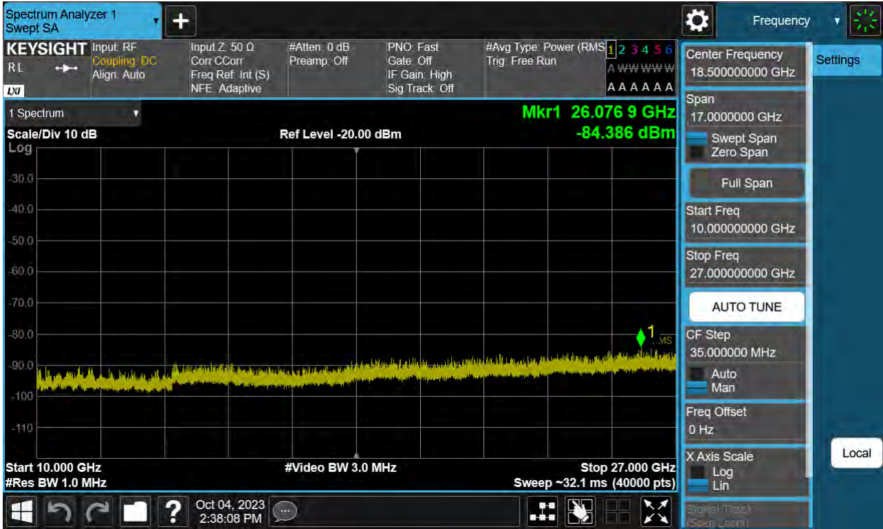
Sub6 n41. Conducted Spurious Plot 2 (40 MHz Ch.504000 BPSK RB 1)
