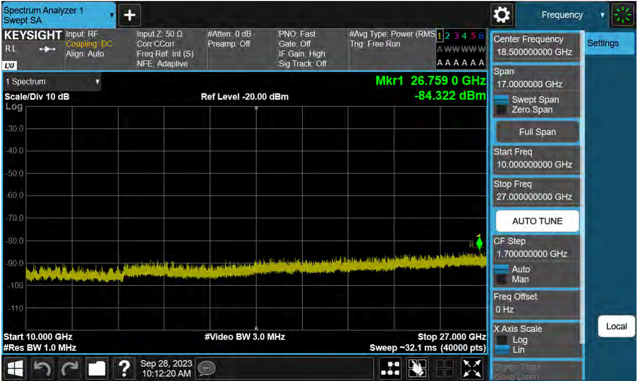
Sub6 n41. Conducted Spurious Plot 2 (40 MHz Ch.518598 BPSK RB 1)
