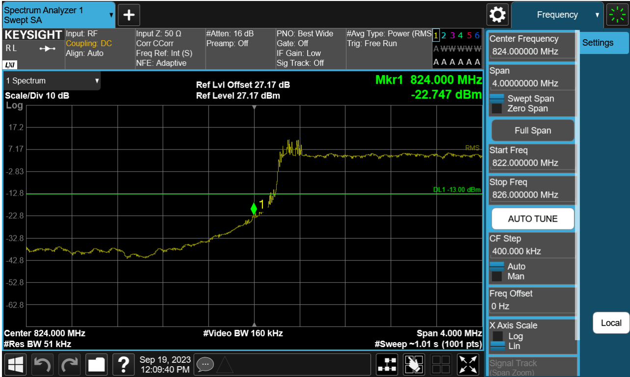
Sub6 n26. Lower Band Edge Plot (5 M BW Ch.165300 BPSK_RB 25_Offset 0)
